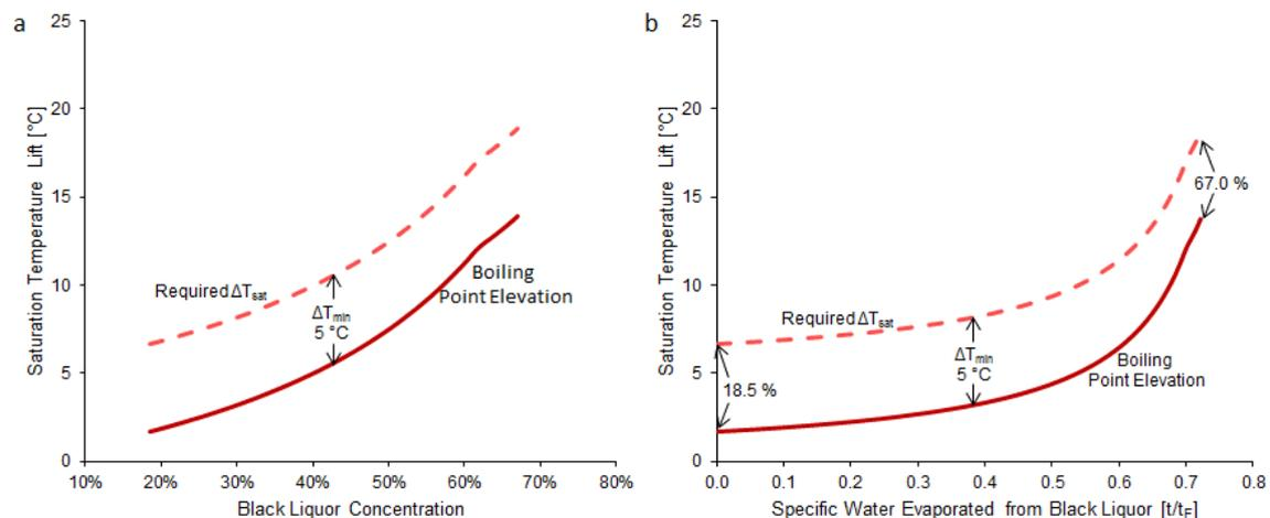
Figure 1: Boiling point elevation for black liquor (Zaman et al., 1998) for concentrating black liquor from 18.5 % to 67.0 %, based on concentration (a) and specific evaporation (b).
