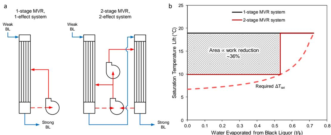
Figure 2: Simple 1- and 2-stage mechanical vapour recompression system designs (a) with the comparison to the required saturation temperature indicating the degree of work reduction (b).
