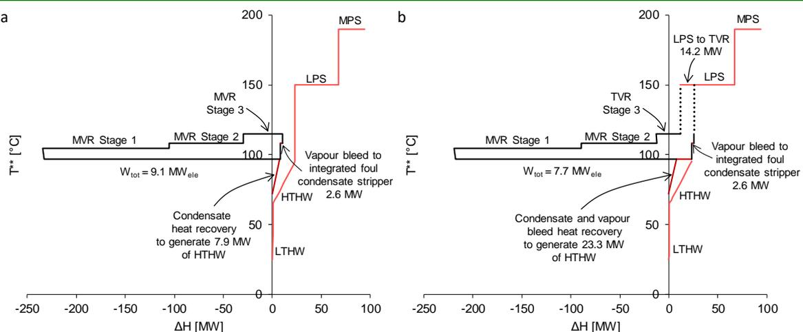
Figure 4: Total Site Heat Integration of 3-stage MVR evaporator (a) and 2-stage MVR, 1-stage TVR evaporator (b) with the site steam and hot water utility system using the Site Utility Grand Composite Curve.
