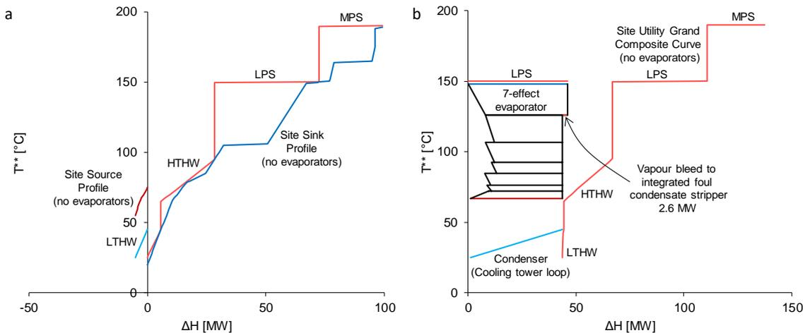
Figure 3: Total Site Profiles (a) and Site Utility Grand Composite Curve (b) with existing integration for a conventional 7-effect black liquor evaporator.
