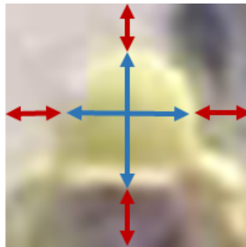
Figure 4.7: The cap is located at the centre of the box with margin of half a cap width around it.
