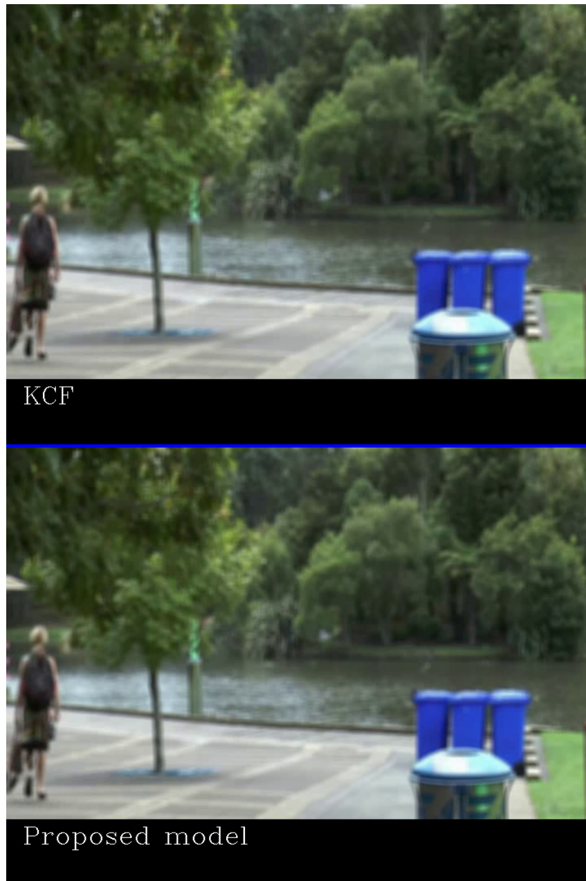
Figure 6.11: Visual tracking result for Waikato-1. The KCF lost objects after they walk behind the tree. This is because the KCF algorithm did not encode the background motion information therefore the tree is considered as a tracked object and the classifier is trained with the wrong features which leads to the tracking drift.
