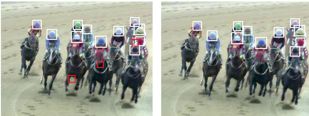
Figure 4.11: The left image shows the detection result before contextual filtering and the right image illustrated the final result after applying contextual filtering. It is shown the false positive (red boxes) are removed by contextual filtering.
