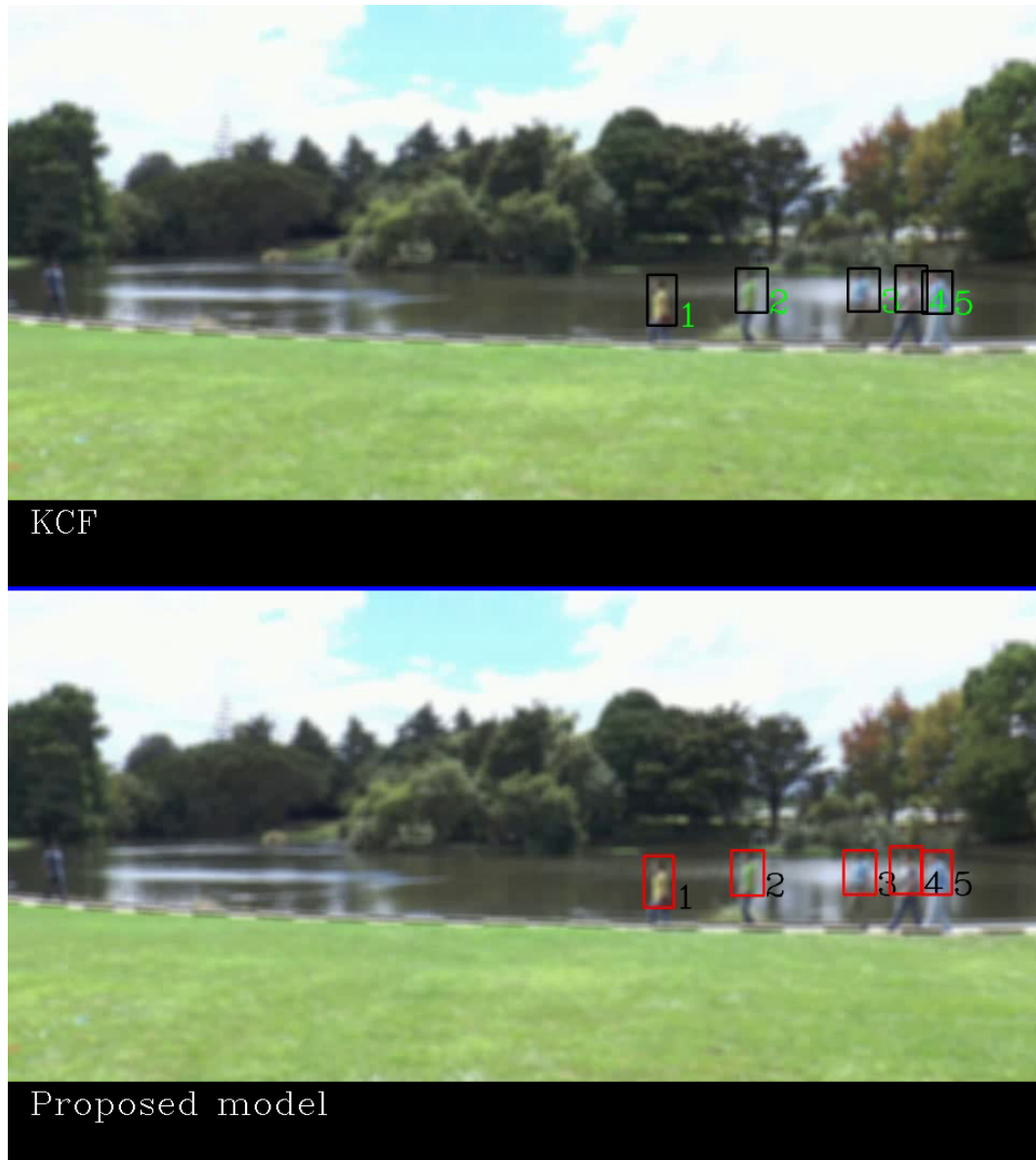
Figure 6.15: Visual tracking result for Waikato-3. The proposed model fails to track objects 3 as both its motion and appearance is similar to object 5.
