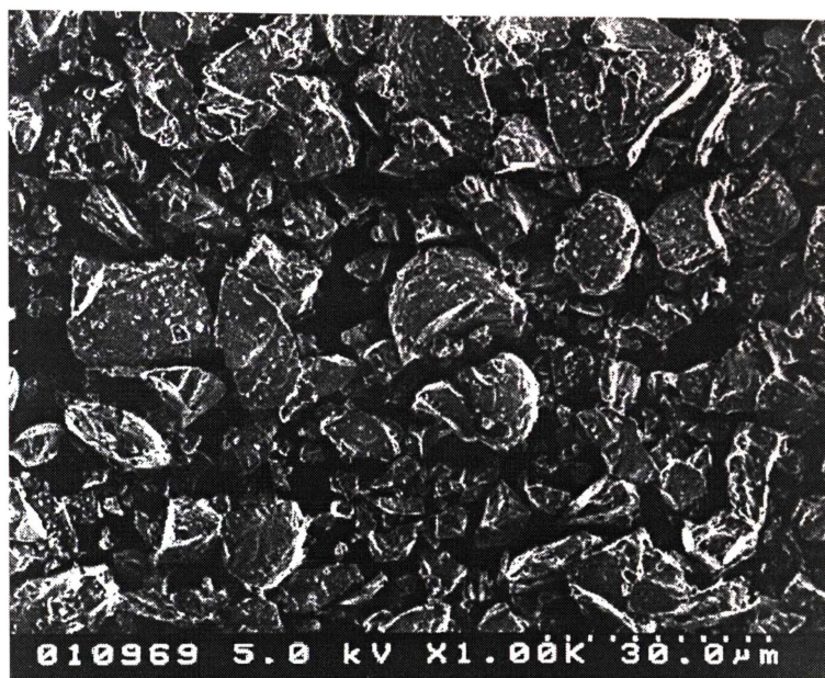
Figure 3.9 Micrograph of YSZ sintered at 1100 °C after 45 minutes of milling.
