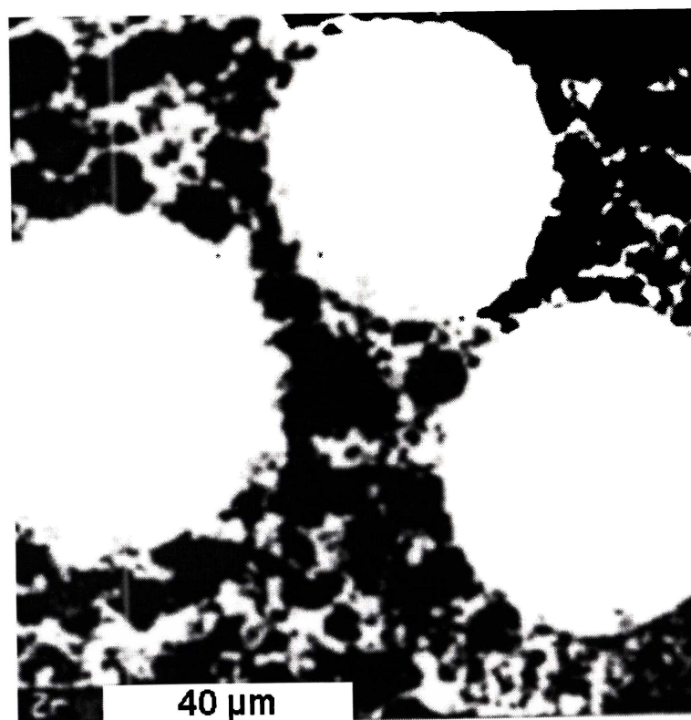
Figure 1.13 Secondary electron image (SEI) of a Ni/YSZ cermet showing the elemental distribution of the two sizes of white YSZ particles and dark NiO particles 44 .
