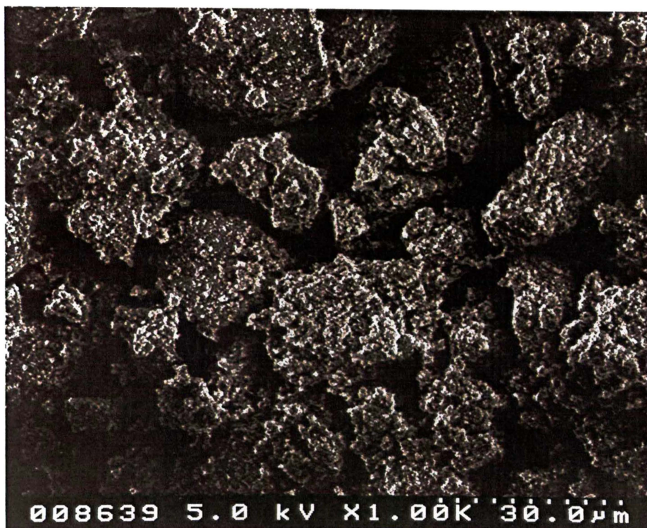
Figure A3.8 SEM micrograph of YSZ sintered at 1100 °C after ball milling for 6 hours.
