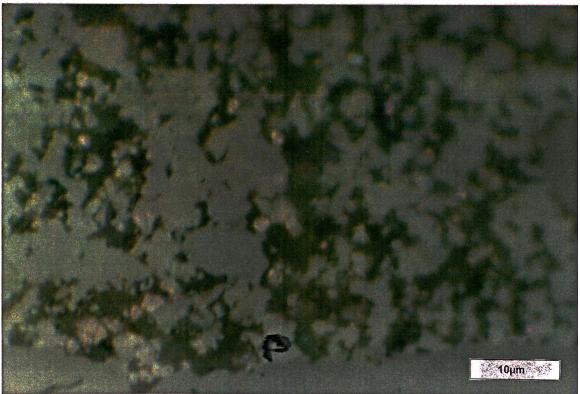
Figure A4.10 Anode #3 illustrating sintering of layer at a magnification of 1500x.
