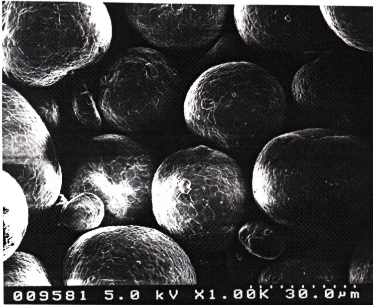
Figure 3.1(b) Micrograph of YSZ sintered at 1400 °C.
