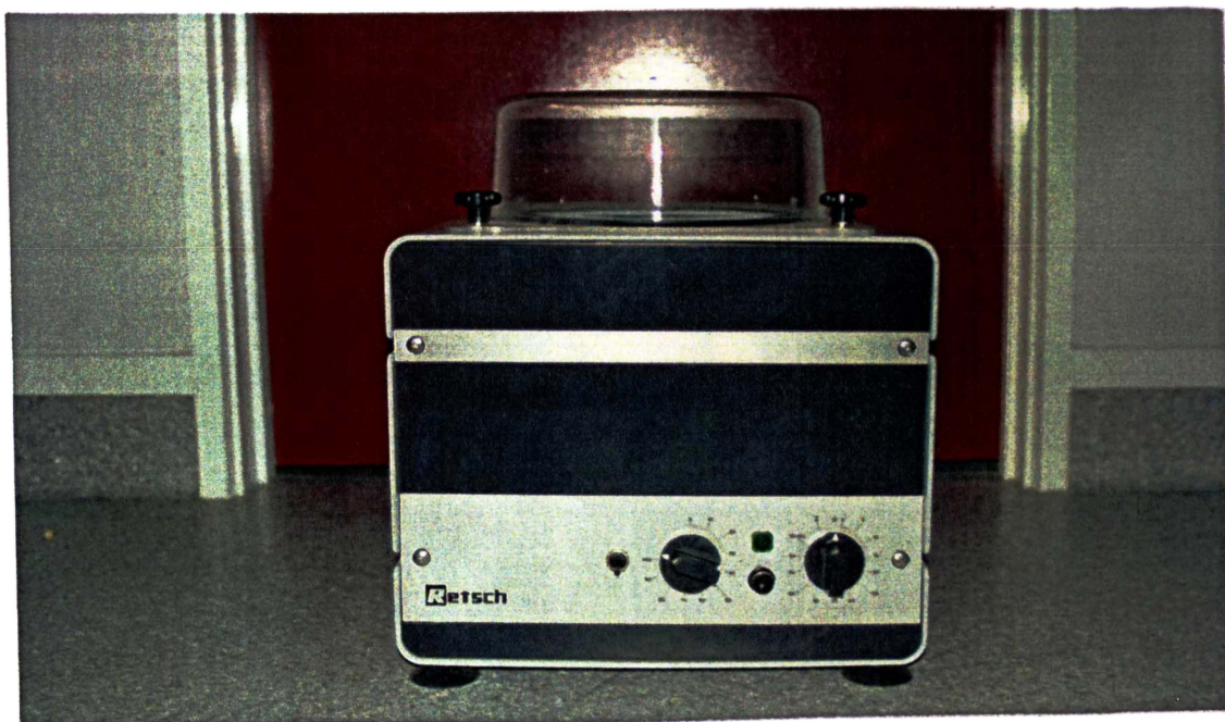
Figure 2.2 Centrifugal mill used for high energy milling of the highly sintered YSZ powders in order to control particle size.
