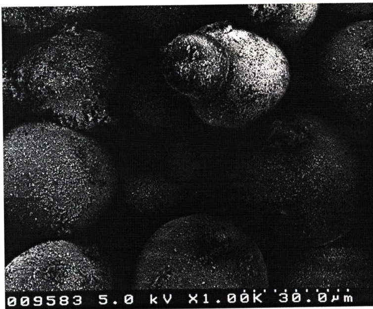
Figure 3.1(a) Micrograph of yttria stabilised zirconia (YSZ) sintered at 1100 °C
