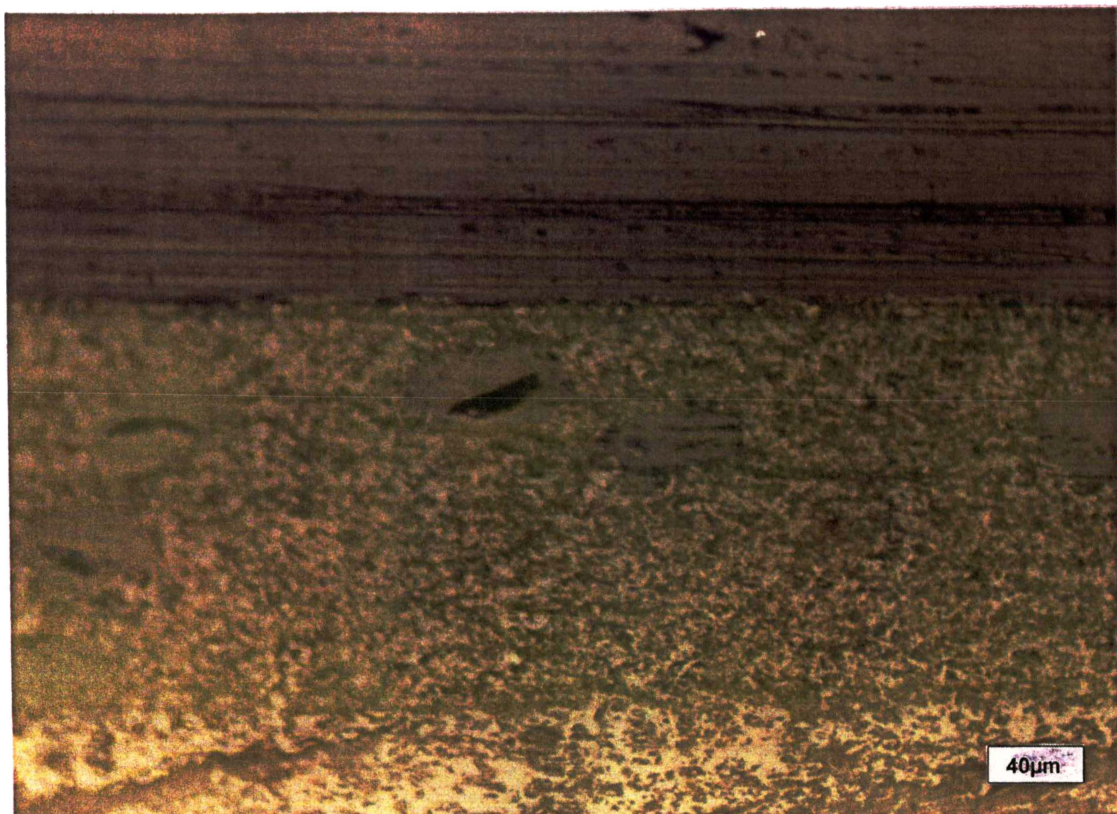
Figure A4.52 Anode #14 illustrating homogeneous NiO/YSZ distribution. Magnification of 200x.
