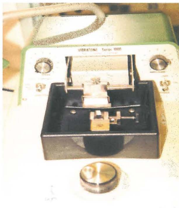
Figure 4.2.1 - Slicing of CIDR ® 1900 Cattle insert segments with the Vibratome ® Series 1000 sectioning system
