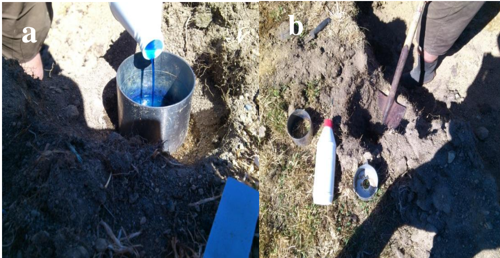
Figure 3.10: Assessment of pore continuity: (a) addition of methylene blue dye in metal rings, (b) cutting the soil back to see how far the dye had travelled through it.
