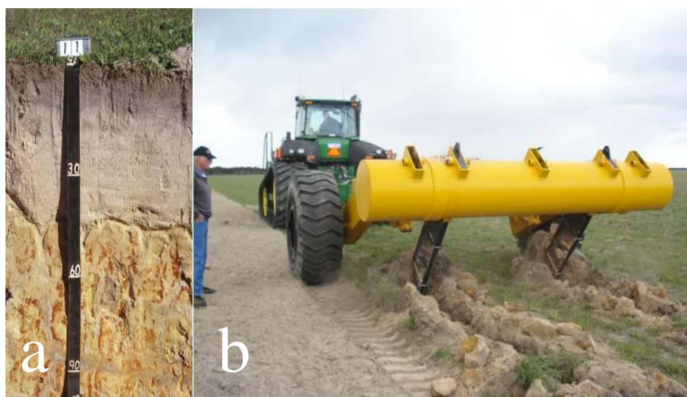
Figure 2.10: Soil mixing to improve physical properties in Australia. (a): example of a duplex soil. From http://grains.agric.wa.gov.au/node/deep-sandy-duplex . (b): Clay delving . From http://www.precisionag.com.au/page16.php .
