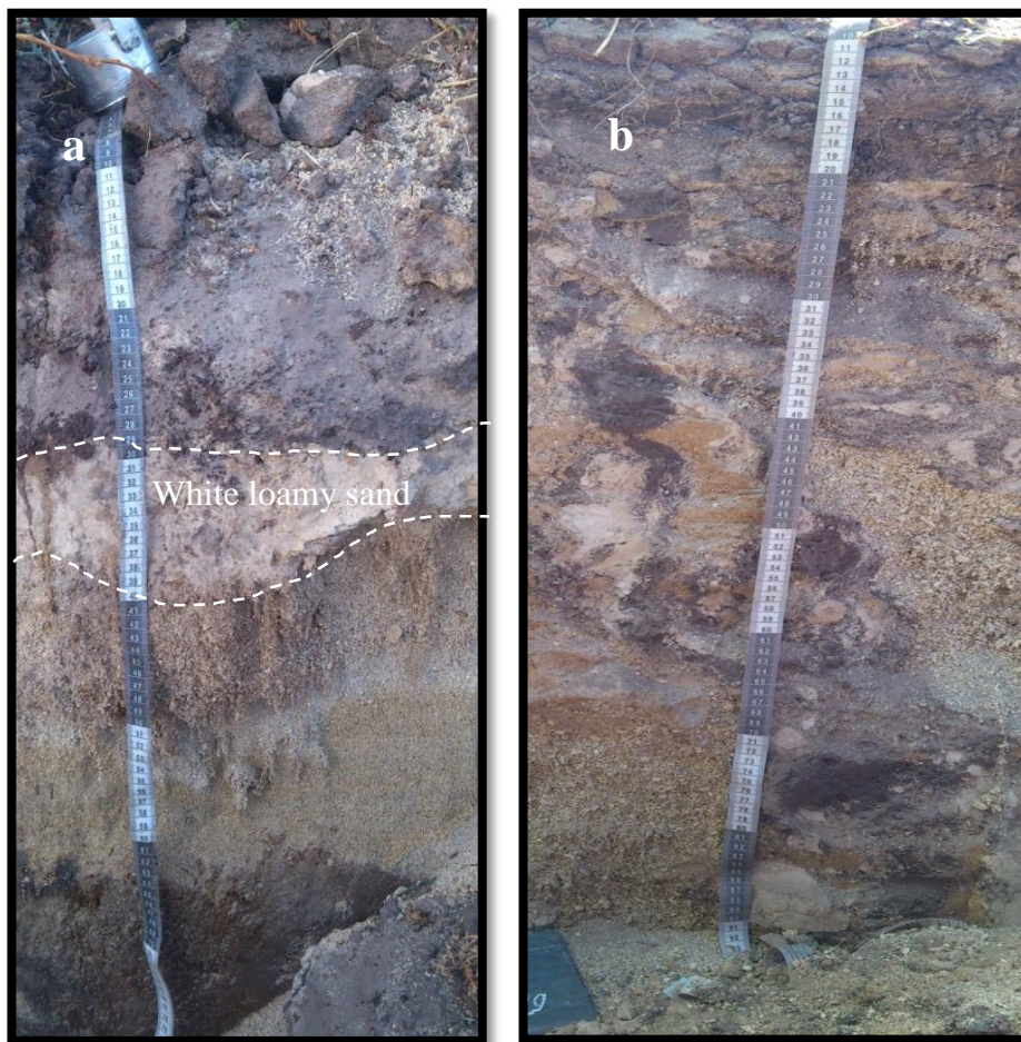
Figure 4.6: Typical soil profiles at site 3, (a) undisturbed area, an example of the lenses of white loamy sand between the (b) flipped areas.
