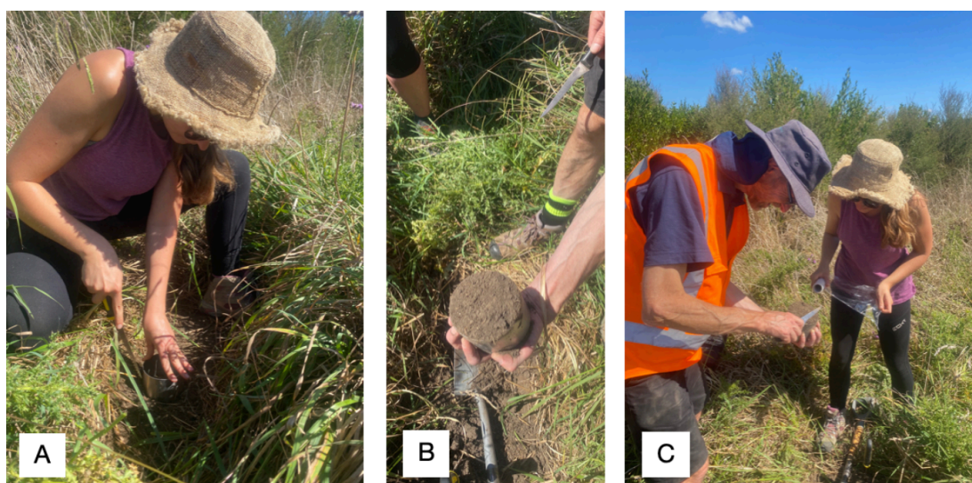
Figure 3.7: Soil coring process. (A) digging the core into the soil with the help of a serrated knife. (B) the soil core, just removed from the ground. (C) wrapping the core for safe transport and storage.
