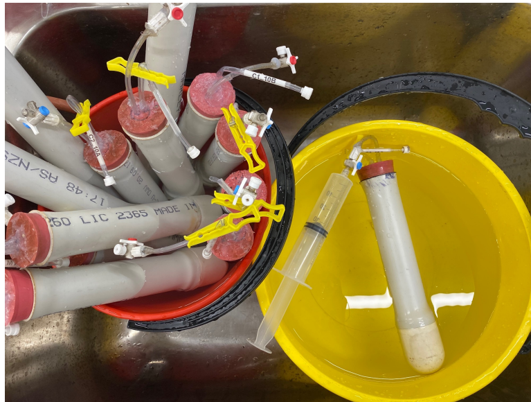
Figure 3.13: Lysimeters being tested for air leaks and vacuum-holding capacity
