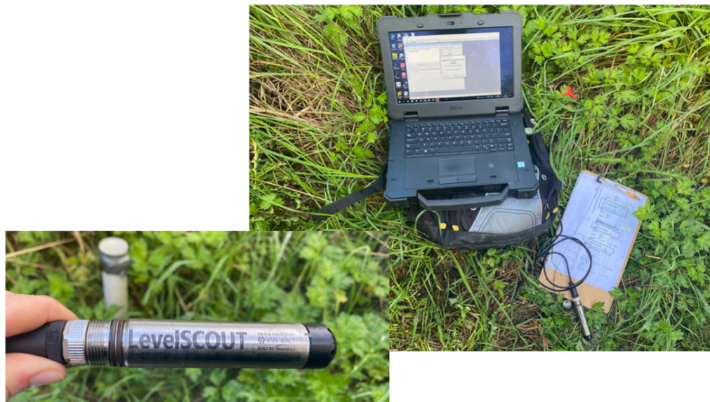
Figure 3.11: Extracting data from the LevelSCOUT data logger in dip well “C”
