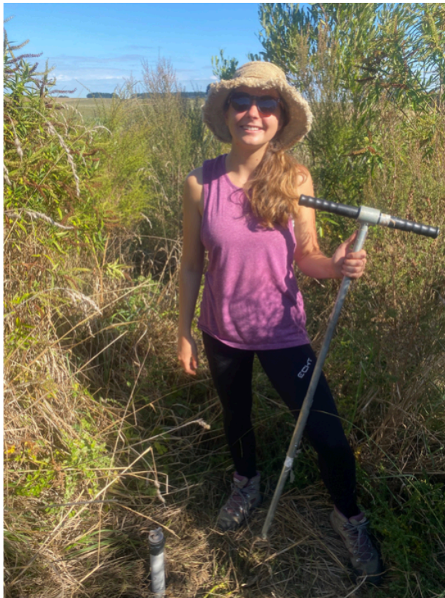
Figure 3.9: Installation of dip well C. Pictured with dutch auger.
