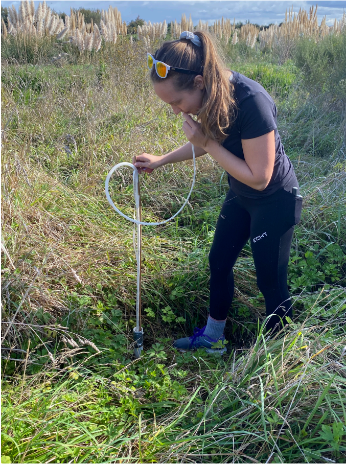
Figure 3.10: Collecting water table measurements at plot C2 using the “bubbler”
