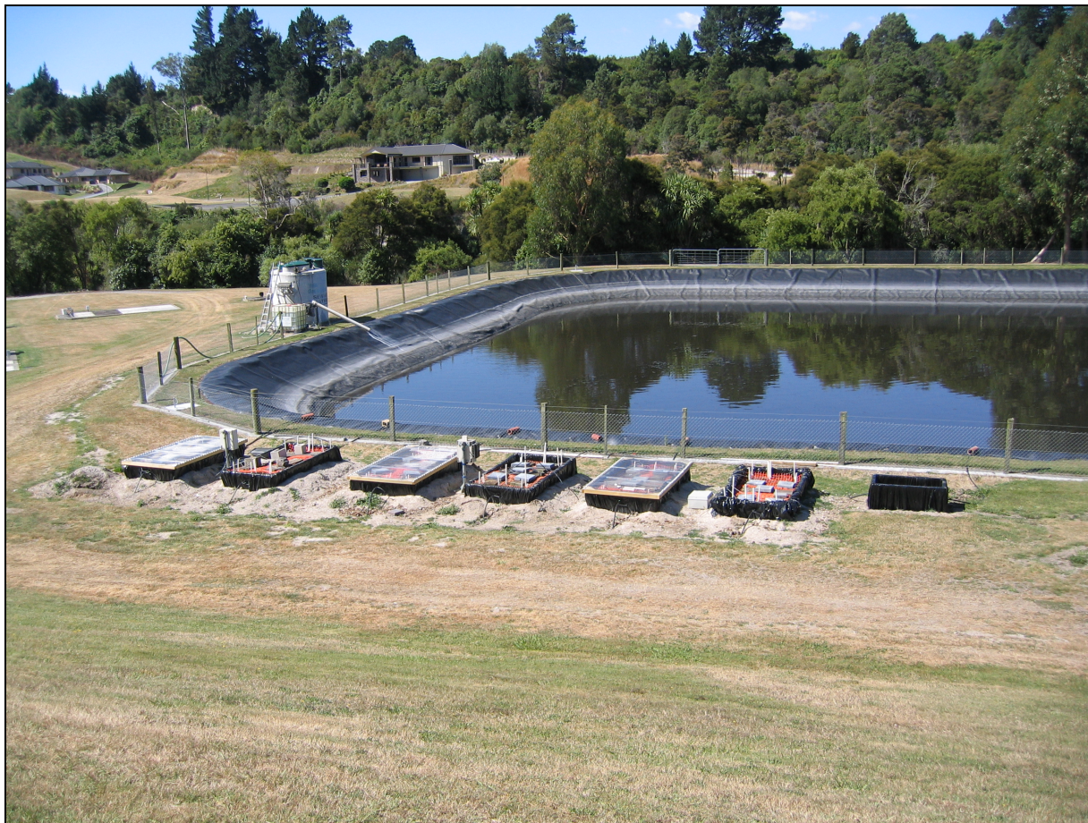
Figure 5.1 – Photograph of pilot scale denitrification bed trial. The poly-carbonate solar covers are on first (bed 1), third (bed 3) and fifth (bed 5) beds from the left. The 15 mm diameter white PVC tubes that can be seen protruding from beds 2, 3 and 5, housed the temperature probes. The loggers and batteries used to record temperature measurements were housed in three instrument boxes located between beds 1 and 2, beds 3 and 4, and beds 5 and 6 (lying on ground). The 5000 L SAF plant can be seen in the background on the left-hand side of the storage pond. The effluent from the beds discharged, by gravity drainage, into the storage pond.
