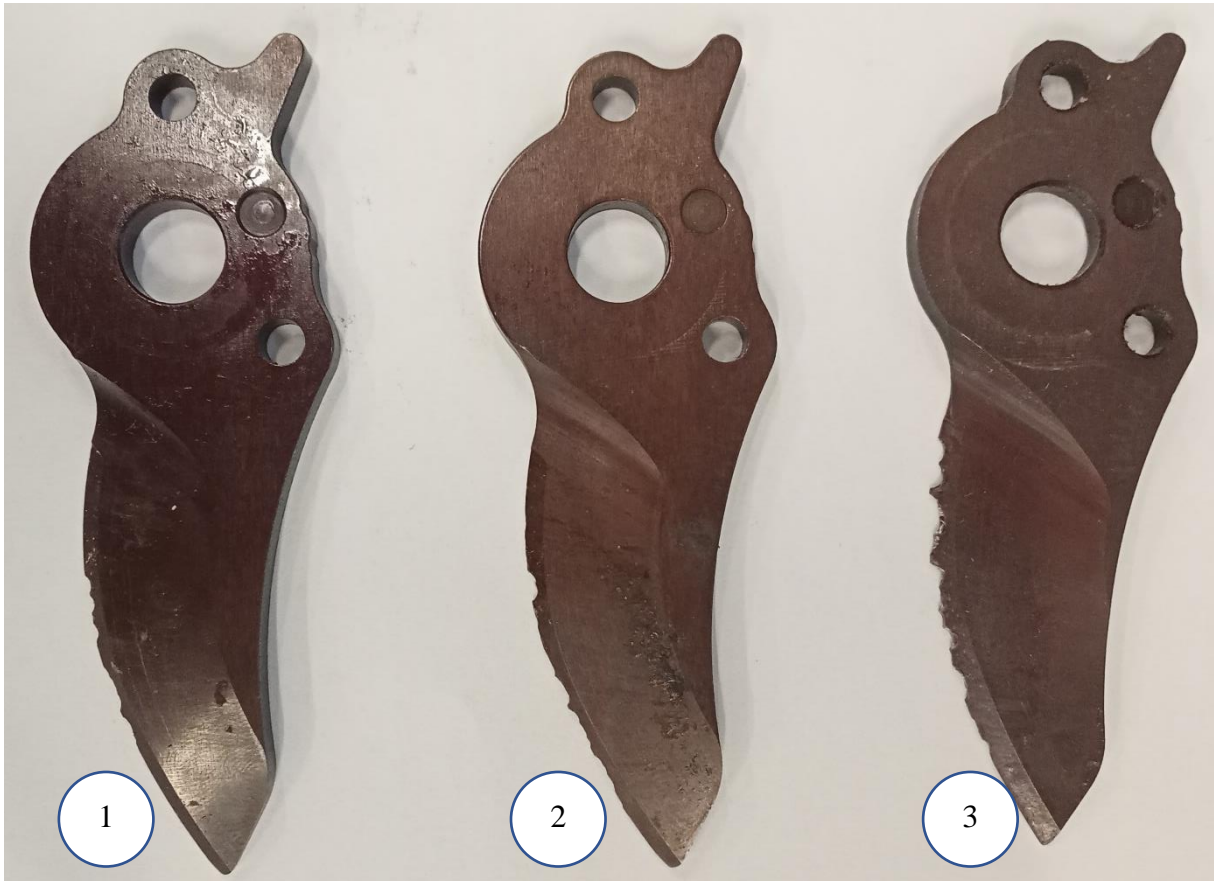
Figure 4-7 - Blade damage of Configurations 2 and 1
