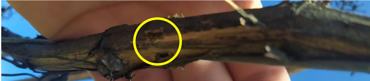
Figure 4-12 - Puncturing of canes caused by Configuration 1
