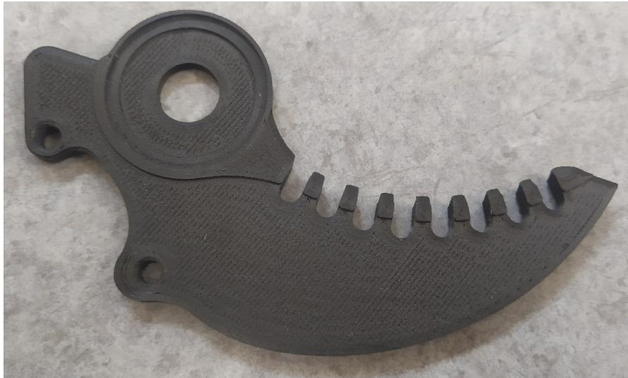
Figure 3-10 - Onyx 3D printed anvil for test fitting
