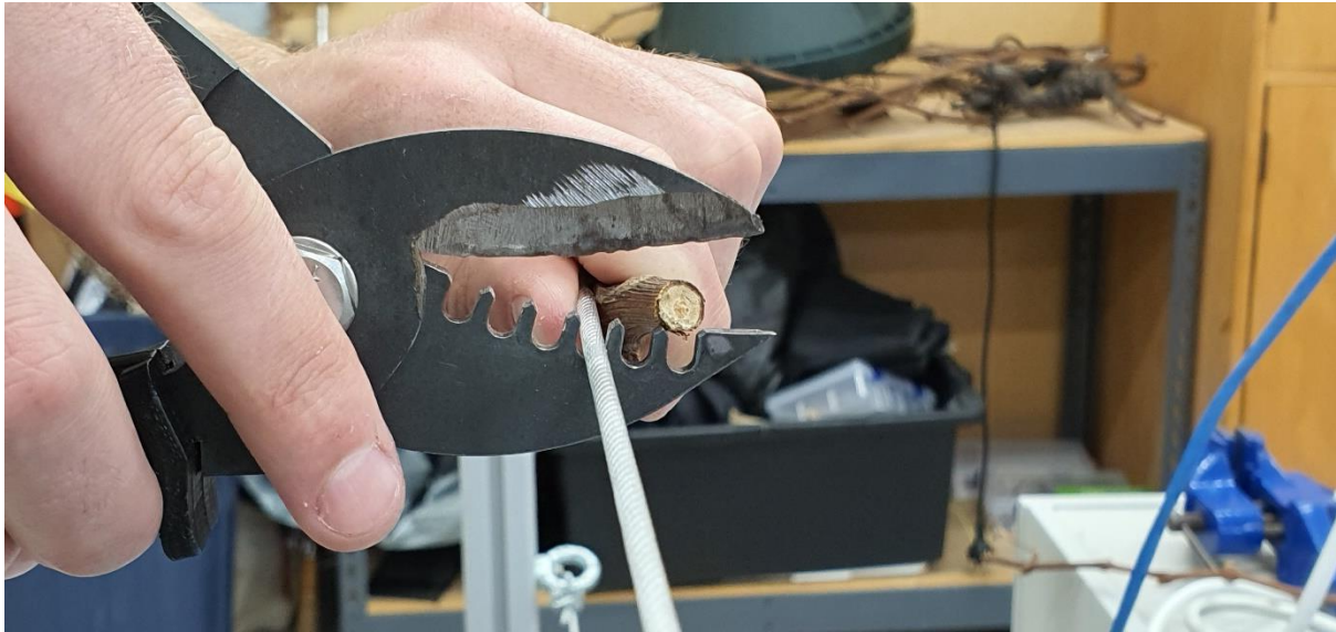
Figure 3-4 - Testing the Barracuda tooth profiles
