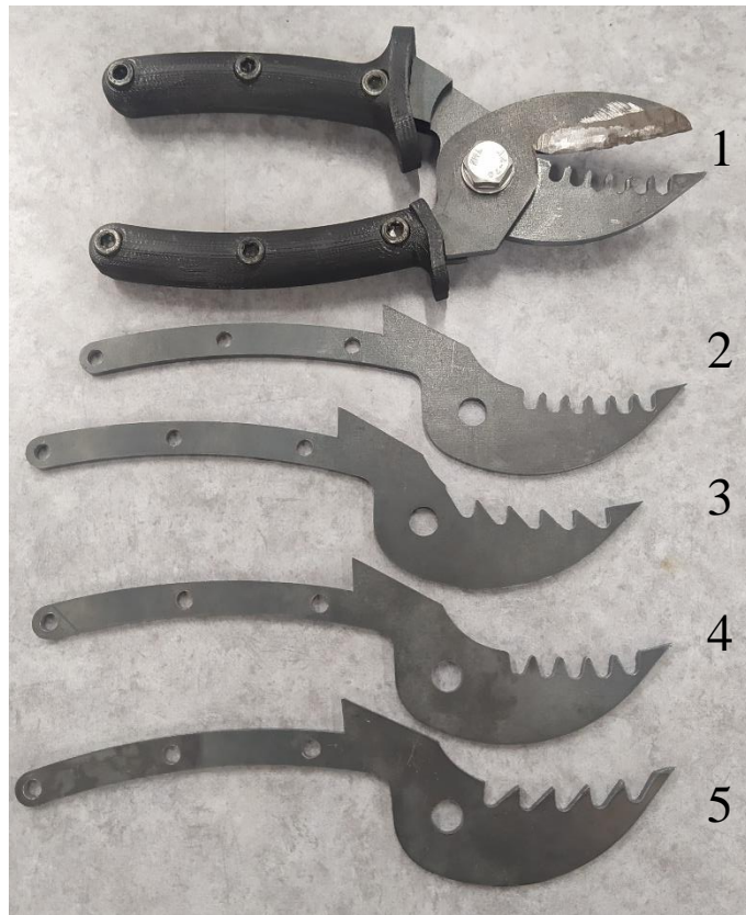
Figure 3-3 - The five Barracuda dirty prototypes labelled 1-5
