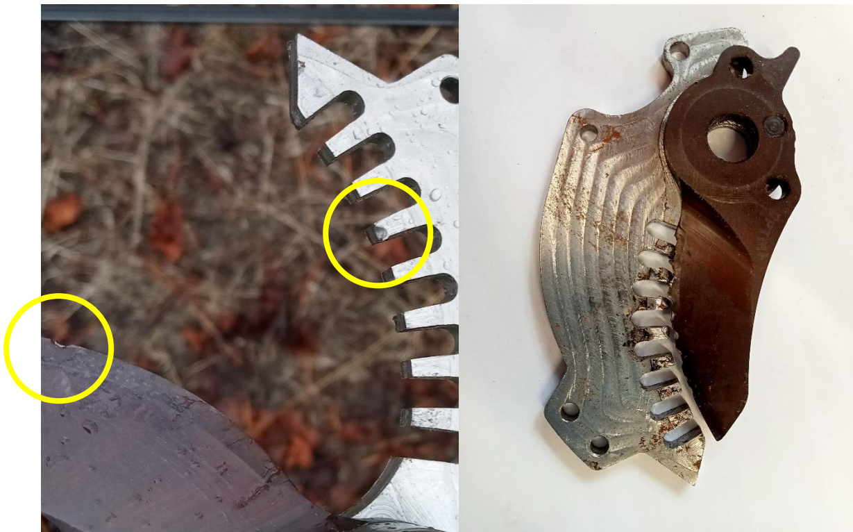
Figure 4-4. Blade damage caused by collision with the guide wire (Left) on Configuration 1. Aggregate blade damage (Right).
