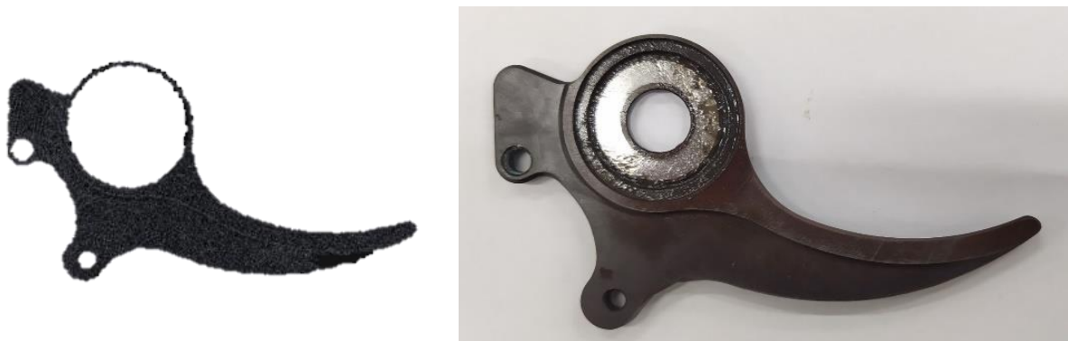
Figure 3-9 - Stock Anvil 3D Scan Point Cloud and isolated original
