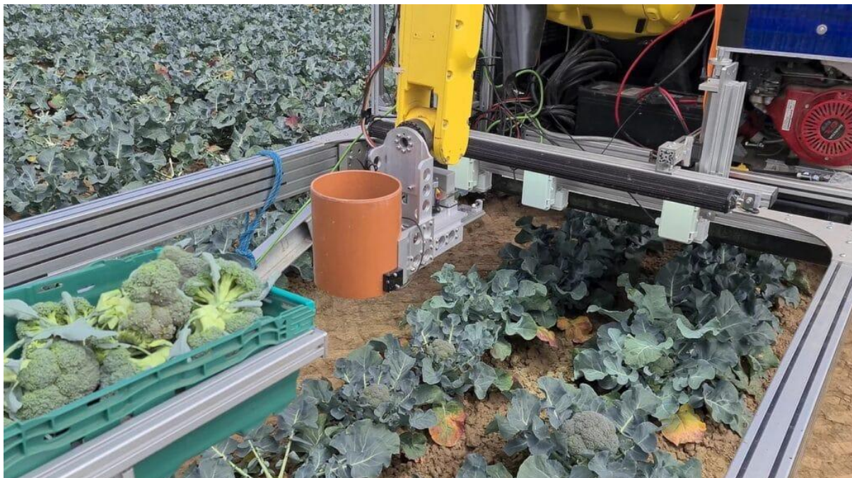
Figure 2-6 - RoboVeg Autonomous Broccoli Harvester. End effector shown on the end of the yellow manipulator
