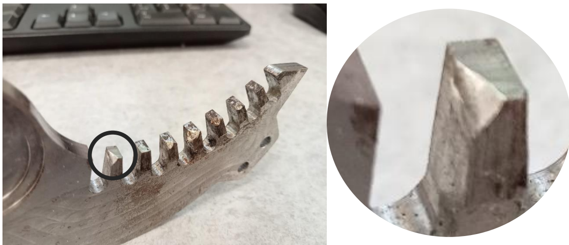
Figure 4-8 - Damage to teeth on Configuration 1, overall view (Left), with detail view (Right)
