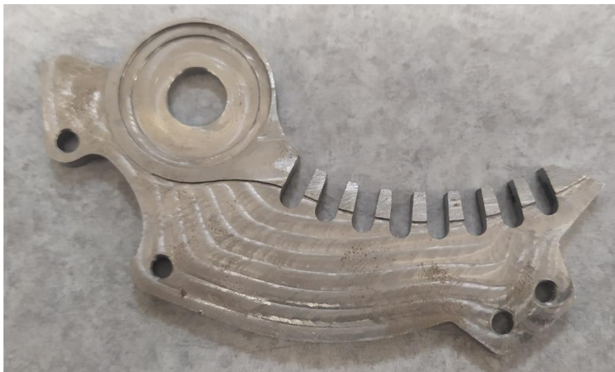
Figure 3-11 - CNC machined anvil for Configuration 1 with additional machining stability holes
