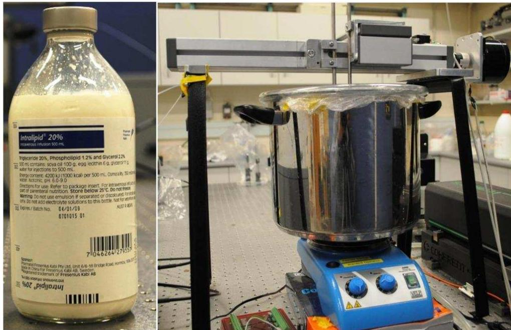
Figure 47 Intralipid 20% bottle along with the sample container setup.
