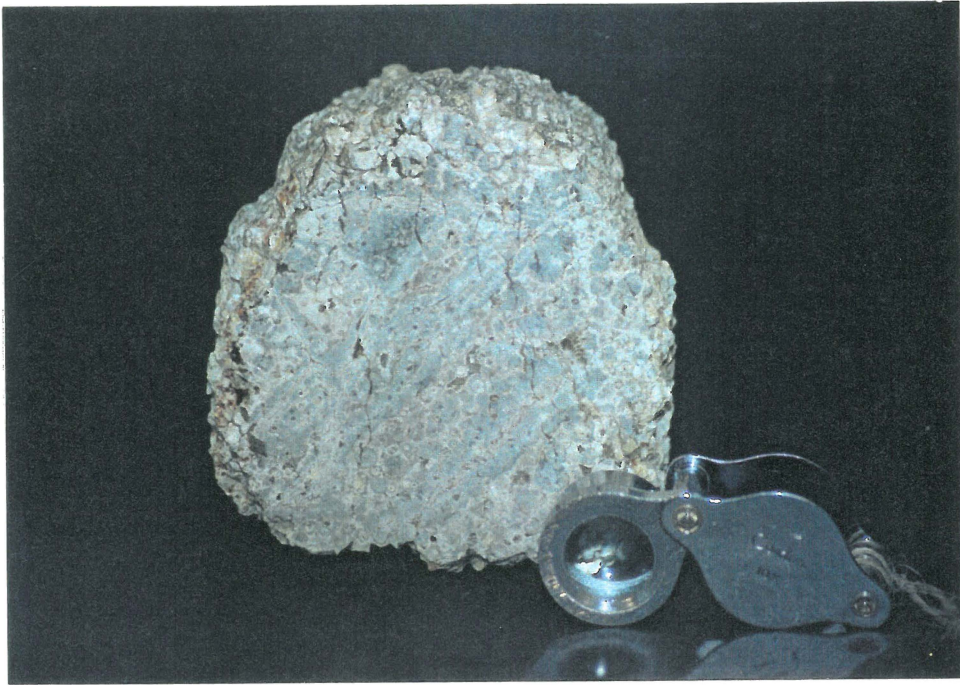
Figure 2.16. Well developed spherulitic textures within the biotite rhyolites of the Eastern Flows (sample W941263; T12 670492). Magnifying lens is 7cm long.
