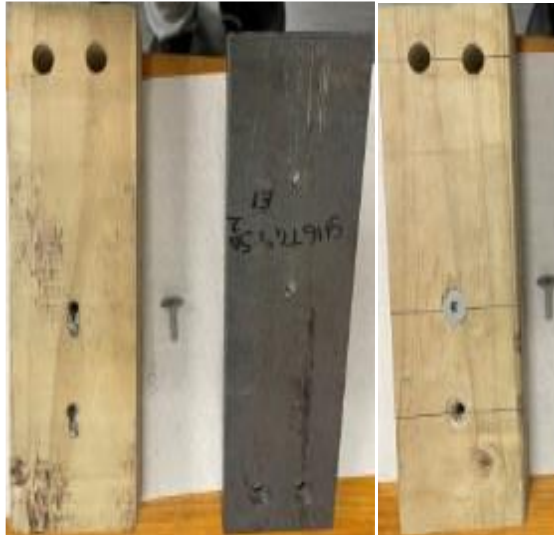
(b) Post-tested samples
