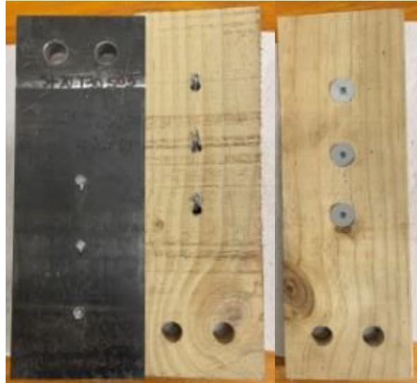
(b) Post-tested samples
