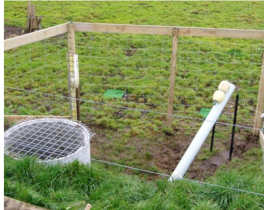
Figure 2.9: A floating decant structure suspended by a pin and two waratahs, June 2012.
