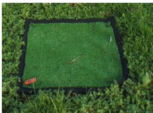
Figure 2.16: A synthetic turf mat used for capturing sediment in the DB ponding basins.
