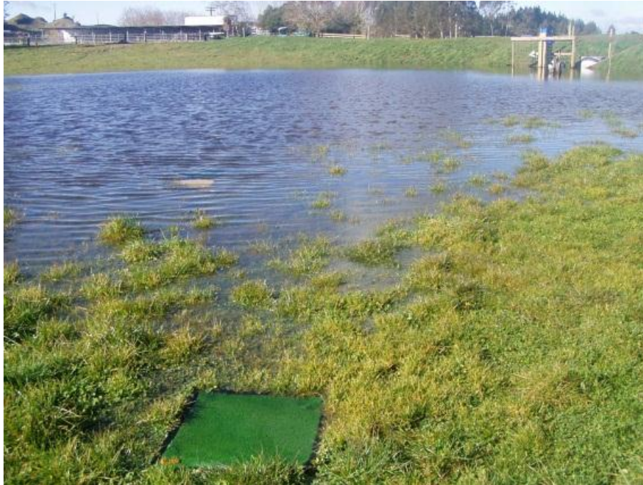
Figure 2.18: Sediment mat ready for collection at Hauraki DB after a ponding event in July, 2012. Although this mat looks clean, sediment had been deposited.
