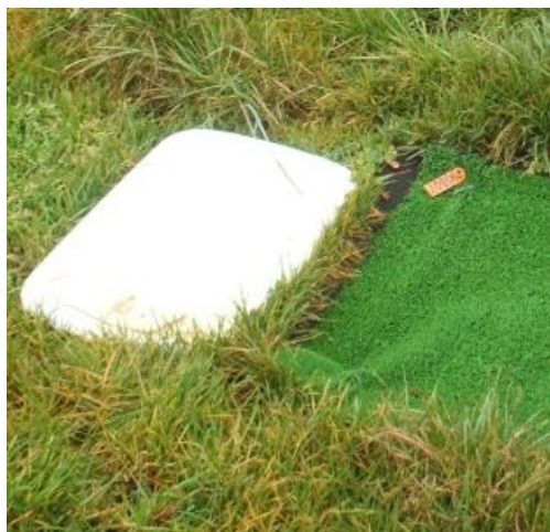
Figure 2.19: Sediment tray deployed next to a mat to capture sediment deposited at Hauraki DB, 2012.
