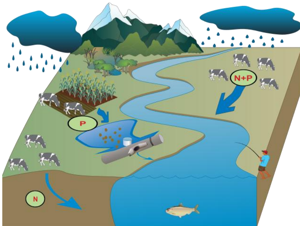
Figure 1.5: Schematic diagram showing the key nutrient pathways including phosphorus in overland flow and nitrogen infiltration through the soil. A detainment bund intercepting runoff water from a cultivated and grazed paddock is shown.
