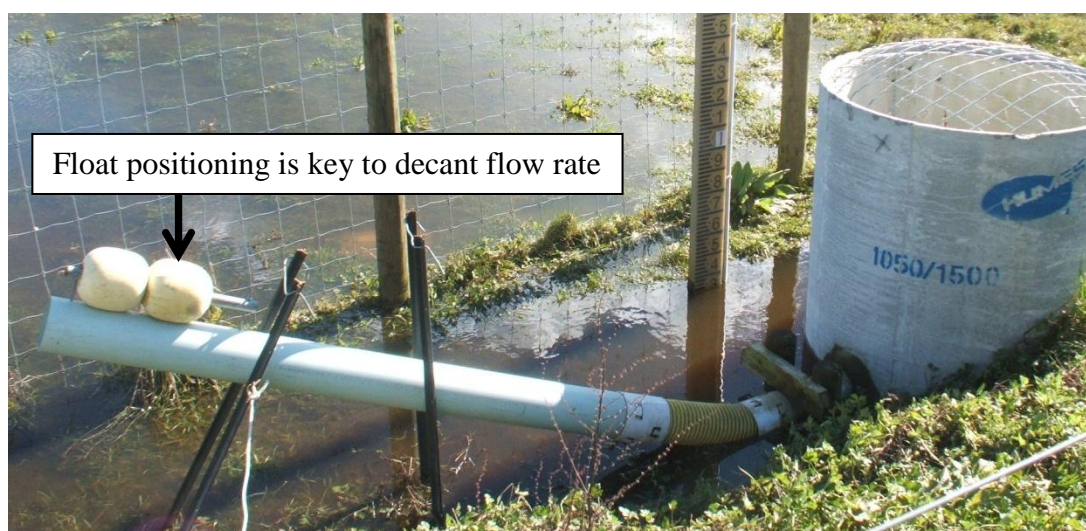
Figure 4.3: Floating decant structure used at Waiteti DB. Further trials are needed to optimise the decant design.
