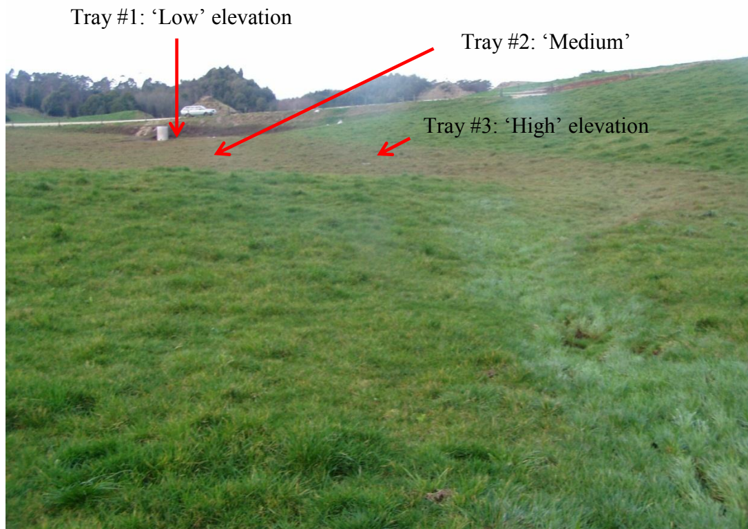
Figure 4.1: Awahou DB after a ponding event in July (July #3). Approximate location of trays are depicted by the red arrow. Elevations of the trays were 100 mm (Tray 1), 600 mm (Tray 2) and 900 mm (Tray 3) relative to ground 0 in the basin at the low elevation. Note the distinct evidence of sediment settling in the basin and the water level line on the bund wall.
