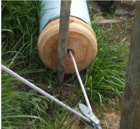
Figure 2.8: Plug and pulley system, prototype #1, for controlled residence time, March 2012.
