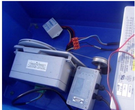
Figure 2.11: Water level recording system (in the blue box seen in Figure 2.10); as water level rises, pulley wheels turn the encoder (left) and data are logged on the Iris 150g (right). Hauraki DB, July, 2012.
