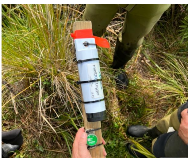
Figure 3: Deployment of dissolved oxygen and temperature loggers within the wetland study reach. (Left) Loggers secured to a stake prior to installation at one of two sites. (Right) Placement of a logger at a monitoring site (T6) within the wetland system. Loggers recorded dissolved oxygen ( \text{mg L}^{-1} ) and temperature ( ^{\circ}\text{C} ) at hourly intervals.
