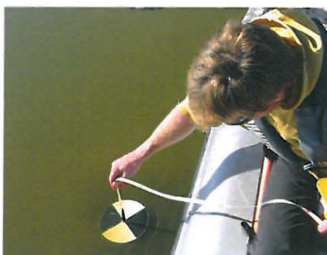
Figure 3. Measuring Secchi depth in Lake Koromatua.
