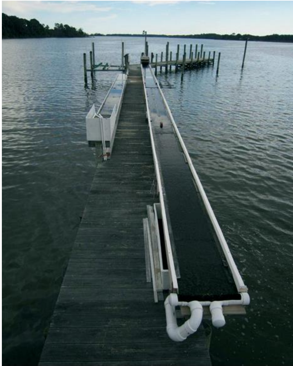
Figure 1.2: Fiberglass trough ATS floways on the Great Wicomico River off the Central Chesapeake Bay. The left floway is 0.61 m wide x 15.2 m long with a 1% slope; the right floway is 0.61 m wide x 24.4 m long with a 2% slope (after Adey et al., 2013)
