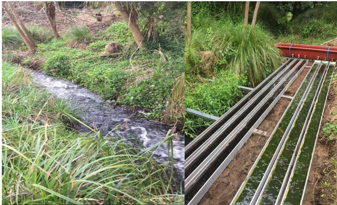
Figure 5.1: The farm stream and the 6 replicate FANS installed along the stream used in Experiment 1. Pumped stream water was distributed between the FANS using a sump with six adjustable valves
