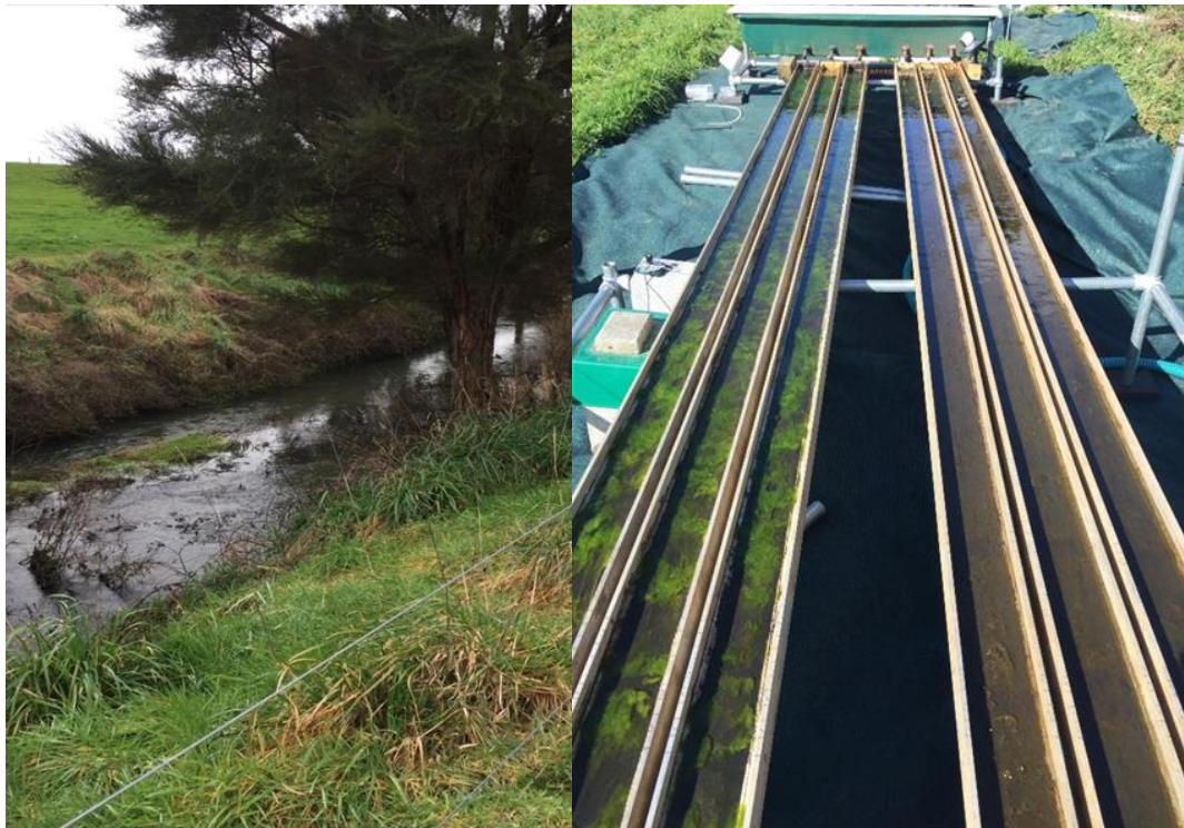
Figure 5.2: The farm river and the 6 replicate FANS installed along the river used in Experiment 2. Pumped river water was distributed between the FANS using a sump with six adjustable valves
