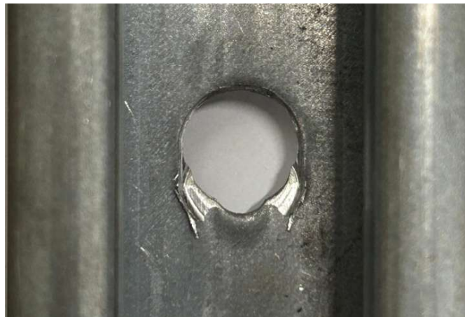
Fig. 23. CFS specimen deformation
