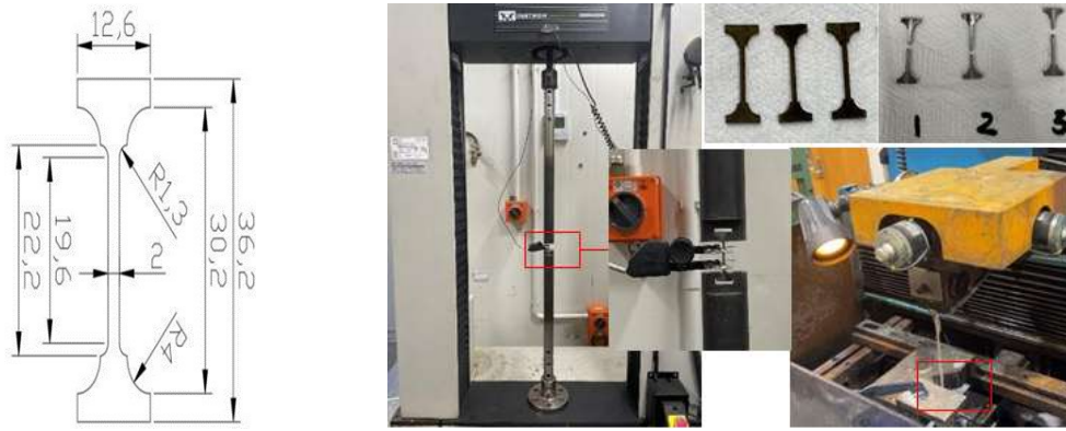
Figure 7 Steel coupon sample preparation.
