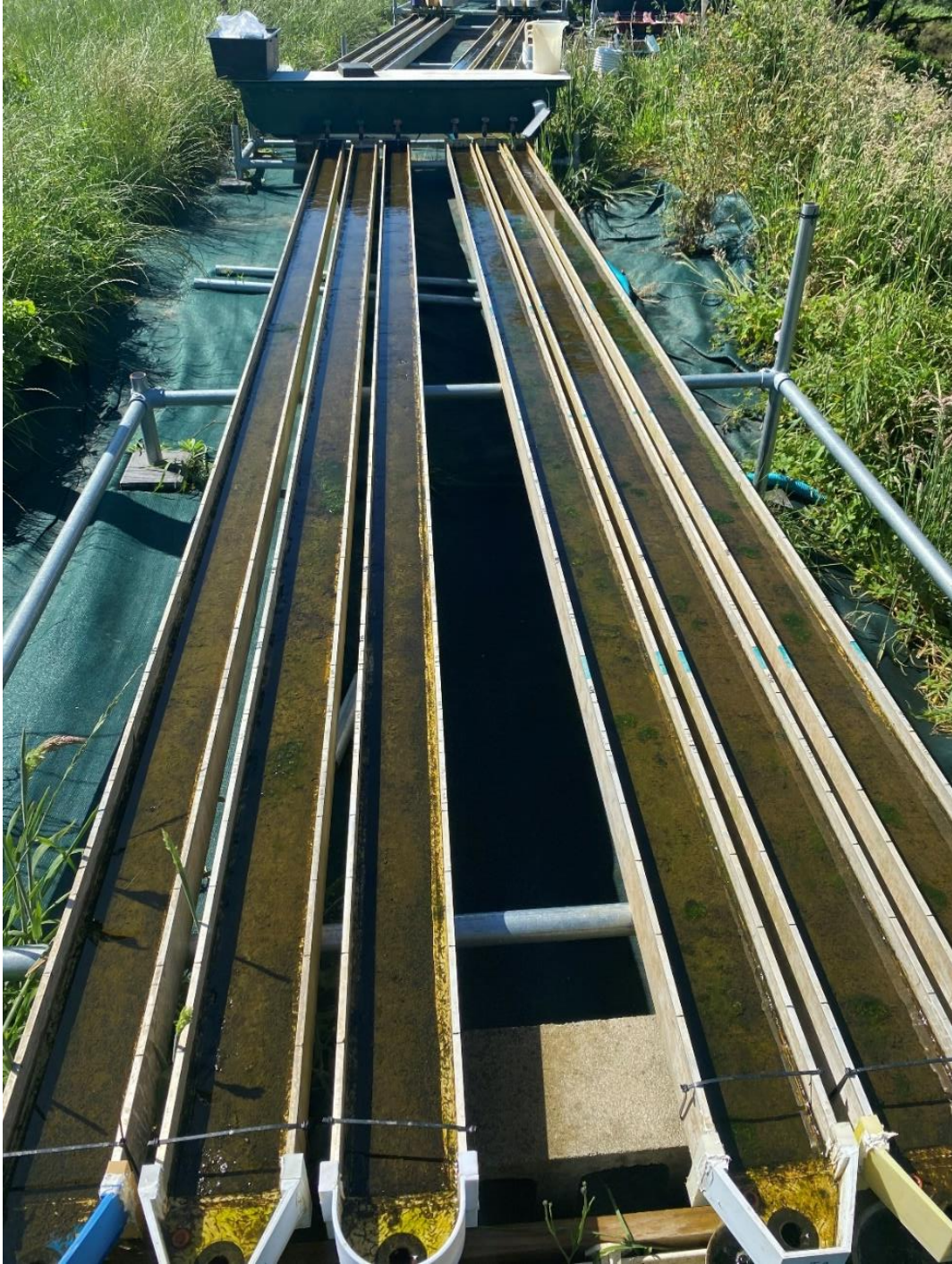
Figure 1.2: (Original photo) Outdoor-scale Filamentous Algal Nutrient Scrubber (FANS).
