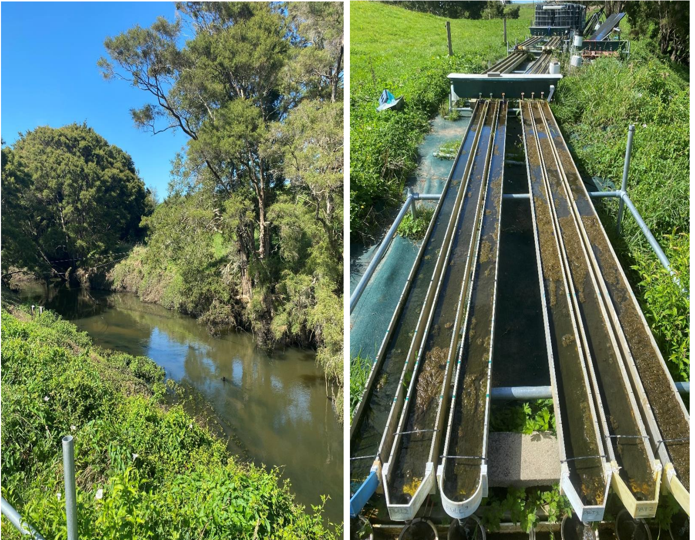
Figure 2.1: (Left) Study site (Paehau Trust farm) and Toenepi Stream. (Right) The FANS system experiment set-up along the stream bank. FULL harvest replicate flow-ways on the left-hand side and PARTIAL harvest replicate flow-ways on the right-hand side, closest to the stream.
