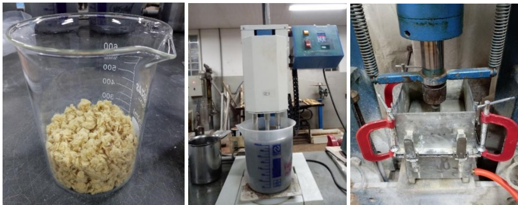
Figure 2 – Processes used to produce the fibre-cement boards. a) Sisal microfibres; b) Slurry mixing process; c) compression of composite after moulding.
