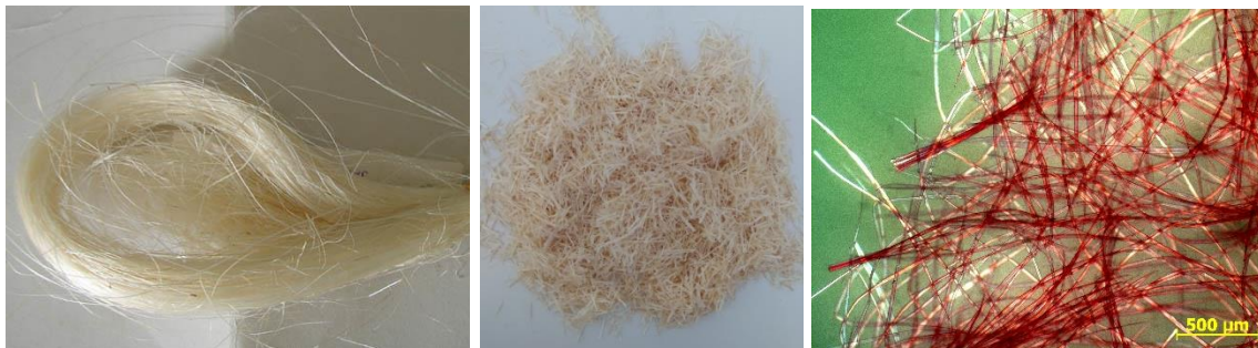
Figure 1 – From left to right: as-received fibres, chopped fibres before treatment and optical microscopy image of microfibrils after defibrillation.
