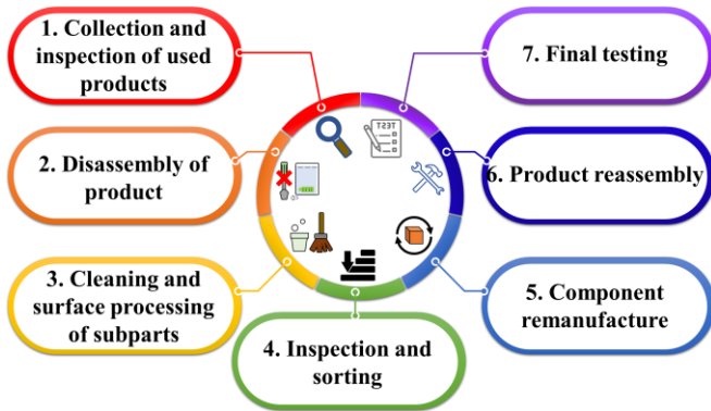
Fig. 3 Key steps of remanufacturing.
