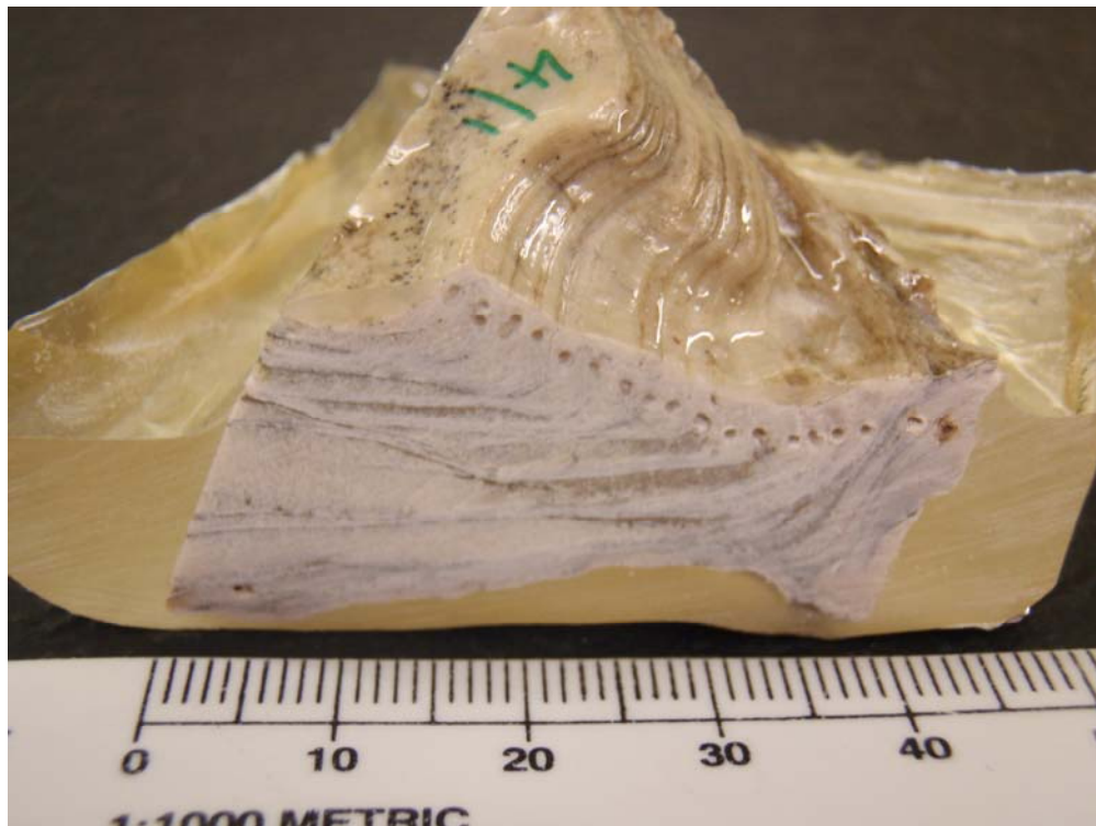
Figure 6.7 Sample PAT4/1 set in resin with drill holes for isotopic analysis taken under the ligamental area (see Fig. 6.6) using a Dremel drill.
