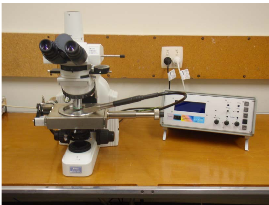
Figure 2.1 Cathodoluminescence stage, microscope and control unit set up at the University of Waikato.
