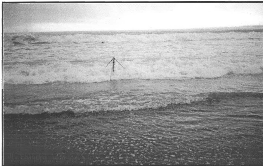
Figure 4.7 — GTS installed at Westshore on 12 March 1999. Note the direction of the rear leg of the frame facing away from the direction of wave approach.
