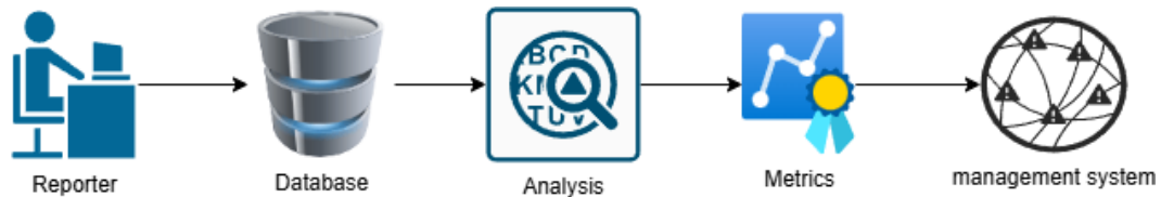
Figure 4.1: Vulnerability Management Process: The process begins with reports from assumed good-faith reporters. These reports are stored in a database with assigned metadata and subsequently analyzed by security analysts. Following the analysis, the vulnerabilities are assigned metrics that assist in their triage. End-users leverage these metrics to prioritize vulnerabilities for mitigation within their management systems.
