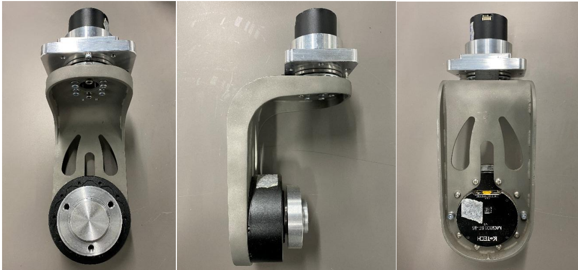
Figure 4-3 Assembled drive-steering system integrated into the test vehicle
