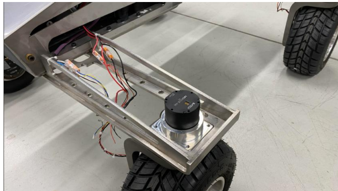
Figure 4-10 Sliding mechanism of the drive-steering assembly within the wheel support beam
