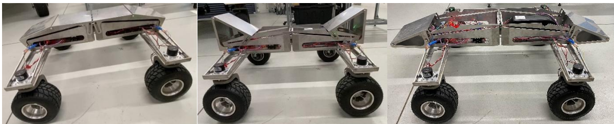
Figure 4-22 a. fully closed cover b. partially opened cover c. fully opened cover
