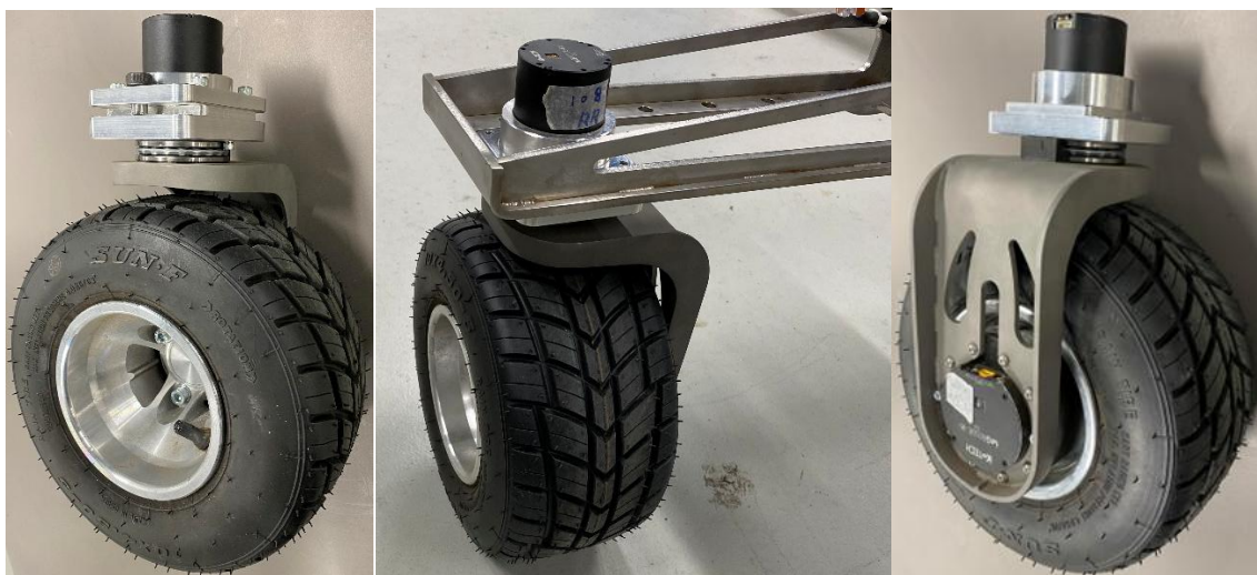
Figure 4-1 Drive-steering system of the test vehicle
