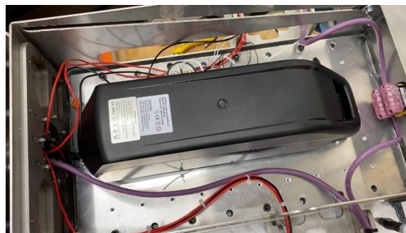
Figure 4-19 DC battery mounted on the electronics mounting plate
