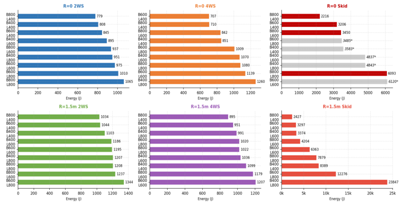
Figure 6-33 Energy ranking by steering mode - configurations sorted from most to least efficient. Asterisked grey bars represent failed/invalid R=0 Skid Steer tests.
