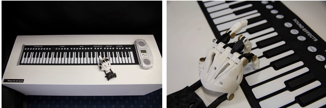
E19 - Close-ups of the 3D-printed hand playing a piano keyboard in Set 6.
