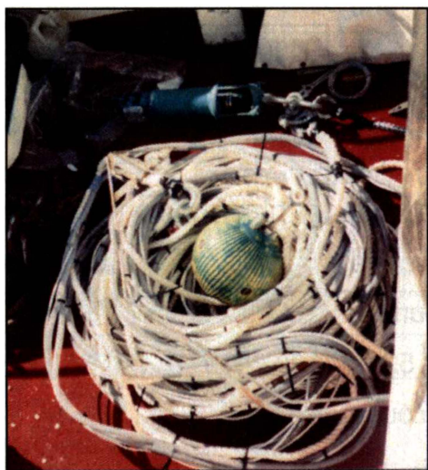
Figure 2-7: The S4P current meter, mooring line and acoustic release set prior to deployment off Port Stephens in November 1996.
