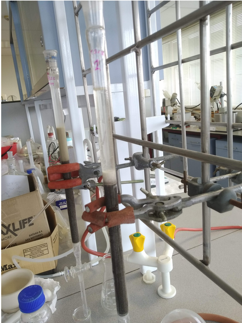
Figure 2.2: RPR column leaching set up
