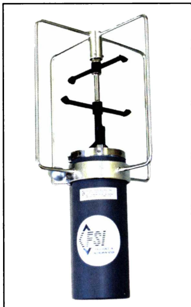
Figure 3.1: 3D-ACM WAVE in protective frame
