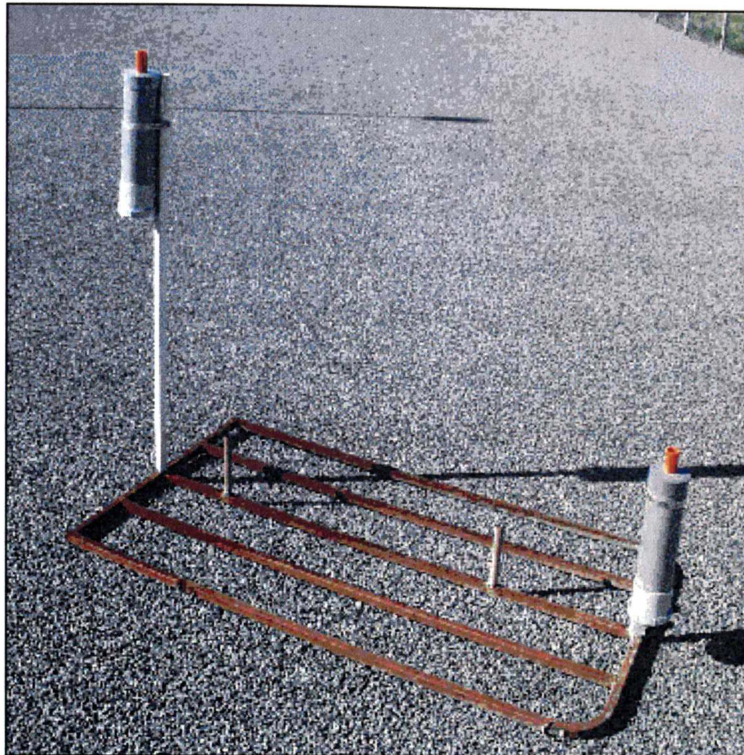
Figure 2.5: Sediment trap array on seabed frame.
