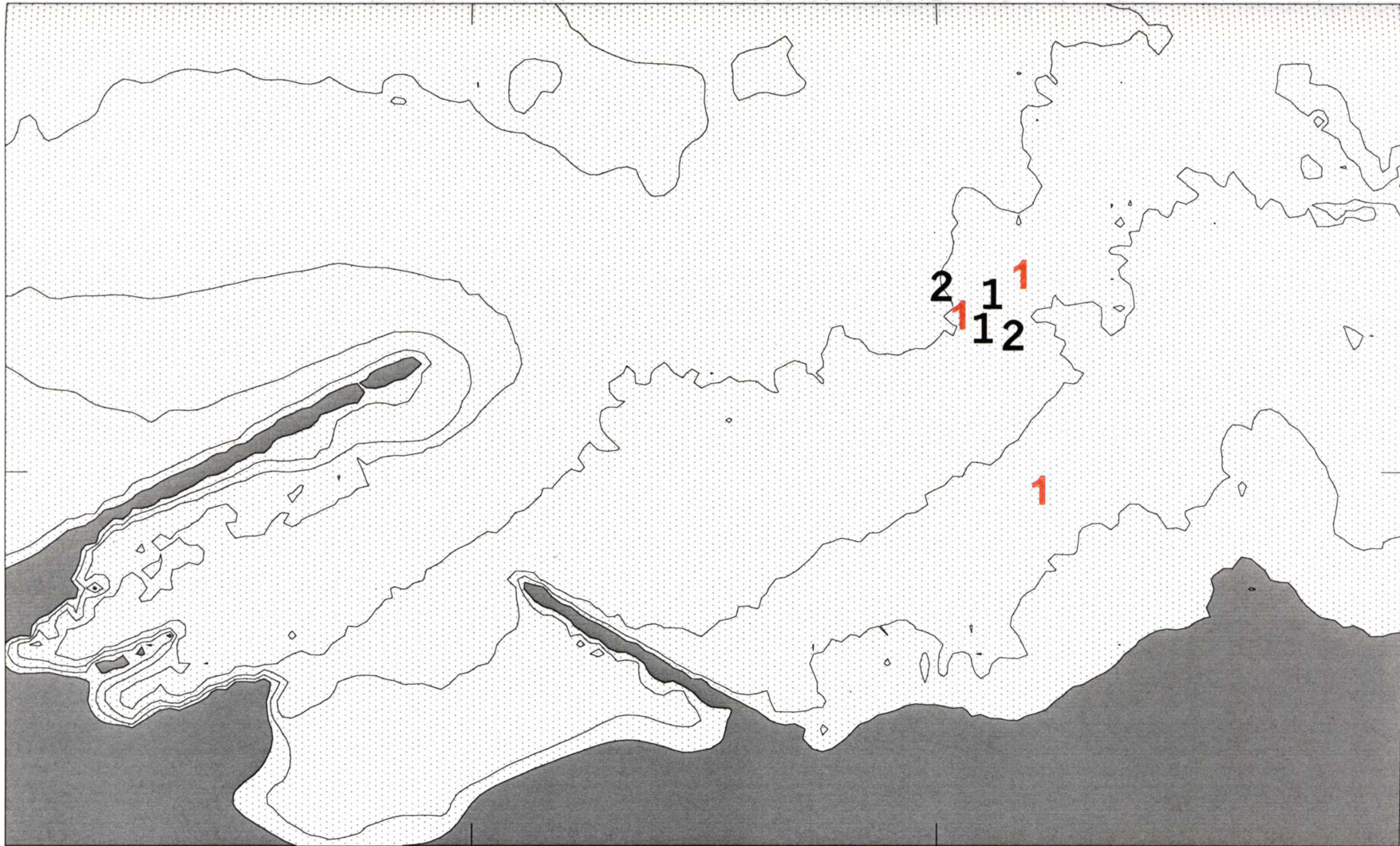
Figure 15 Results of video analysis of tracer samples collected in sample periods 2 & 3 (Days 10 & 13) with grain size <120\mu\text{m} . Red tracer is represented by red numerals, yellow tracer is represented by black numerals.
