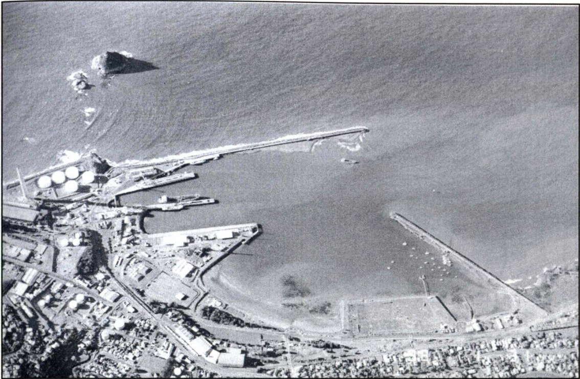
Figure 1.6: Aerial photograph of Port Taranaki showing the present-day layout (March, 1998). The split-hopper dredge Pelican can be seen dredging on the breakwater tip-shoal (photo by J. Kito, Taranaki Regional Council)
