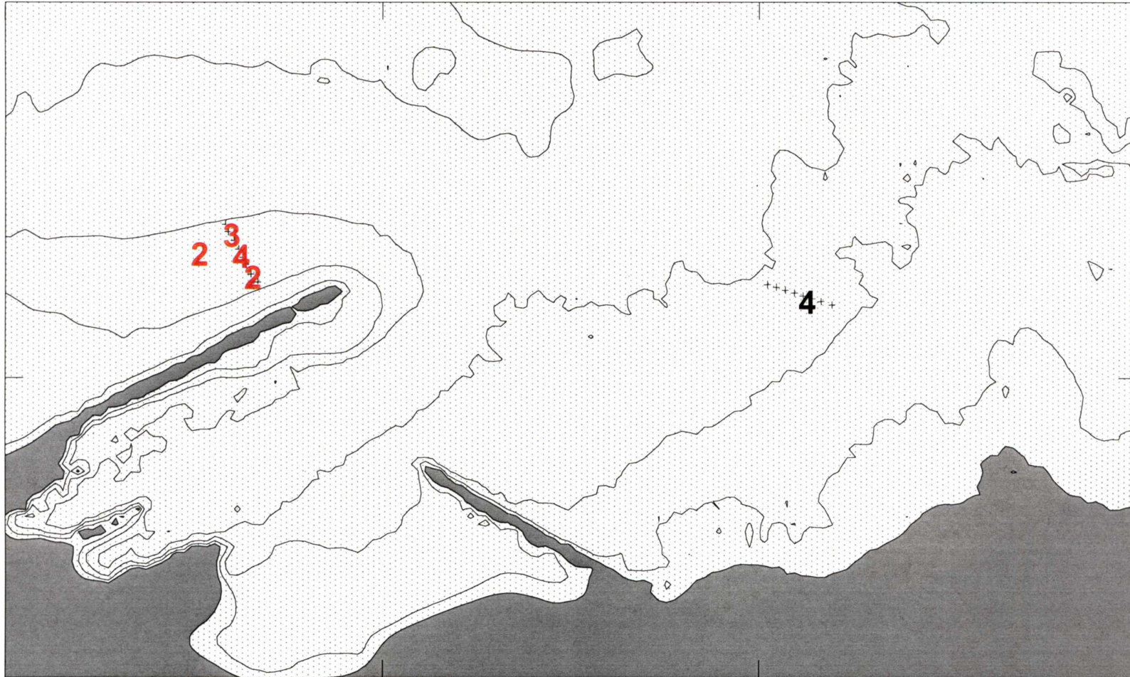
Figure 18 Results of video analysis of tracer samples collected in sample period 4 (Day 18) with grain size <120\mu\text{m} . Red tracer is represented by red numerals, yellow tracer is represented by black numerals.
