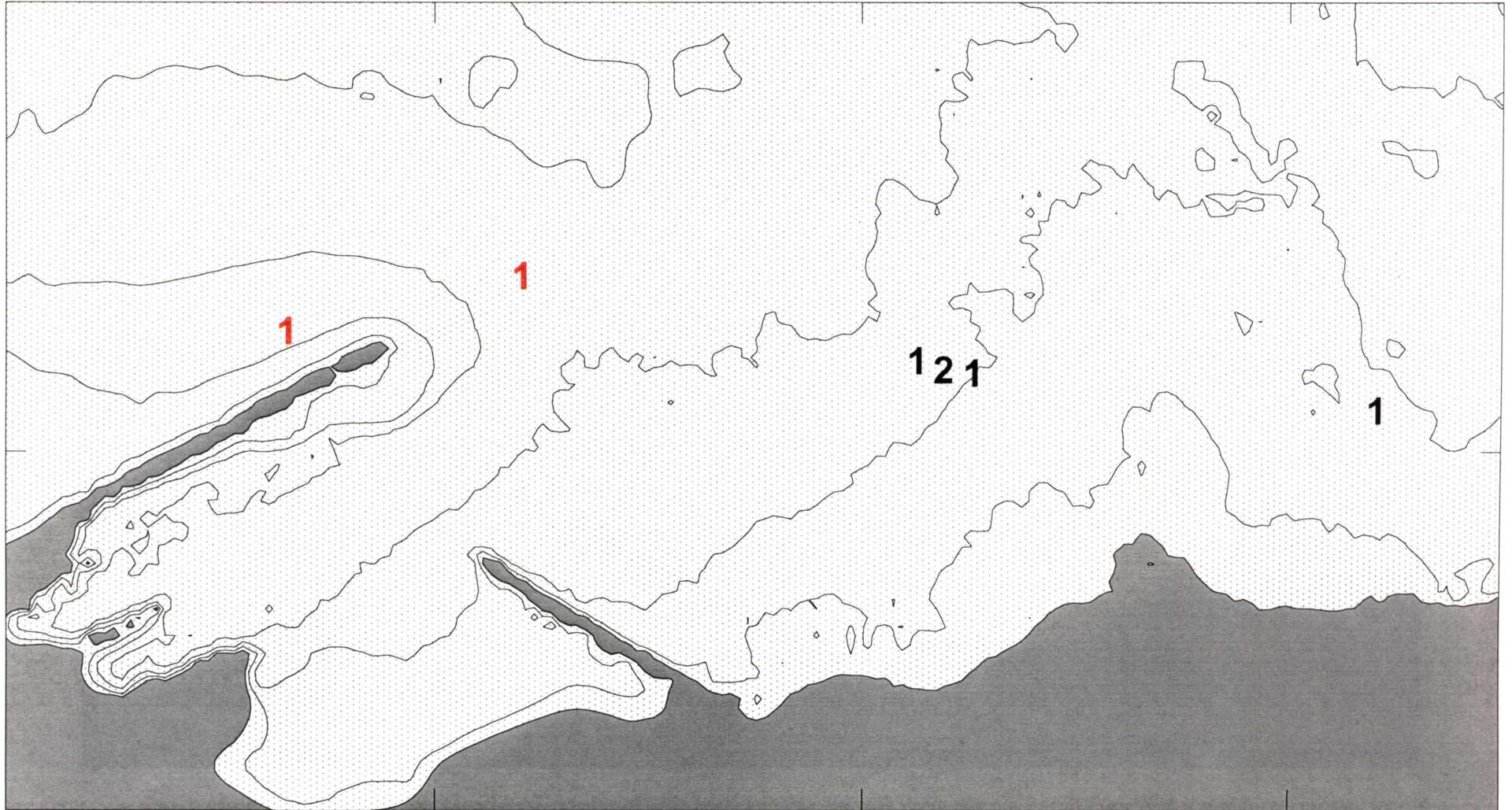
Figure 27 Results of video analysis of tracer samples collected in sample period 6 (Day 49) with grain size <math><200 - >120\mu\text{m}</math>. Red tracer is represented by red numerals, yellow tracer is represented by black numerals.
