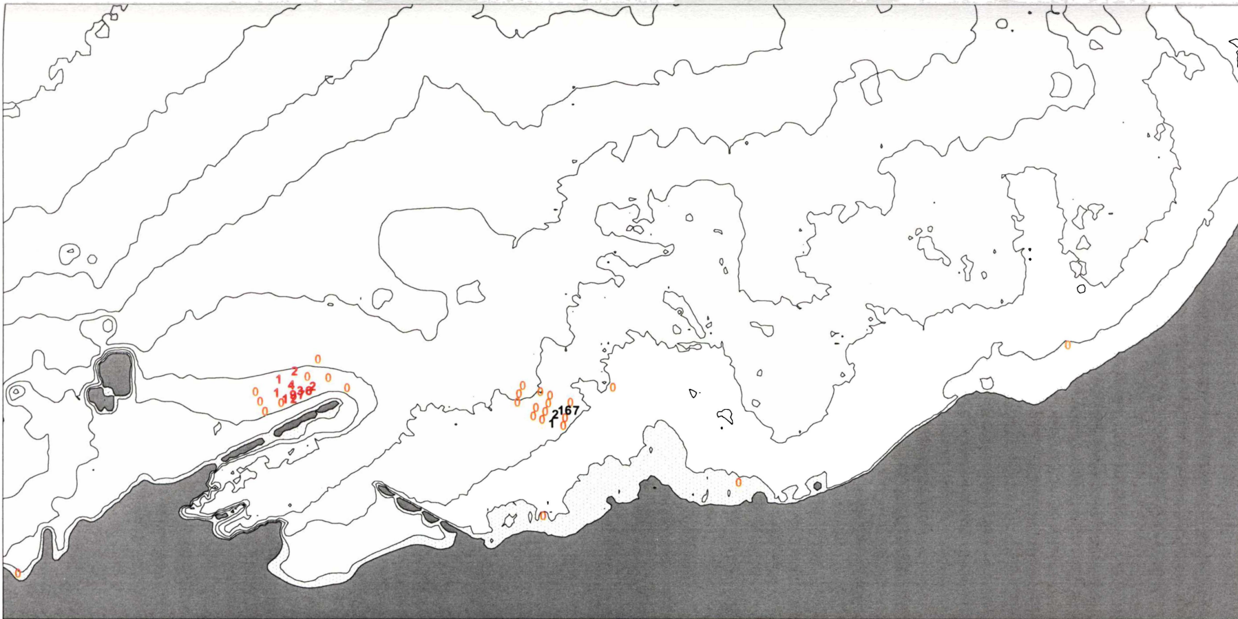
Figure 1 Results of visual analysis of tracer samples collected in sample period 1 (Day 4). Red tracer is represented by red numerals, yellow tracer is represented by black numerals and orange zeros indicate locations where no tracer was found.
