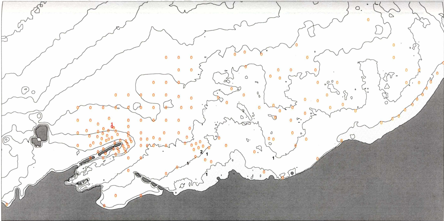
Figure 10 Results of visual analysis of tracer samples collected in sample period 11 (Day 308). Red tracer is represented by red numerals, yellow tracer is represented by black numerals and orange zeros indicate locations where no tracer was found.
