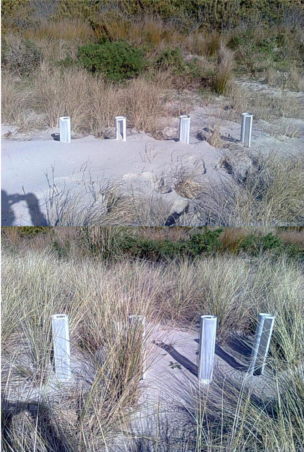
**Figure 5.10:** Images showing the deposition of sand around sediment traps following the first period of their deployment from the 15<sup>th</sup> of June to the 29<sup>th</sup> of July 2010. Top image shows site B, deposition amongst *Spinifex* plants. Bottom image shows site A, deposition around *Ammophila* plants.
