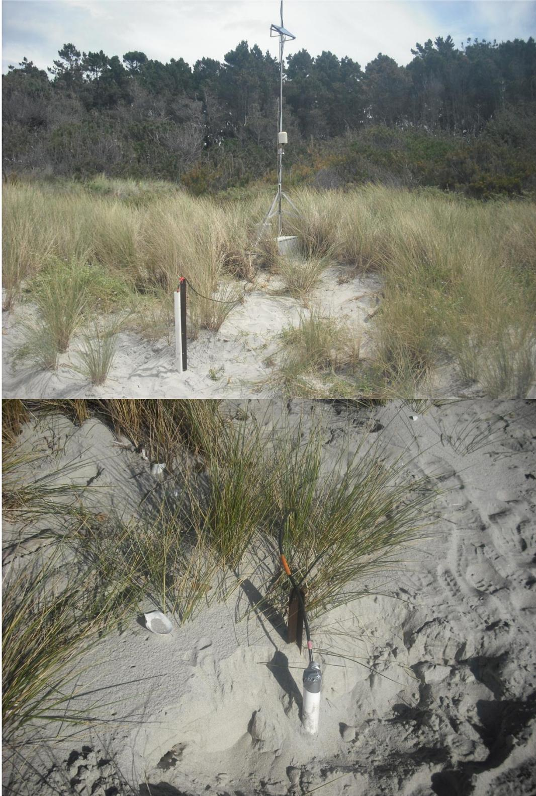
**Figure 5.8:** Images showing the deposition of sand around piezometers over a period of this study from the 15<sup>th</sup> of June to the 16<sup>th</sup> of October 2010. Top image shows initial sand level at site A piezometer 15<sup>th</sup> June. Bottom image shows sand level at site A piezometer 16<sup>th</sup> October after some sand has been dug away.
