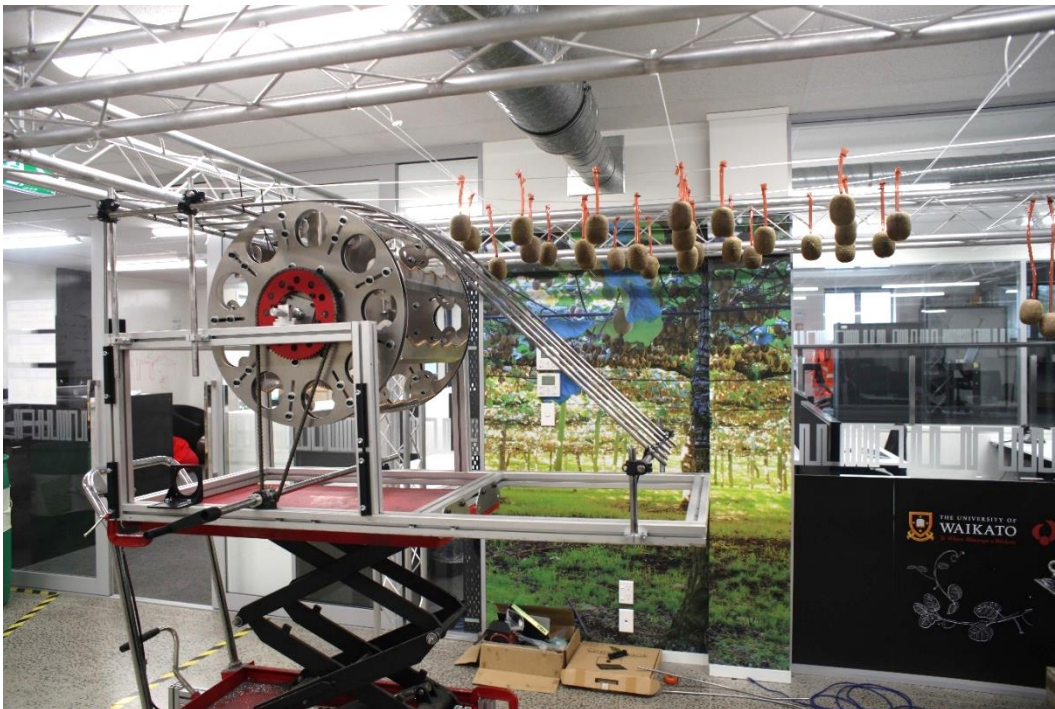
Figure 36: Non-selective harvester lab testing with silicone kiwifruit models
