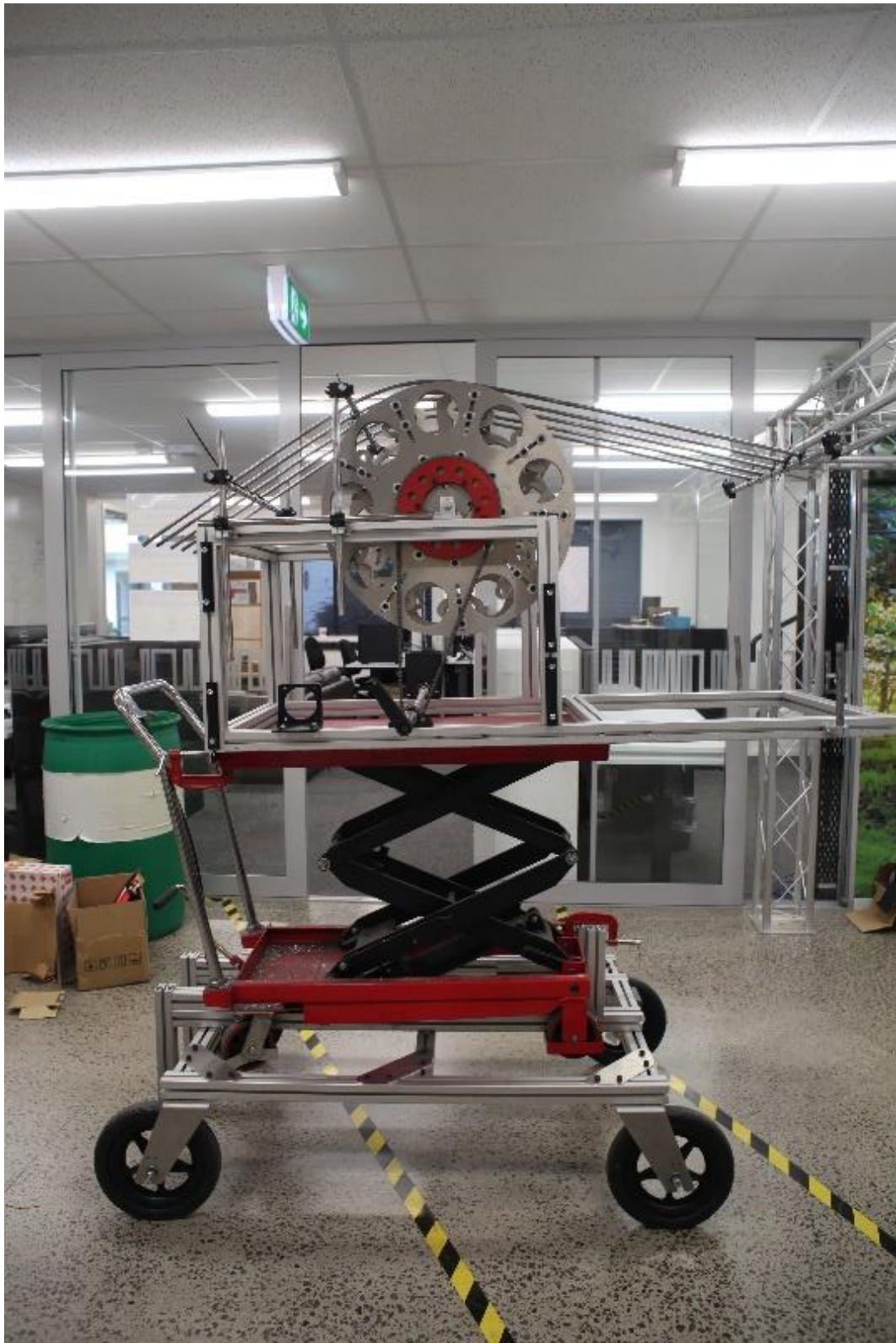
Figure 35: Stem-shear non-selective harvester proof-of-concept prototype
