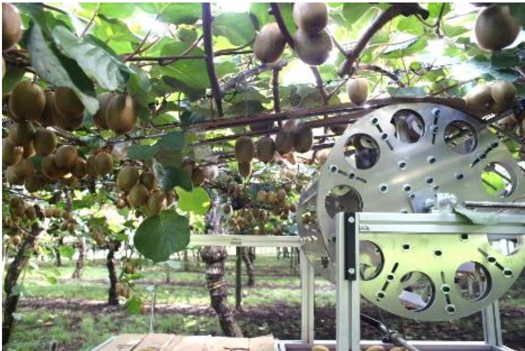
Figure 37: Non-selective harvester preliminary orchard testing
