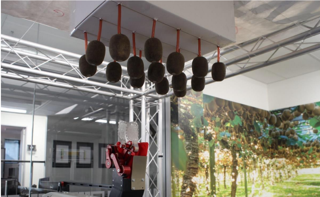
Figure 7: Lab testing with silicone kiwifruit models
