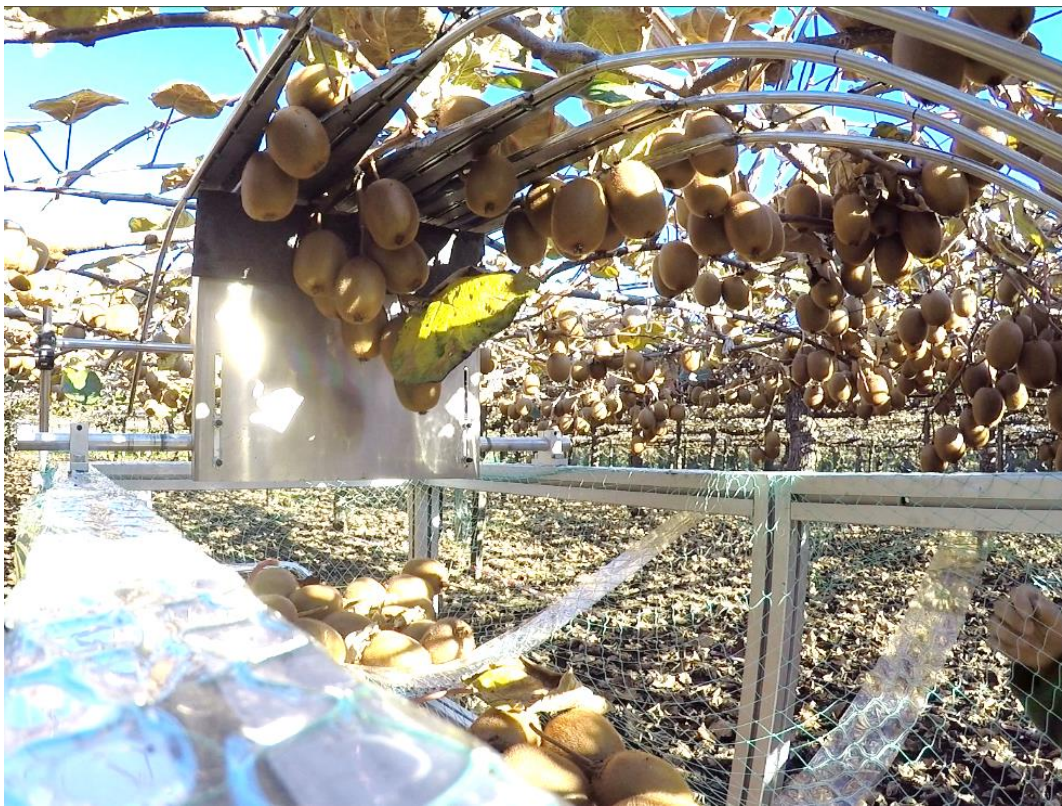
Figure 39: Non-selective harvester combing orchard testing
