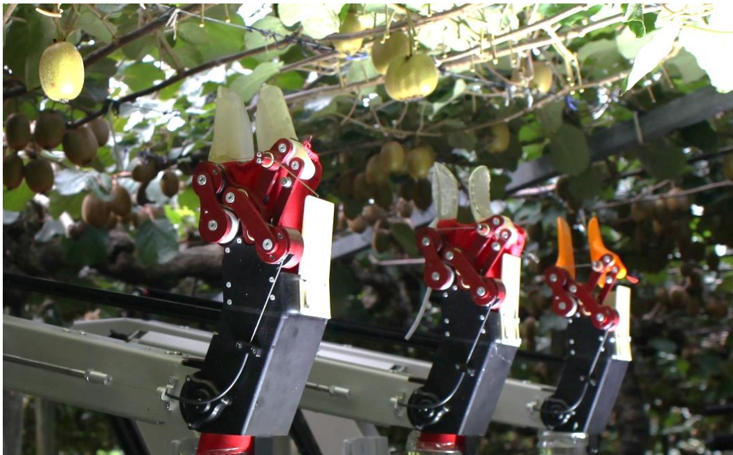
Figure 12: Orchard testing of the grippers
