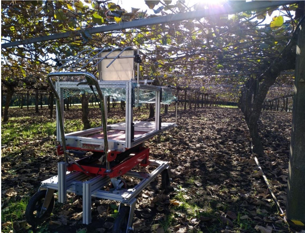
Figure 39: Non-selective harvester combing orchard testing
