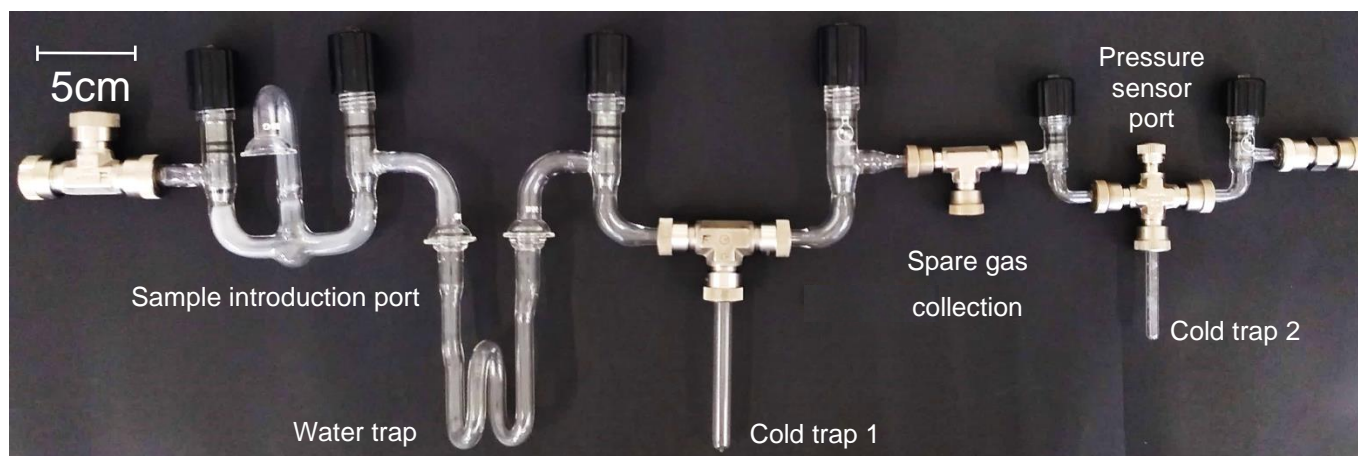
Figure 3.3 Measuring manifold of the current vacuum line used at the WRDL.
