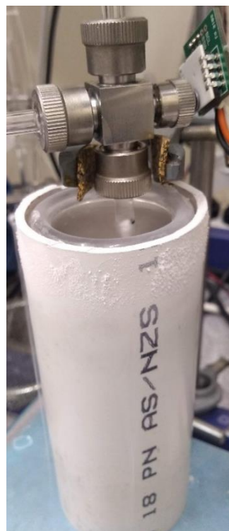
Figure 3.17 Liquid nitrogen is placed around the quartz tube, containing \text{Mg}(\text{ClO}_4)_2 , to freeze \text{CO}_2 into the graphite reactor.
