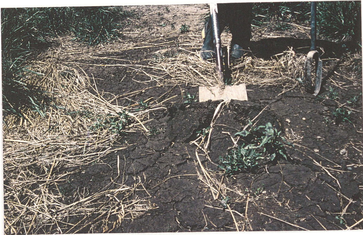
Figure 4.4 Surface crust material at the Kaiapoi site, six months after effluent irrigation had ceased.
