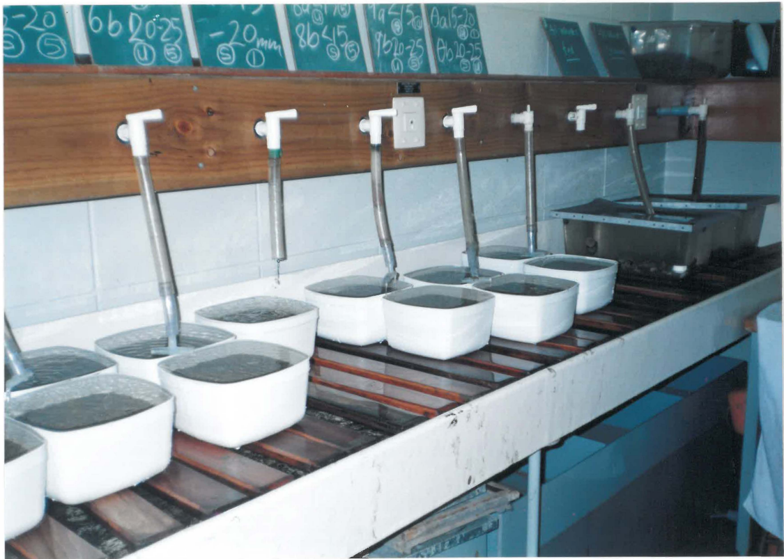
Plate 5.1 Experimental setup for the reburial experiment showing containers and circulation system
