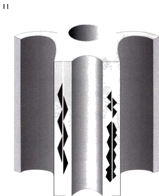
9. Type C1: unusually wide cavities (expansive in tangential plane). 10. Type C2: cavities with diffuse distal edges a tangential plane. 11. Type C4: coalesced V-notched cavitation initiated at ML. 12. Type C5: branched hyphae within V-notched cavity wall (overlying lumen wall is intact).
