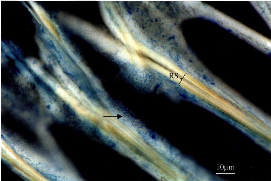
RS = radial section through pine tracheid; arrow = erosion bacterium.
