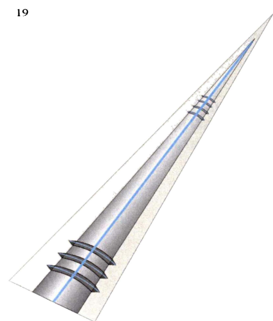
17. Type C7: cavities with serrated edges. 18. Type C7: many merged serrated cavities (easily mistaken for Corbett's Type 2 erosion). 19. Type E1: oblique section through beech fibre with central lumen hyphae and side branches (T-branches?) within troughs. 20. Type E2: Large trough with serrated edges.
