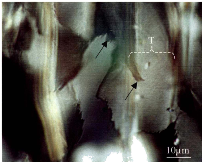
T = width of pine tracheid (earlywood); arrow = fractured cell wall.
