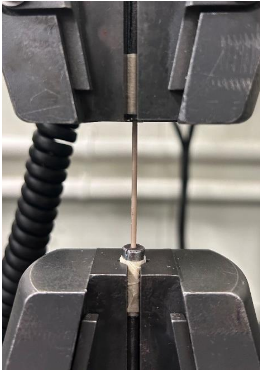
Figure 19: LDPE + 30wt% filament during tensile testing.
