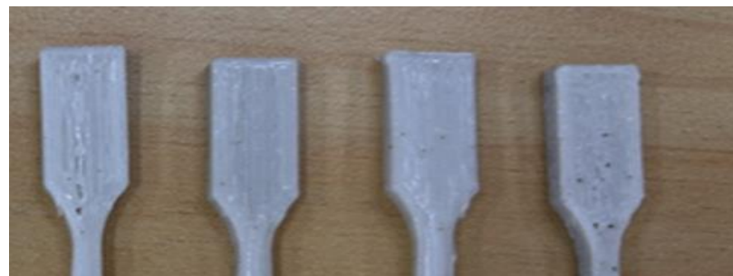
Figure 44: PLA tensile bars a) 0-10wt% bars, b) close view of tensile bars.
