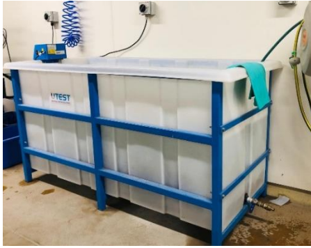
Fig. 14 Water tank used for curing samples at a constant temp.
