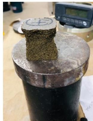
Fig. 23 shear failure for one of the samples.
