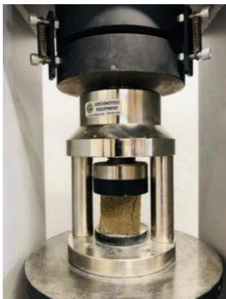
Fig. 22 Test set up for compressive strength of mortar
