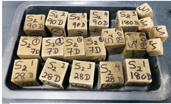
Fig. 13 Samples for curing for 7,28 and 90 days
