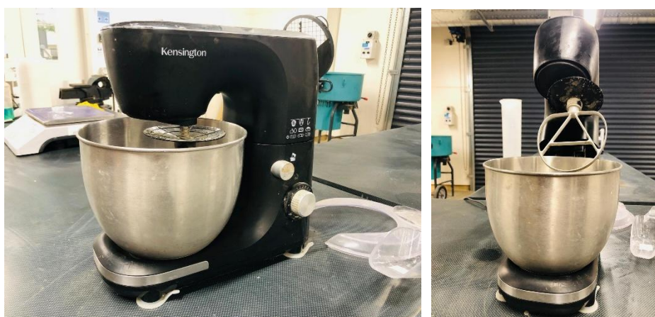
Fig. 11. Kitchen hand mixer used for sample preparation
