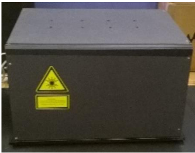
Figure 4.2.1: Light proof optical enclosure.
