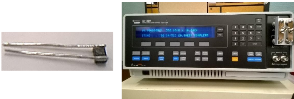
Figure 3.3.1: BRL3225TR51M inductor hardware test.
