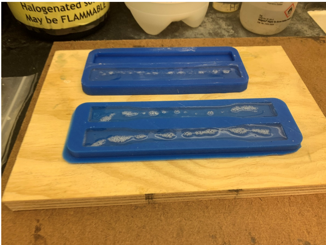
Figure 75: Mold after pouring resin
