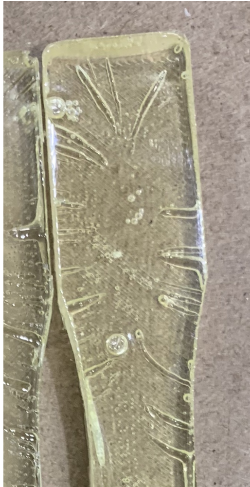
Figure 77: Crack of desired sample
