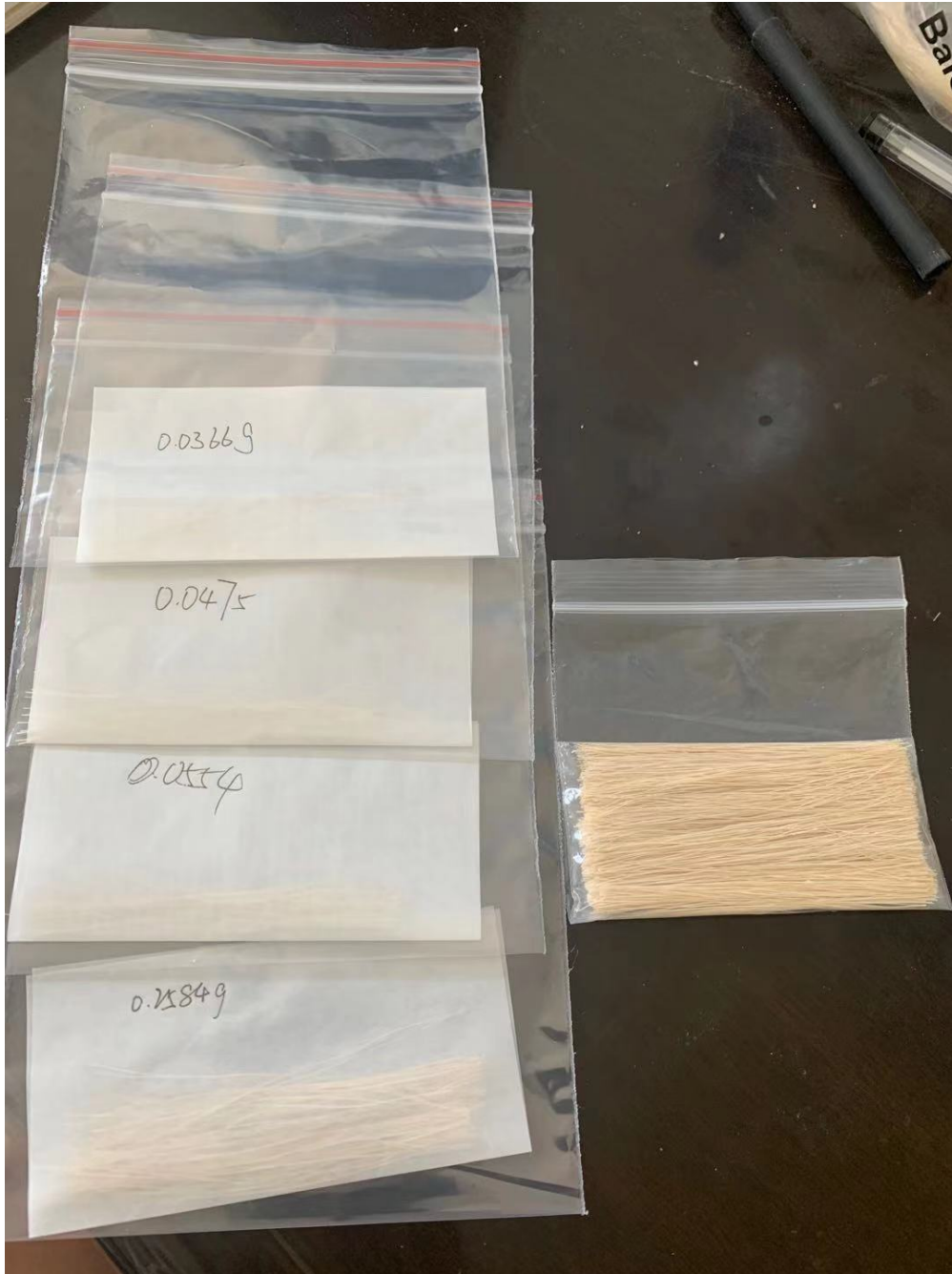
Figure 81: The fiber has been straightened and shaped by the oven
