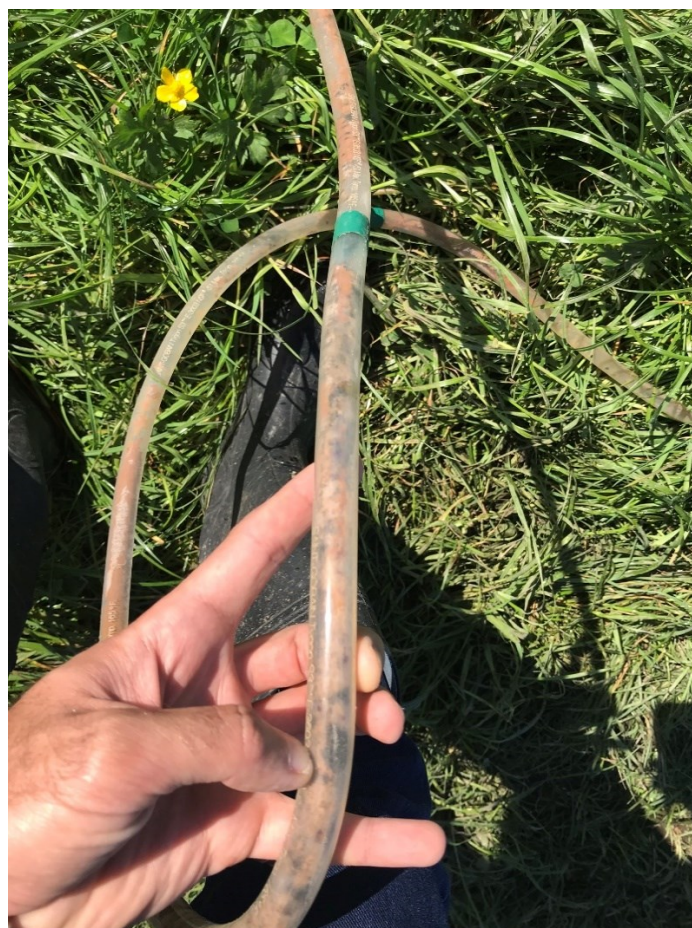
Figure 5.S6: Metal-sulfide precipitates in pump' tubing
