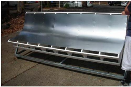
Figure 1: Small parabolic trough reflector (no absorber tube shown)
