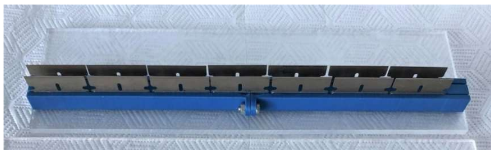
Figure 4: The bespoke gel cutter with replaceable Teflon-coated blades laying on the acrylic chopping board.
