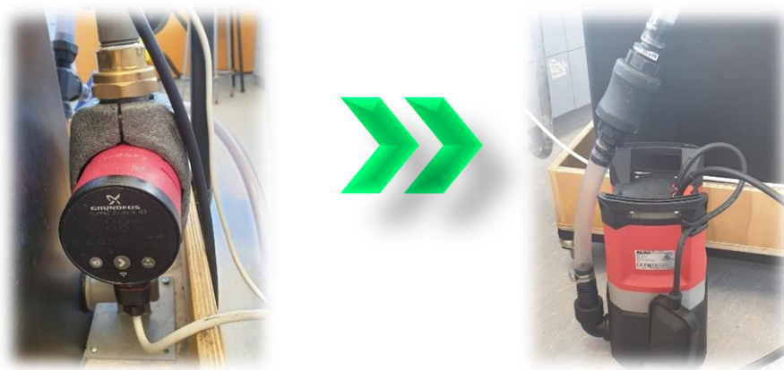
Figure 3.12 Column Modification with Pump
