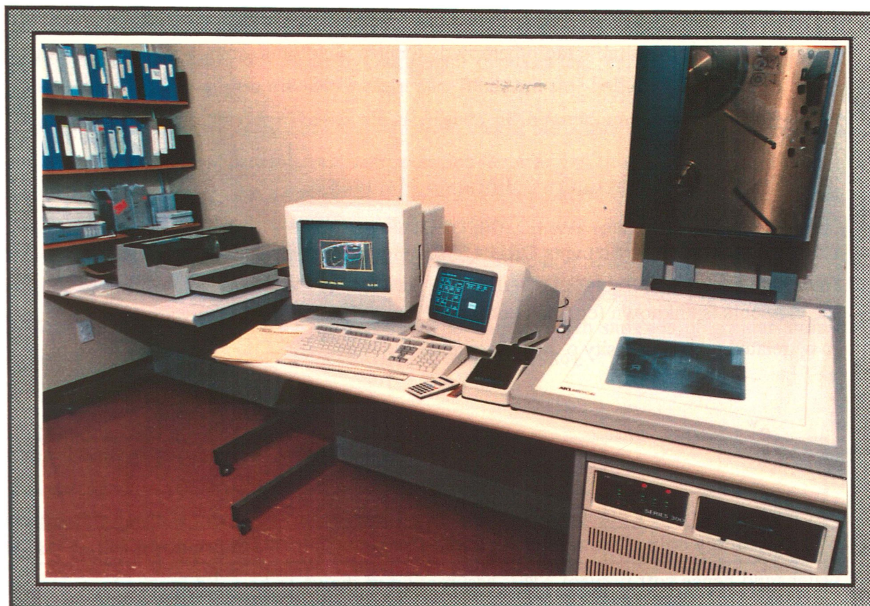
Figure 2.2: Photograph of the Theraplan treatment planning system which was commissioned by the author in 1989 at the Waikato Hospital Radiotherapy Centre.
