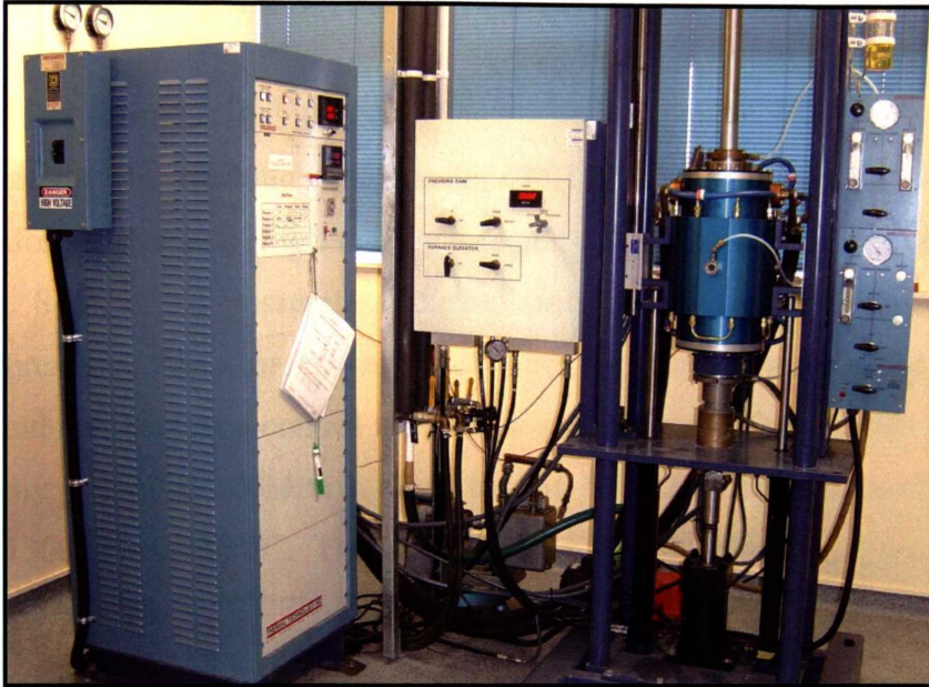
Figure 2.8: Thermal Technology's Group 1400 Laboratory Hot Press
