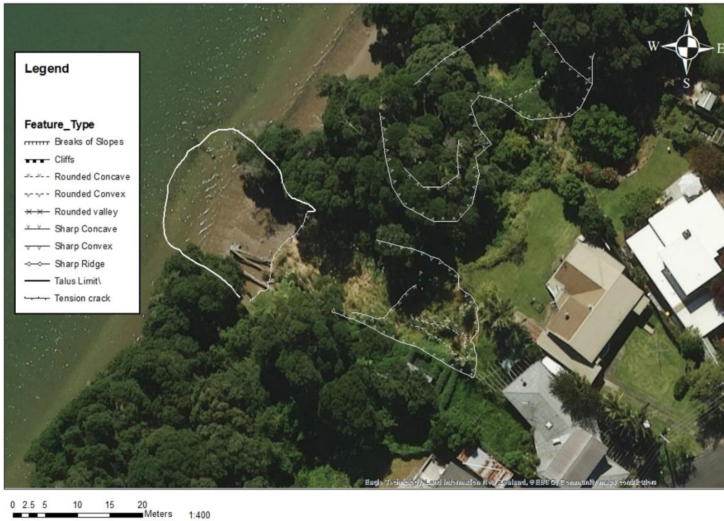
Figure 3.6. An annotated aerial image of the 2017 Kowhai Grove landslide provides a geomorphological context to the landslide. Standard geomorphological ESRI symbols are used and are shown in the legend.
