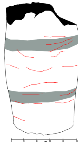
Figure 6.31(a,c) An annotated image of the 12 month treated, 200 kPa, soil cores following failure. Note in this instance barrel failure with a bulging of the material between the two primary shear zones. Some damage to the core has occurred and is shown by the black shaded area. The outline of the features is shown in (c) (b,d) The reverse side of the failed soil core with similar features noted as in (a). Note outlines of the failed core are shown in (d).
