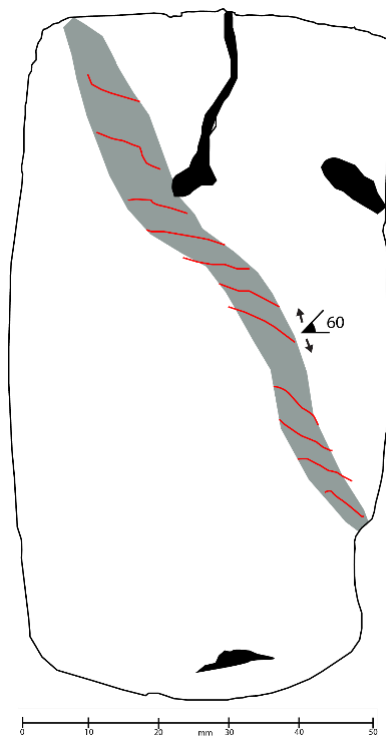
Figure 6.28(a,c) An annotated image of the 200 kPa confining stress, 1 month treated, soil core. A singular primary shear zone is present, with shear seen to occur at an angle of 69°. Minor shears are associated with the primary shear zone. The outline of the shear features are shown in (c). (b,d) The reverse side of the failed 200 kPa, 1 month, core. The primary shear zone has a shallower angle (60°), with some pieces of the sample noted as missing (black zones).
