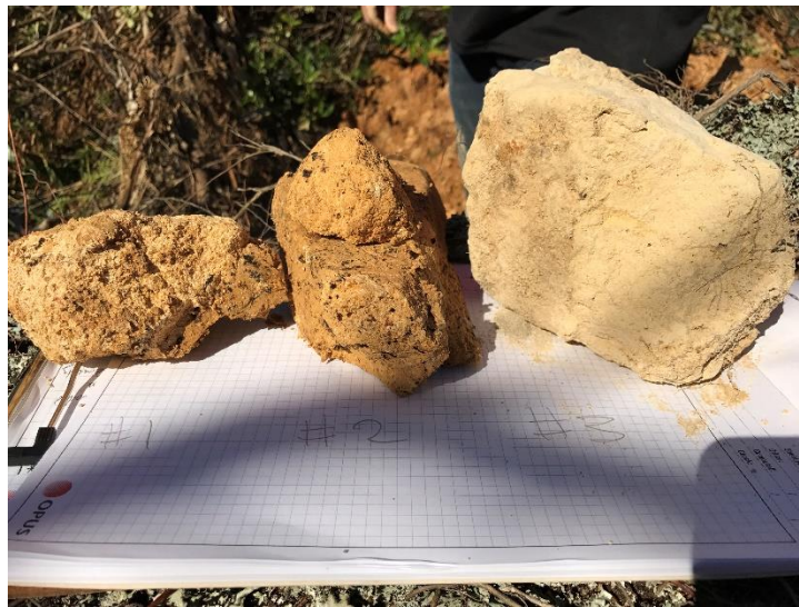
Figure 3.8. Samples of soils found within the Waterview Terrace landslide scarp. From left to right, the soil is representative of Pahoia Tephra, a slightly more weathered Pahoia Tephra, and Te Puna Ignimbrite
