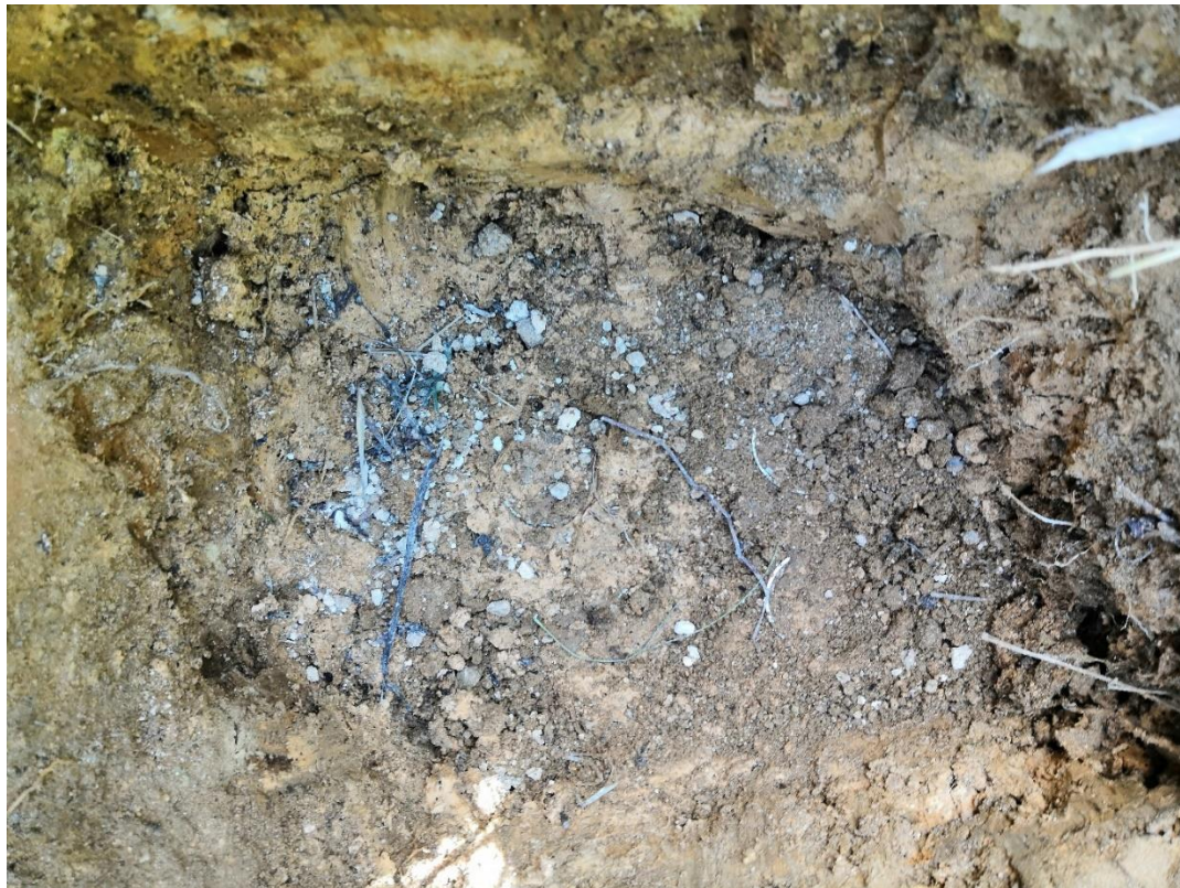
Figure 3.10. An image of a small test pit dug into the Kowhai Grove landslide scarp. Some features of note in this are stark colour change (top right of image) where the soil transitions from the dark brown clayey SILT to an underlying light greyish brown clayey SILT. Sensitive material is hard to distinguish within this image due to the uniformity in which the soil appears. The only visible evidence is the slight smearing of clays between the wall and the base of the test pit, as the pit begins to go into the sensitive layer. Some detritus has fallen into the pit from around the edges.
