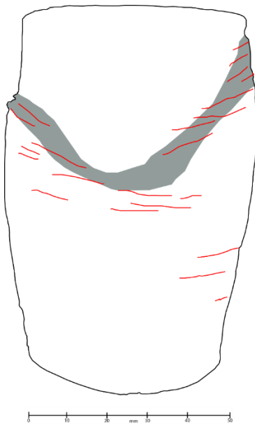
Figure 6.36 (a,c) An annotated image of the wedge style failure observed for the 160 kPa confining stress, 12 month treated soil cores. An outline of shear features is shown in (c). (b) The reverse side of the 160 kPa core, with a 54° angle of failure measured. An outline of shear features is shown in (d).
