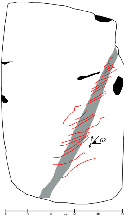
Figure 6.30. (a,c)The annotated image of the 160 kPa, 3 month treated, soil cores. A singular primary shear zone exists with failure occurring at 62°. Minor shears are present along the primary shear zone. The outline of shear features is shown in (c). (b,d) The reverse of the failed core, with the same singular primary shear zone noted, though the angle of failure was slightly shallower (59°). The outline of the image is shown in (d).
