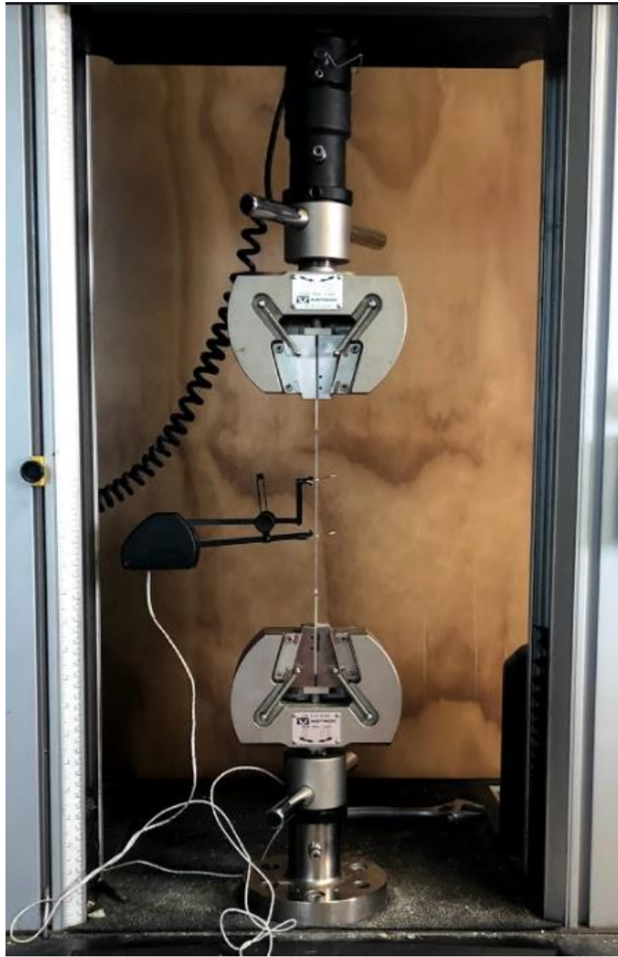
Fig.4 Setup of the tensile coupon tests
