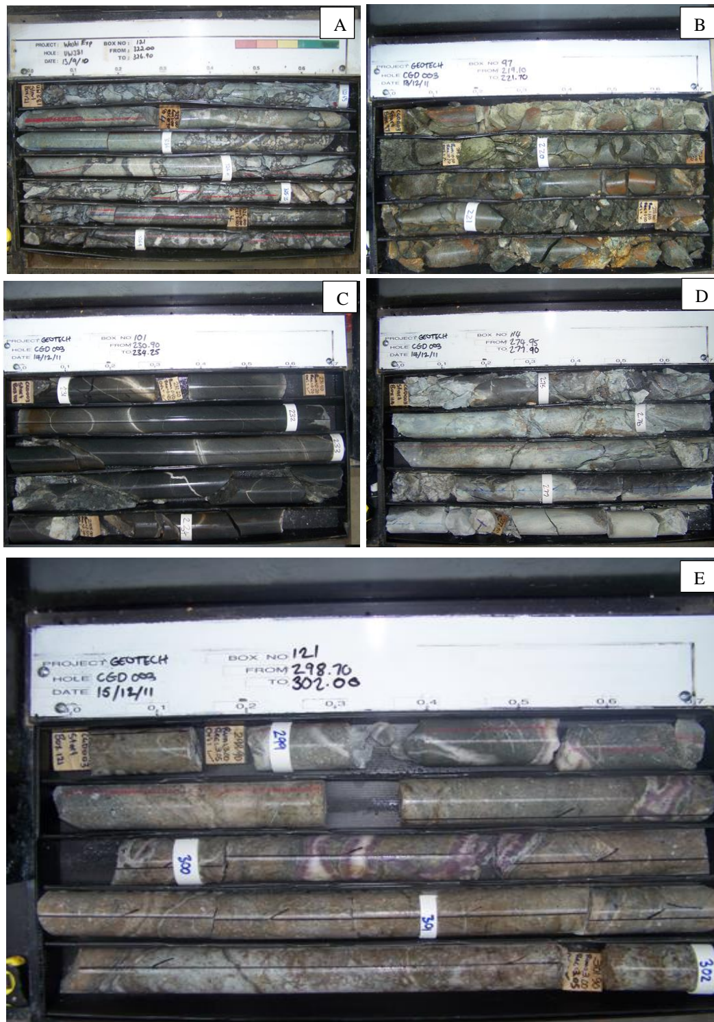
Figure 5.3. (A) Jigsaw shaped hydrothermal breccia at UW381/322m. (B) Propylitic alteration at CGD003/219m. (C) Quartz veins in the hard bar (D) argillic altered andesite at UWCGD003/274.95). (E) Amethyst and quartz veins with breccia clasts at CGD003/298.70.
