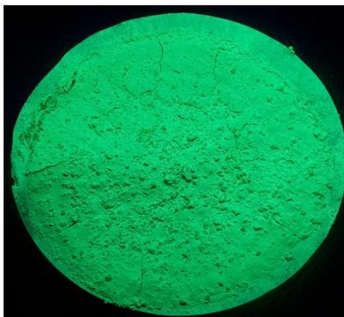
**Figure 1.20:** Znq<sub>2</sub> under UV excitation.
