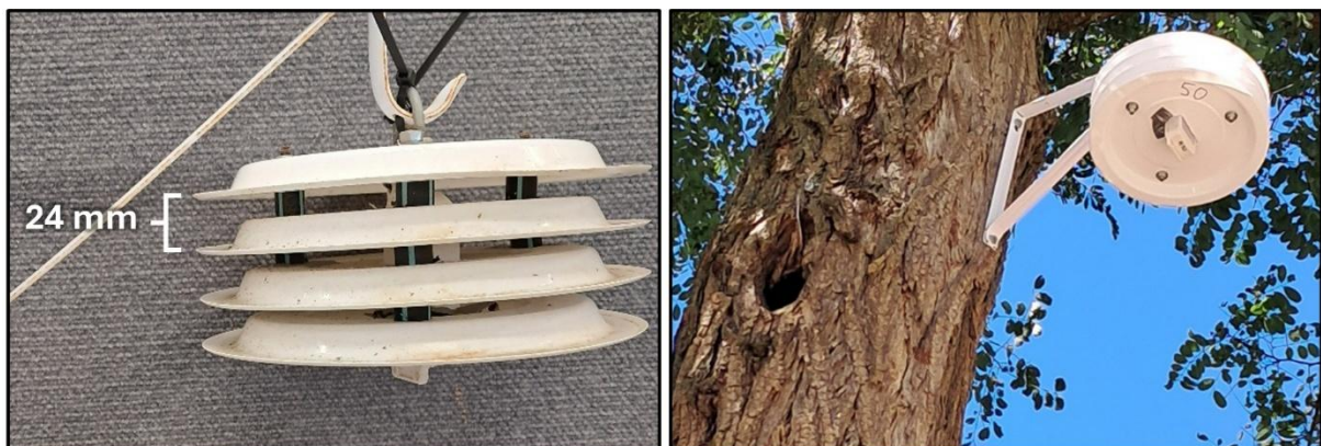
Figure 2.4 Ambient microclimate dataloggers within solar radiation shields. Image on right shows one installed next to Natural Roost 1.
