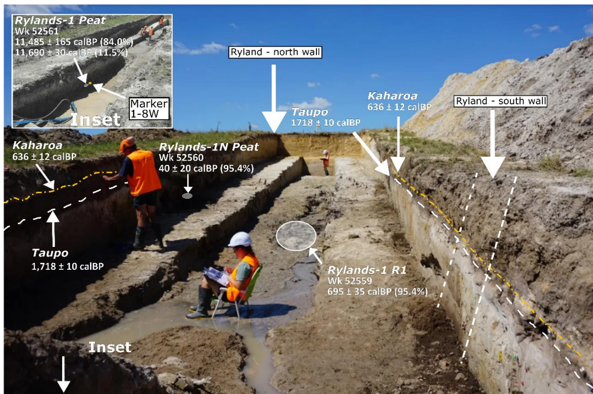
Figure 3.4: Synthesis of radiocarbon dates of wood and peat, and (tephrochronological) dates of visible tephra layers, observed in the Arnold trench. Photo: D.J. Lowe.
