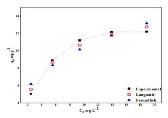
Figure 4-17: The fitting of the non-linear adsorption models to the experimental data for  $Cu^{2+}$  adsorption on the CH/cHAp composites
