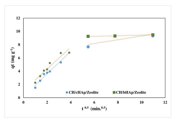
Figure 4-134: The fitting of the intra-particle diffusion model (IPD) to the experimental data for  $Cu^{2+}$  adsorption on the CH/HAp/zeolite composites
