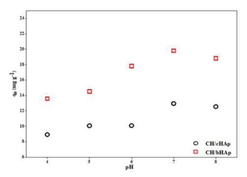
Figure 4-5: AAS data showing the effect of initial solution pH on  $Cd^{2+}$  adsorption on the CH/HAp composites. Results are reported as the average of 3 replicates.  $SE=\pm0.01$
