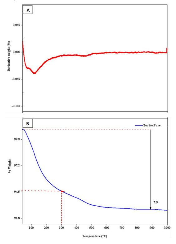
Figure 2-31: Thermograms of mordenite used in this study (A) DTG Curve (B) Thermogram
