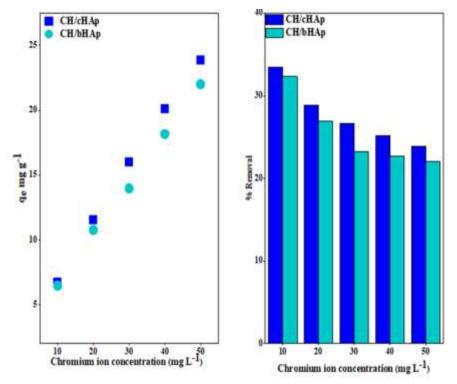
Figure 4-12: AAS data showing the effect of initial metal ion concentration on chromate ion adsorption on the CH/HAp composites. Results are calculated as an average of 3 replicates.  $SE = \pm 0.1$ .
