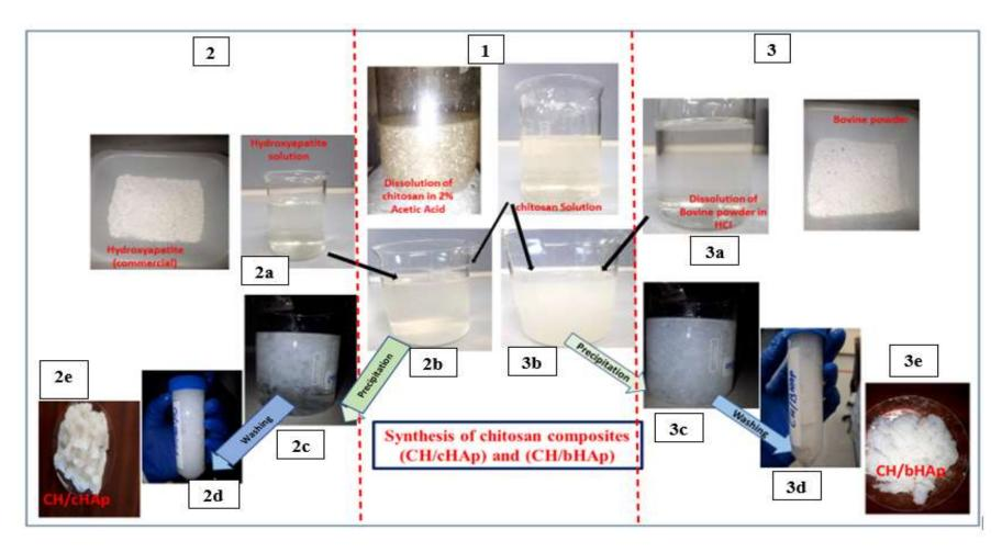
Figure 3-2: The synthesis of the CH/HAp composites
