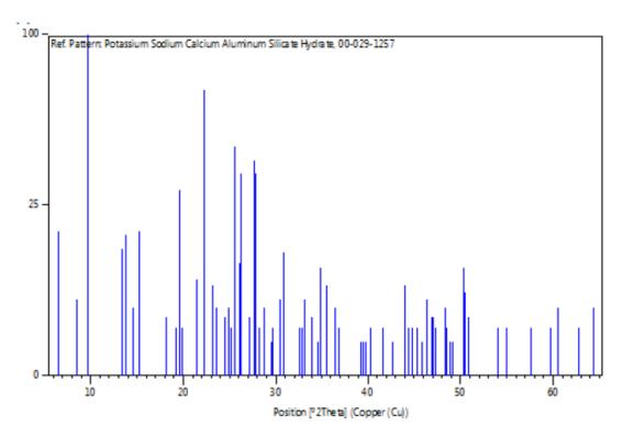
Figure 2-30: The reference diffraction pattern of mordenite (ICDD: 00-029-1257)
