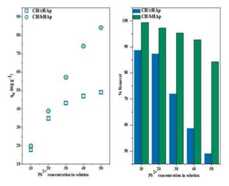
Figure 4-10: AAS data showing the effect of initial metal ion concentration on Pb<sup>2+</sup> adsorption on the CH/HAp composites. Results are calculated as an average of 3 replicates.  $SE = \pm 0.1$ .
