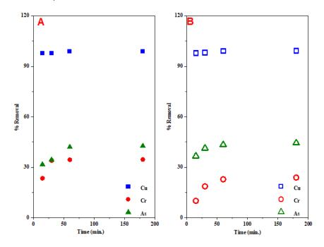
Figure 6-4: ICP-MS data showing the removal of Cu<sup>2+</sup>, chromate ion and arsenate ion from an industrial input stream solution sample by the CH/HAp/CF composites for a 0.1 g dose of (A) CH/cHAp/CF and (B) CH/bHAp/CF (Contact time data).
