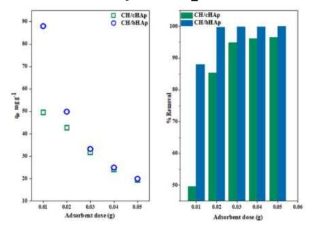
Figure 4-2: AAS results showing the effect of adsorbent dose on  $Pb^{2+}$  ion removal and adsorption of  $Pb^{2+}$  ion on the CH/HAp composites: Results are presented as the average of measurements from 3 replicates.  $SE = \pm 0.1$
