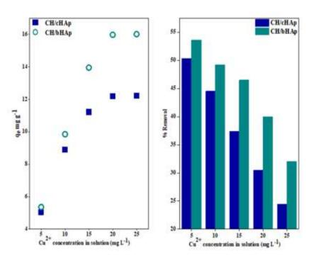
Figure 4-11: AAS data showing the effect of initial metal ion concentration on  $Cu^{2+}$  adsorption on the CH/HAp composites. Results are calculated as an average of 3 replicates. SE =  $\pm$  0.1.
