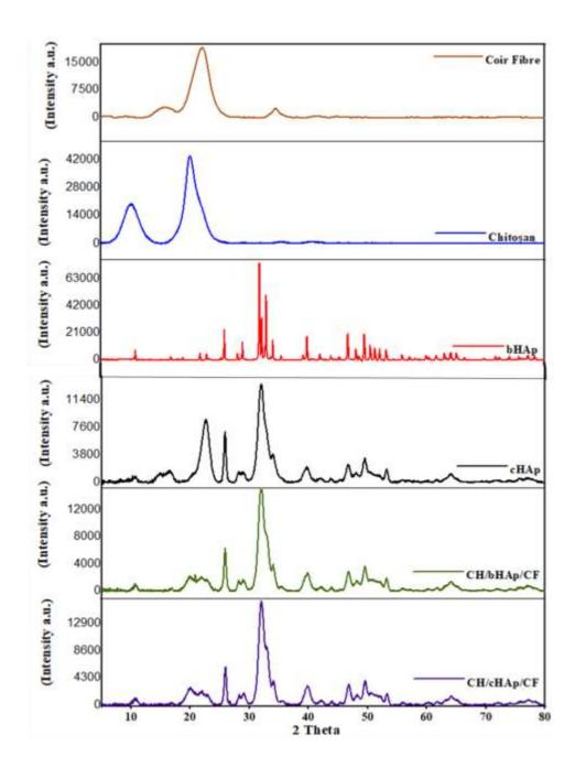
Figure 3-17: The X-ray diffractograms of CH/cHAp/CF and CH/bHAp/CF and the raw candidate materials of the composites
