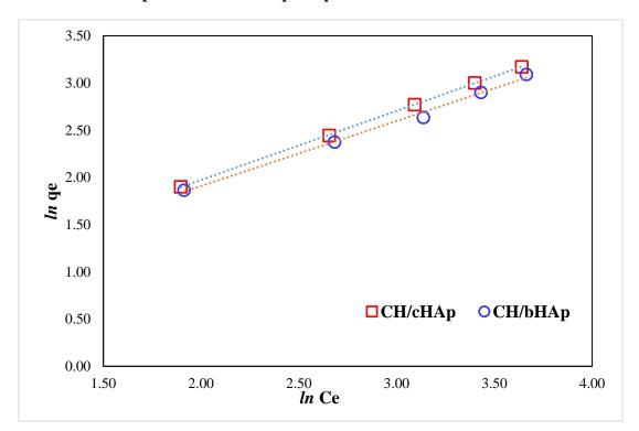
Figure 4-20: The fitting of the linearized Freundlich isotherm model to the experimental data for chromate ion adsorption on the CH/HAp composites.
