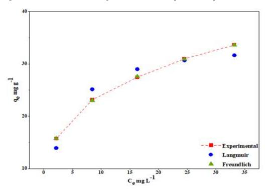
Figure 4-79: The fitting of non-linear Langmuir and Freundlich adsorption isotherms to experimental data for Pb<sup>2+</sup> adsorption on the CH/cHAp/SCGs composite
