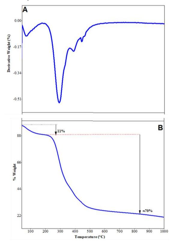
Figure 2-25: Thermograms of spent coffee grounds (SCGs) (A) DTG Curve (B) Thermogram  $\,$
