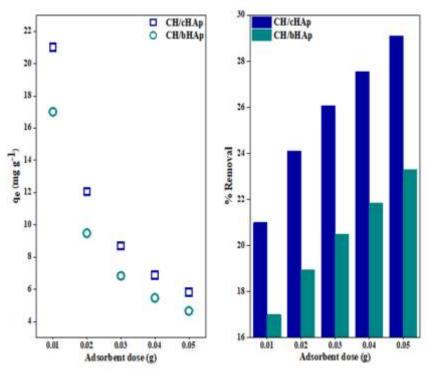
Figure 4-4: AAS results showing the effect of adsorbent dose on chromate ion removal and adsorption of chromate ion on the CH/HAp composites: Results are presented as the average of measurements from 3 replicates.  $SE = \pm 0.1$
