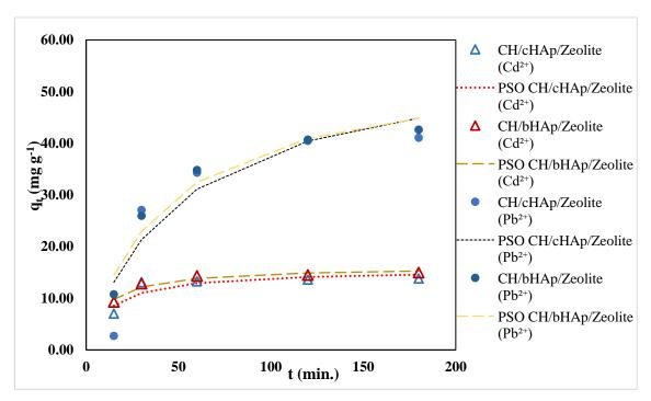
Figure 5-23: relating to  $Cd^{2+}$  and  $Pb^{2+}$  competitive adsorption on the CH/HAp/zeolite composites for an adsorbent dose of 0.01 g
