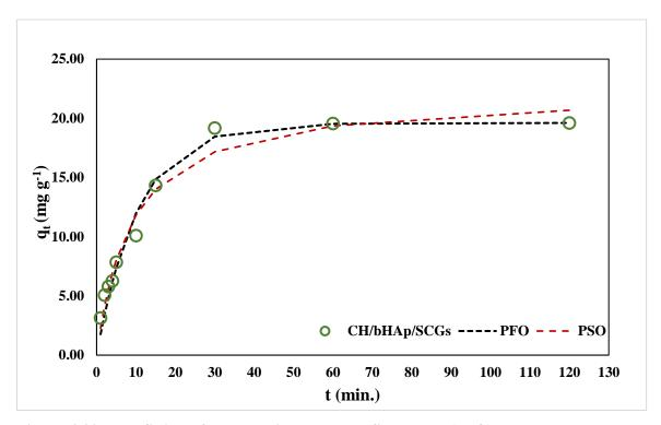
Figure 4-92: The fitting of the non-linear pseudo-first-order (PFO) and pseudo-second-order (PSO) kinetics models to the experimental data for  $Pb^{2+}$  adsorption on the CH/bHAp/SCGs composites
