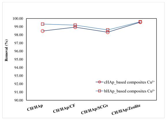
Figure 5-4: Comparison of the removal efficiencies of the synthesised composites for the removal of  $Cu^{2+}$  ions from an industrial input stream sample using 0.1 g of adsorbent
