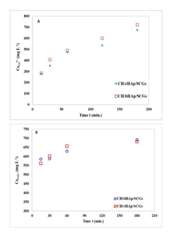
Figure 6-11: The concentration of  $Ca^{2+}$  ions analysed by ICP-MS in an industrial input stream solution during its exposure to (A) 0.01 g and (B) 0.1 g doses of the CH/HAp/SCGs composites
