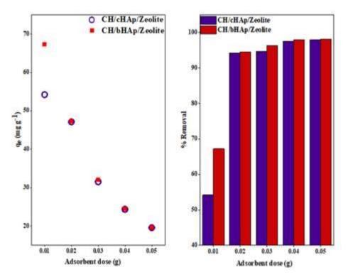
Figure 4-98: AAS data showing the effect of adsorbent dose on  $Pb^{2+}$  removal and adsorption on the CH/HAp/zeolite composites: The results are presented as the average of measurements of three replicates.  $SE = \pm 0.4$
