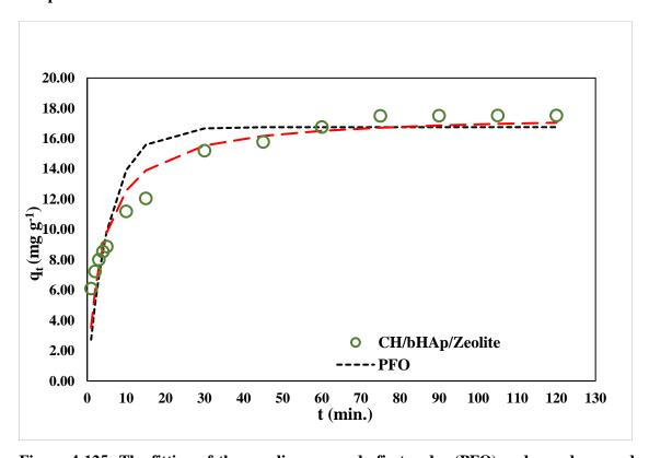
Figure 4-125: The fitting of the non-linear pseudo-first-order (PFO) and pseudo-second-order (PSO) kinetic models to the experimental data for  $Cd^{2+}$  adsorption on the CH/bHAp/zeolite composites
