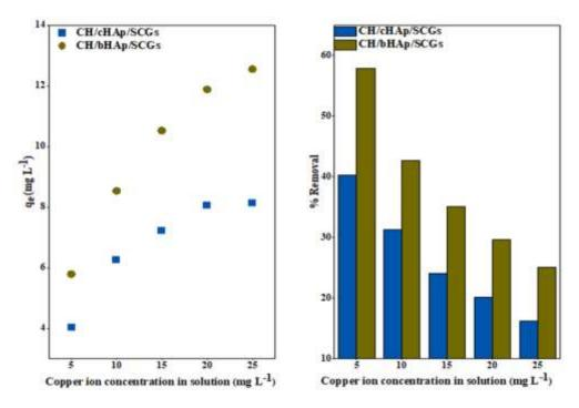
Figure 4-75 AAS data showing the effect of initial metal ion concentration on  $Cu^{2+}$  removal and adsorption on the CH/HAp/SCGs composites. The results are presented as the average of measurements of three replicates. SE =  $\pm$  0.3
