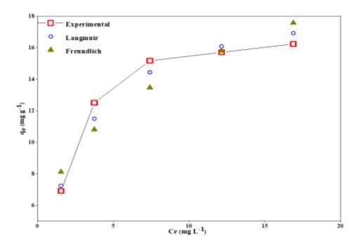
Figure 4-45: The fitting of non-linear Langmuir and Freundlich isotherm models to experimental data for Cd<sup>2+</sup> adsorption on the CH/cHAp/CF composite.
