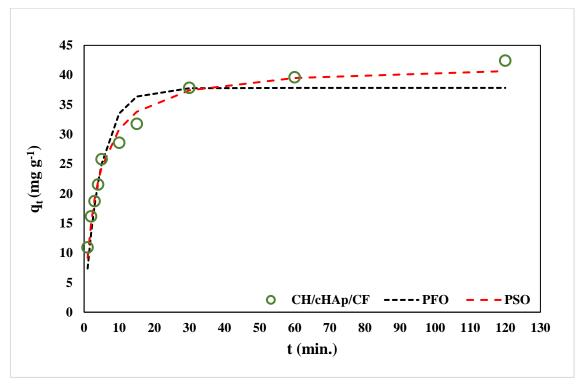
Figure 4-59: The fitting of the non-linear pseudo-first-order and pseudo-second-order kinetics models to contact time data for Pb<sup>2+</sup> adsorption on the CH/cHAp/CF composite
