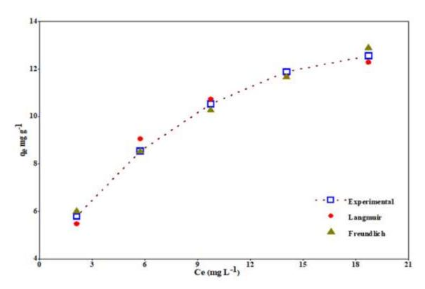
Figure 4-82: The fitted non-linear Langmuir and Freundlich isotherms for  $Cu^{2+}$  adsorption on the CH/bHAp/SCGs composite
