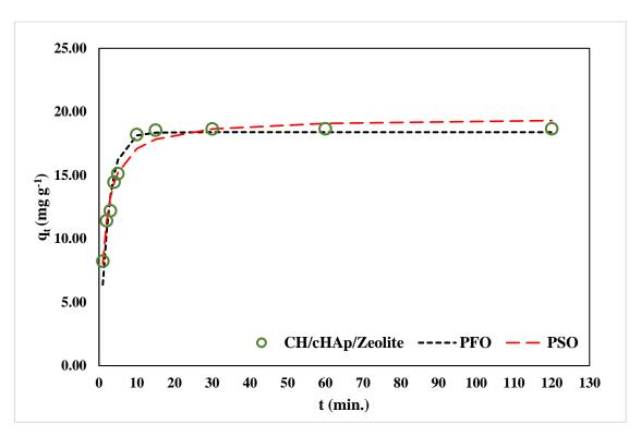
Figure 4-126: The fitting of the non-linear pseudo-first-order (PFO) and pseudo-second-order (PSO) kinetic models to the experimental data for  $Pb^{2+}$  adsorption on the CH/cHAp/zeolite composites
