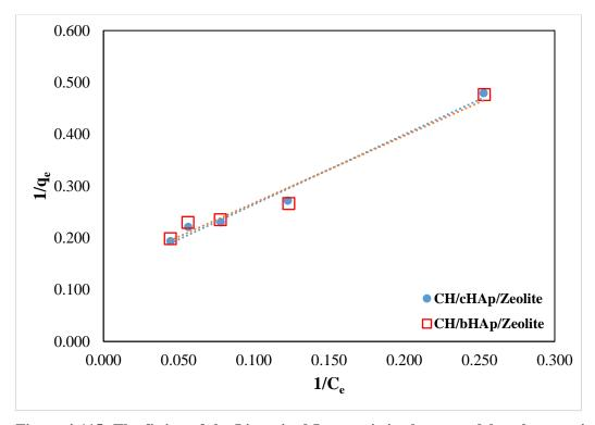
Figure 4-115: The fitting of the Linearized Langmuir isotherm model to the experimental data for chromate ion adsorption on the CH/HAp/zeolite composites
