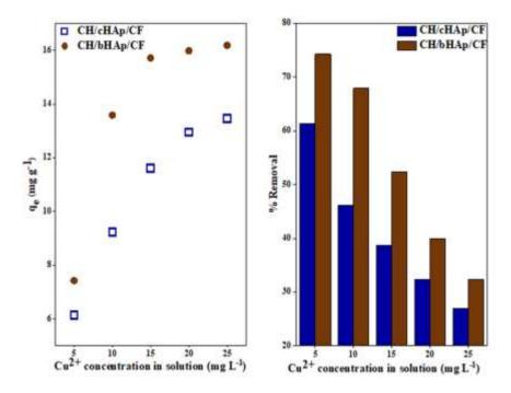
Figure 4-43: AAS data showing the effect of initial metal ion concentration on  $Cu^{2+}$  removal and adsorption on the CH/HAp/CF composites. The results are presented as the average of measurements of three replicates.  $SE = \pm 0.1$
