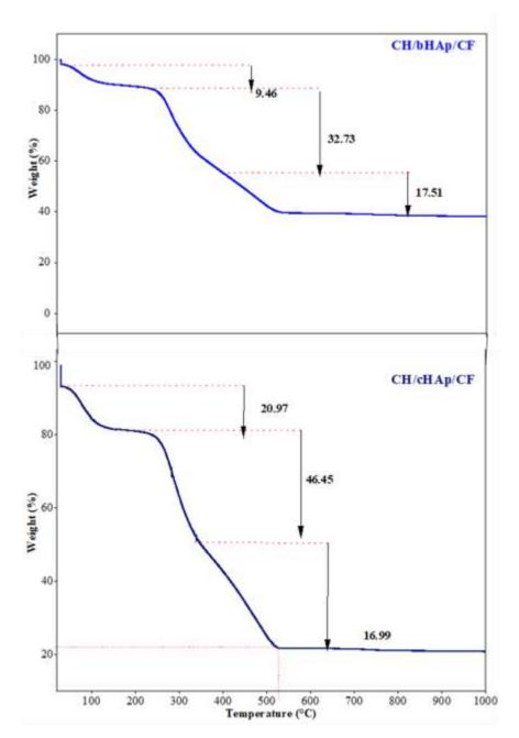
Figure 3-18: Thermograms of the CH/cHAp/CF and CH/bHAp/CF composites
