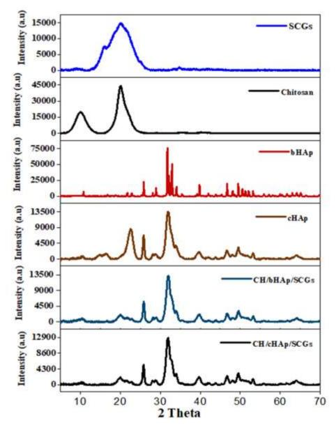
Figure 3-22: X-ray diffractograms of the CH/cHAp/SCGs and CH/bHAp/SCGs composites
