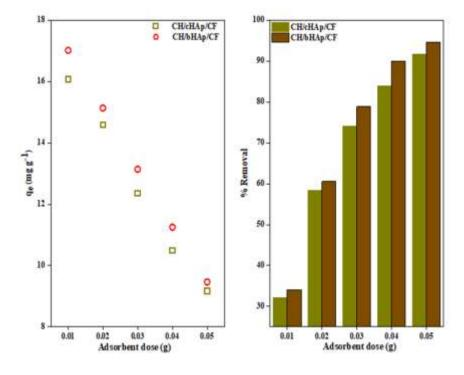
Figure 4-33: AAS data showing the effect of adsorbent dose on  $Cd^{2+}$  ion removal and adsorption of  $Cd^{2+}$  ion on CH/HAp/CF composites: Results are presented as the average of measurements from 3 replicates. SE =  $\pm$  0.1
