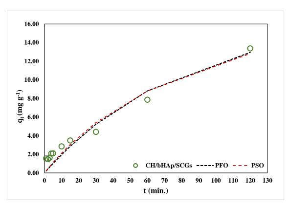
Figure 4-94: The fitting of the non-linear pseudo-first-order and pseudo-second-order kinetics models to experimental data for Cu<sup>2+</sup> adsorption on the CH/bHAp/SCGs composite
