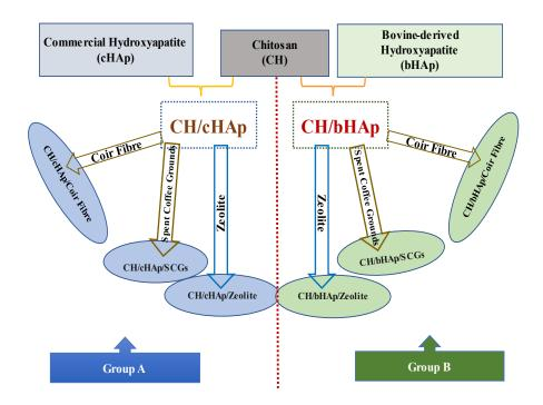
Figure 3-1: Schematic diagram showing the composite matrices synthesised in this study
