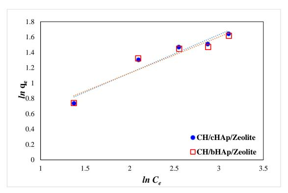
Figure 4-116: The fitting of the Linearized Freundlich isotherm model to the experimental data for chromate ion adsorption on the CH/HAp/zeolite composites
