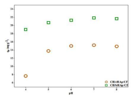
Figure 4-37: AAS data showing the effect of solution pH on  $Cd^{2+}$  removal and adsorption on the CH/HAp/CF composites. The results are presented as the average of measurements of three replicates.  $SE = \pm 0.1$
