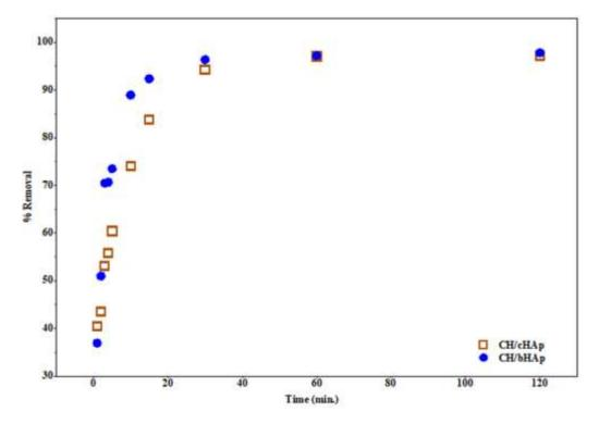
Figure 4-22: AAS data showing the effect of contact time on Pb<sup>2+</sup> adsorption on the CH/HAp composites. Results are reported as the average of 3 replicates.  $SE = \pm 0.1$ .
