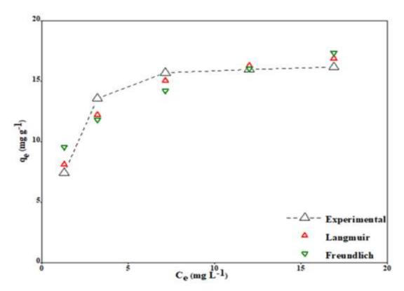
Figure 4-50: The fitting of the non-linear Langmuir and Freundlich isotherms to data for  $Cu^{2+}$  adsorption on the CH/bHAp/CF composite.
