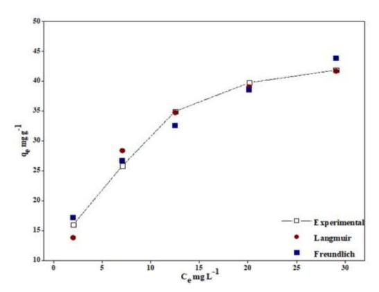
Figure 4-80: The fitting of the non-linear Langmuir and Freundlich adsorption isotherms to experimental data for Pb<sup>2+</sup> adsorption on the CH/bHAp/SCGs composite
