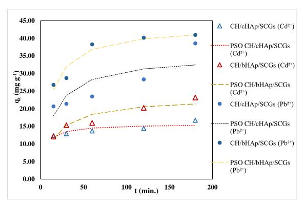
Figure 5-17: The fitting of the non-linear pseudo-second-order kinetic model to experimental (contact time) data relating to  $Cd^{2+}$  and  $Pb^{2+}$  competitive adsorption on the CH/HAp/SCGs composites for an adsorbent dose of 0.01 g
