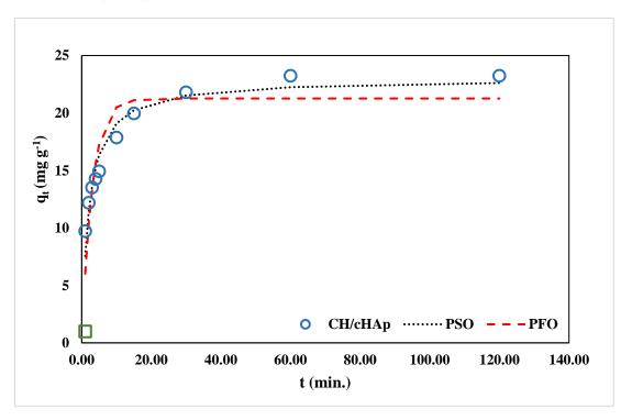
Figure 4-31: The fitting of the non-linear PFO and PSO kinetic models to the experimental contact time data for chromate ion adsorption on the CH/cHAp composites
