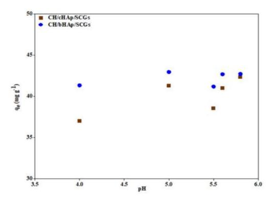
Figure 4-70: AAS data showing the effect of solution pH on  $Pb^{2+}$  adsorption on the CH/HAp/SCGs composites. The results are presented as the average of measurements of three replicates.  $SE = \pm 0.2$
