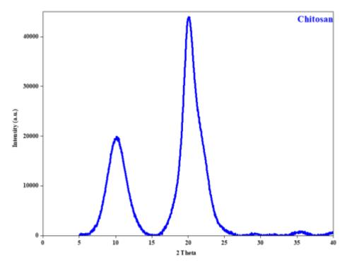
Figure 2-6: X-ray diffractogram of powdered TCI chitosan used in this study
