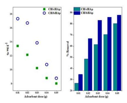
Figure 4-3: AAS results showing the effect of adsorbent dose on  $Cu^{2+}$  ion removal and adsorption of  $Cu^{2+}$  ion on the CH/HAp composites: Results are presented as the average of measurements from 3 replicates.  $SE = \pm 0.1$
