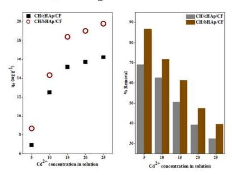
Figure 4-41: AAS data showing the effect of initial metal ion concentration on  $Cd^{2+}$  adsorption on CH/HAp/CF composites. Results are calculated as an average of 3 replicates.  $SE = \pm 0.1$ .
