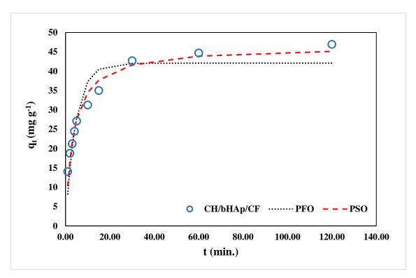
Figure 4-60: The fitting of the pseudo-first-order and pseudo-second-order kinetics models to contact time data for Pb<sup>2+</sup> adsorption on the CH/bHAp/CF composite
