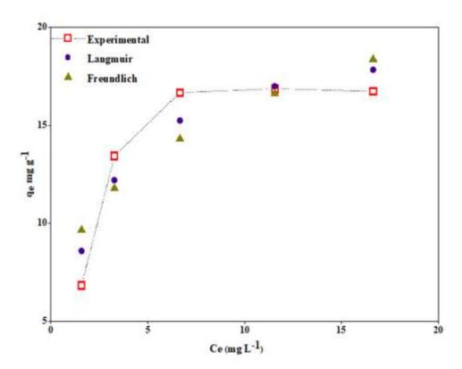
Figure 4-114: The fitting of the non-linear Langmuir and Freundlich isotherms to data for  $Cu^{2+}$  adsorption on the CH/bHAp/zeolite composite
