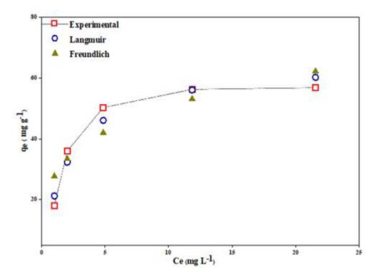
Figure 4-47: The fitting of non-linear Langmuir and Freundlich adsorption isotherms to experimental data for Pb<sup>2+</sup> adsorption on the CH/cHAp/CF composite
