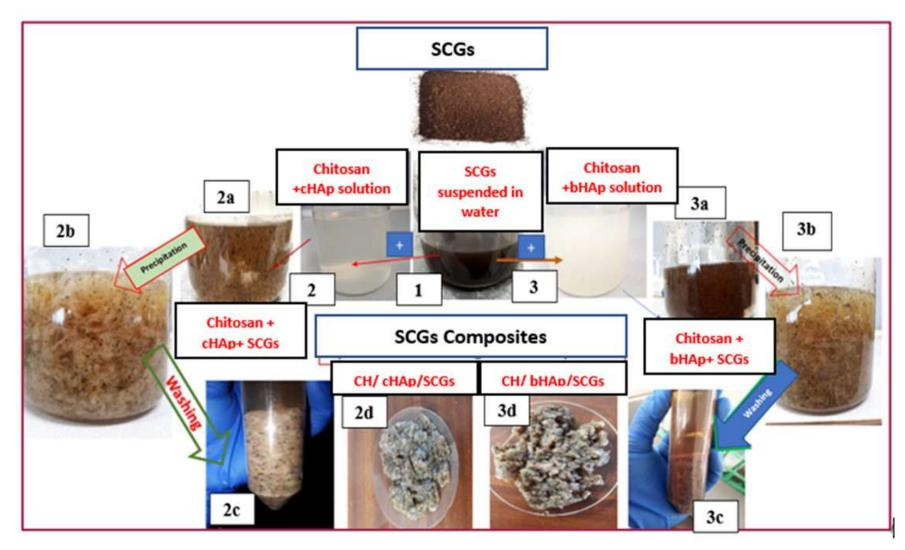
Figure 3-4: The synthesis of the CH/HAp/SCGs composites
