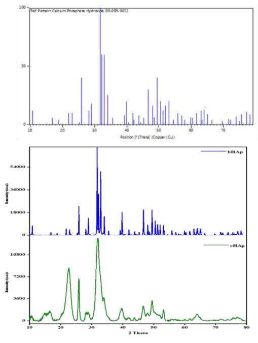
Figure 2-14: The reference diffraction pattern of stoichiometric hydroxyapatite ((ICDD no. 09-0432), and the diffractograms of bHAp and cHAp
