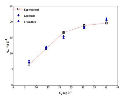
Figure 4-109: The fitting of the non-linear Langmuir and Freundlich adsorption isotherms to experimental data for  $Cd^{2+}$  adsorption on the CH/cHAp/zeolite composite
