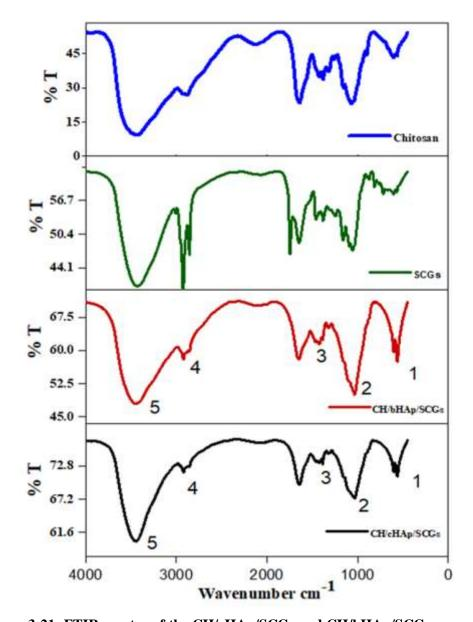
Figure 3-21: FTIR spectra of the CH/cHAp/SCGs and CH/bHAp/SCGs composites as well as those of the raw chitosan and SCGs materials
