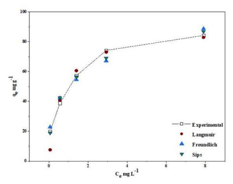
Figure 4-16: The fitting of various non-linear adsorption models to experimental data for  $Pb^{2+}$  adsorption on the CH/bHAp composites
