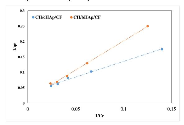
Figure 4-51: Fitting of the Linearized Langmuir isotherm model to the experimental data for chromate ion adsorption on the CH/HAp/CF composites
