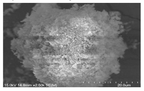
Figure 2-26: SEM micrograph of zeolite (mordenite)
