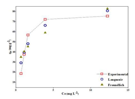
Figure 4-48: The fitting of non-linear Langmuir and Freundlich adsorption isotherms to experimental data for Pb<sup>2+</sup> adsorption on the CH/bHAp/CF composite.
