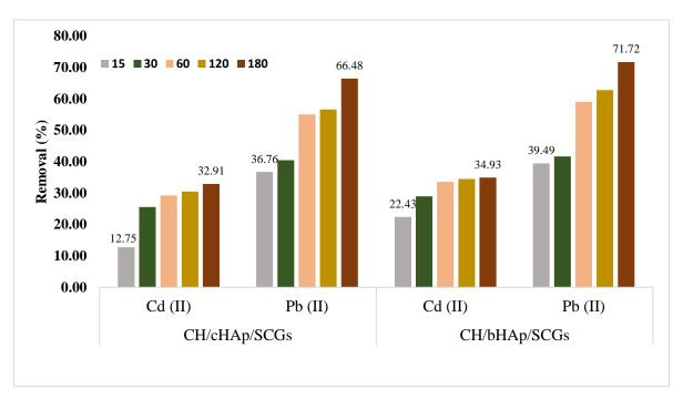
Figure 5-13: Graph showing the competitive removal (%) of Cd<sup>2+</sup> and Pb<sup>2+</sup> ions by 0.01 g doses of the CH/HAp/SCGs composites at contact times ranging from 15 minutes to 180 minutes.
