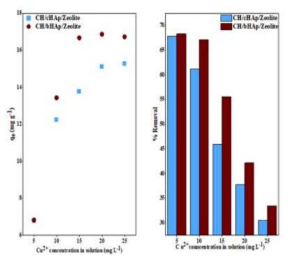
Figure 4-107: AAS data showing the effect of initial metal ion concentration on  $Cu^{2+}$  removal and adsorption on the CH/HAp/zeolite composites. The results are presented as the average of measurements of three replicates. SE =  $\pm$  0.3
