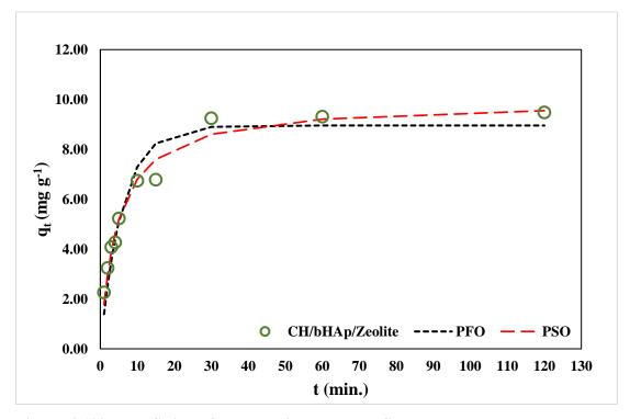
Figure 4-129: The fitting of the non-linear pseudo-first-order and pseudo-second-order kinetics models to experimental data for  $Cu^{2+}$  adsorption on the CH/bHAp/zeolite composite
