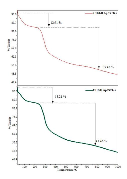
Figure 3-23: Thermograms of CH/cHAp/SCGs and CH/bHAp/SCGs
