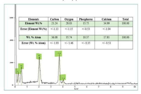
Figure 3-7: EDX analysis of the CH/cHAp composite
