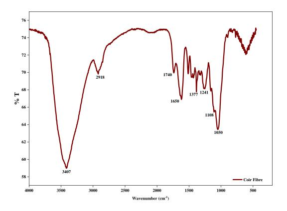
Figure 2-18: FTIR spectrum of coir fibre
