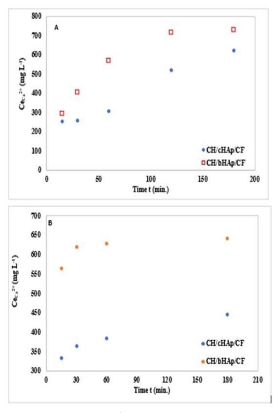
Figure 6-10: The concentration of  $Ca^{2+}$  ions analysed by ICP-MS in an industrial input stream during its exposure to (A) 0.01 g and (B) 0.1 g doses of the CH/HAp/CF composites
