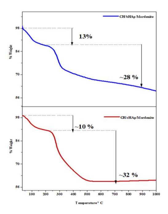
Figure 3-28: Thermograms of the CH/cHAp/Zeolite and CH/bHAp/Zeolite composites
