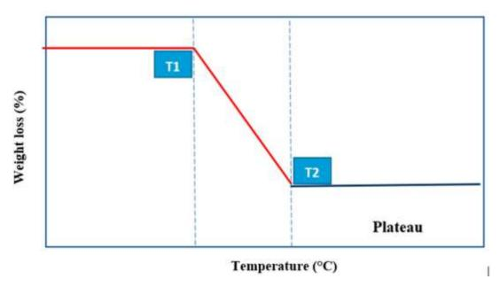
Figure 2-1: A typical thermogram with a single weight-loss event
