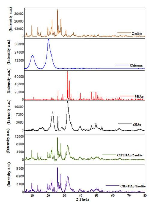
Figure 3-27: X-ray diffraction patterns of the CH/cHAp/Zeolite and CH/bHAp/Zeolite composites as well as those of the raw materials.
