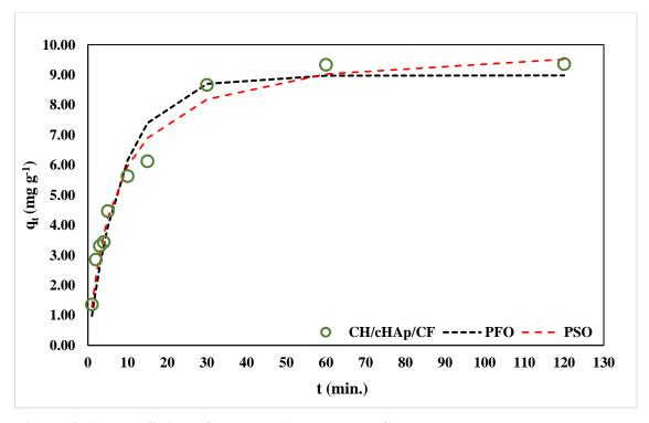
Figure 4-61: The fitting of the non-linear pseudo-first-order and pseudo-second-order kinetics models to contact experimental time data for  $Cu^{2+}$  adsorption on the CH/cHAp/CF composite
