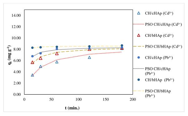
Figure 5-6: The fitting of the PSO kinetic model to the experimental contact time data for the CH/HAp composites exposed to solutions containing both  $Cd^{2+}$  and  $Pb^{2+}$  for an adsorbent dose of 0.05 g
