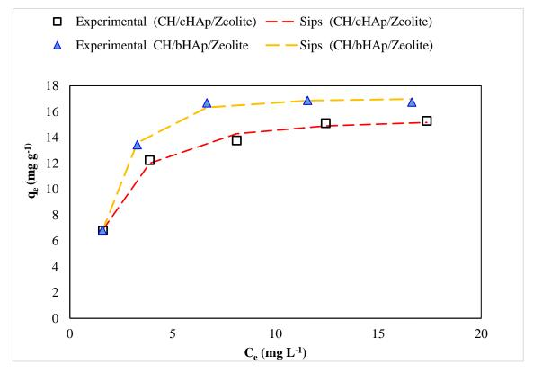
Figure 4-119: The fitting of the Sips isotherm model to the experimental data for  $Cu^{2+}$  ion adsorption on the CH/HAp/zeolite composite
