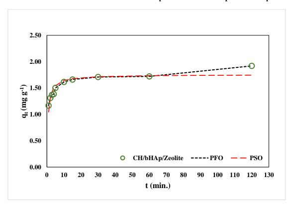
Figure 4-131: The fitting of the pseudo-first-order and pseudo-second-order kinetics model to the data for chromate ion adsorption on the CH/bHAp/zeolite composites
