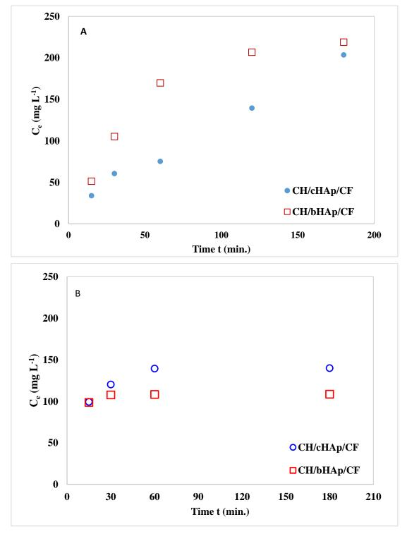
Figure 6-14: The concentration of phosphorus as analysed using ICP-MS in the industrial input stream solution exposed to the CH/HAp/CF composites at (A) 0.01 g, (B) 0.1 g of adsorbent doses
