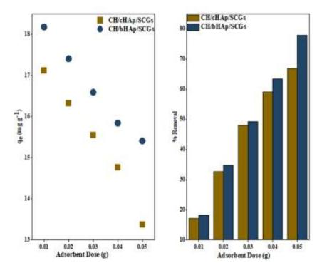
Figure 4-65: AAS data showing the effect of adsorbent dose on  $Cd^{2+}$  ion removal and adsorption of cadmium ion on the CH/HAp/SCGs composites: Results are presented as the average of measurements from 3 replicates.  $SE = \pm 0$ .
