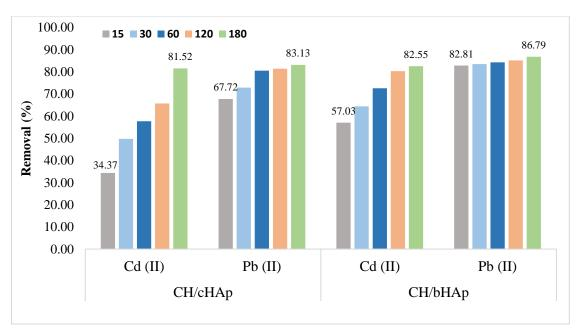
Figure 5-2: The competitive adsorption of Cd<sup>2+</sup> and Pb<sup>2+</sup> shown as removal (%) values at 0.01 g of the CH/HAp composites during contact times ranging from 15 minutes to 180 minutes.
