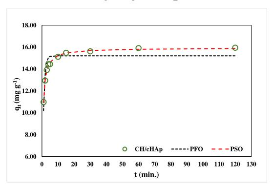
Figure 4-25: The fitting of the non-linear pseudo-first-order (PFO) and pseudo-second-order (PSO) kinetic models to the contact time experimental data for  $Cd^{2+}$  adsorption on the CH/cHAp composite
