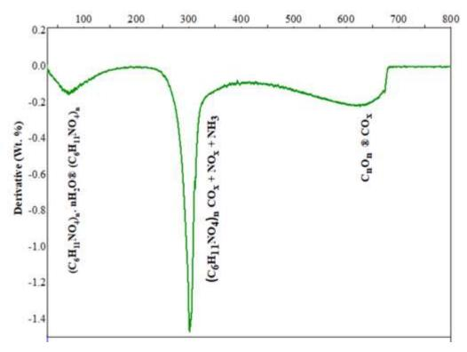
Figure 2-7: Thermogram of chitosan used in this study (Derivative % weight loss curve)
