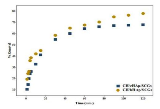
Figure 4-85: AAS data showing the effect of contact time on  $Cd^{2+}$  removal (%) by the CH/HAp /SCGs composites. The results are presented as the average of measurements of three replicates.  $SE = \pm 0.1$
