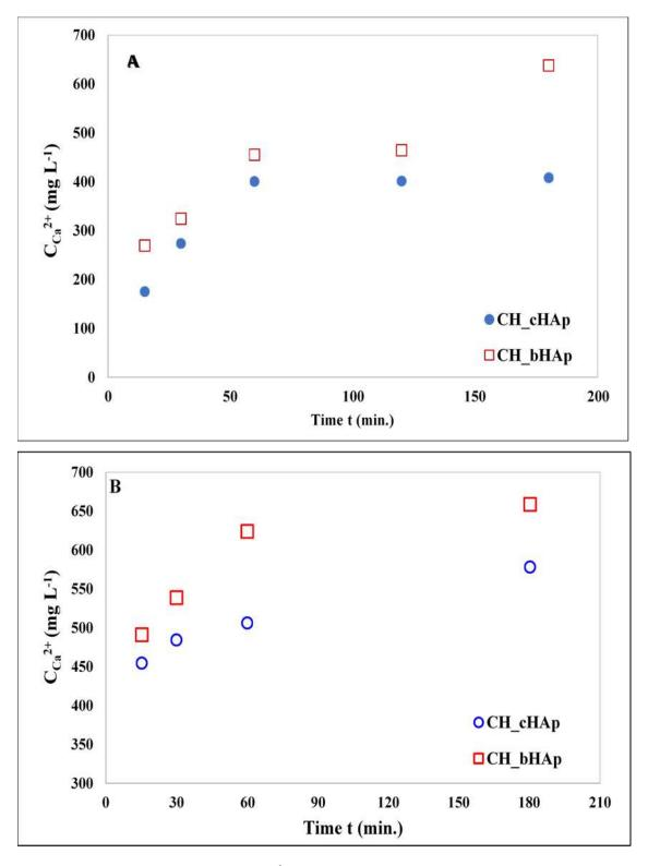
Figure 6-9: The concentration of  $Ca^{2+}$  ions analysed by ICP-MS in an industrial input stream sample during its exposure to (A) 0.01 g and (B) 0.1 g of the CH/HAp composites
