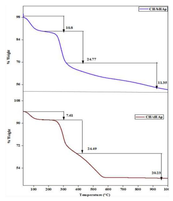
Figure 3-13: Thermograms of the CH/cHAp and CH/bHAp composites
