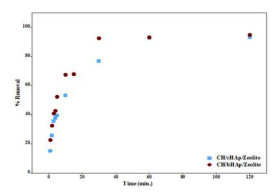
Figure 4-122: AAS data showing the effect of contact time on  $Cu^{2+}$  removal by the CH/HAp/zeolite composites. The results are presented as the average of measurements of three replicates.  $SE=\pm 0.1$
