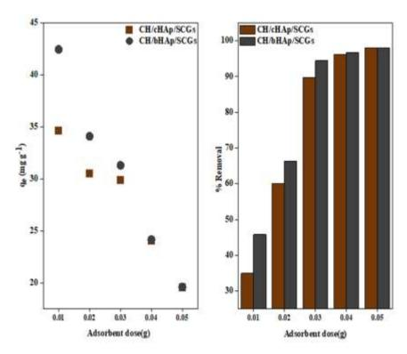
Figure 4-66: AAS data showing the effect of adsorbent dose on  $Pb^{2+}$  removal and adsorption on the CH/HAp/SCGs composites. The results are presented as the average of measurements of three replicates.  $SE = \pm 0.2$
