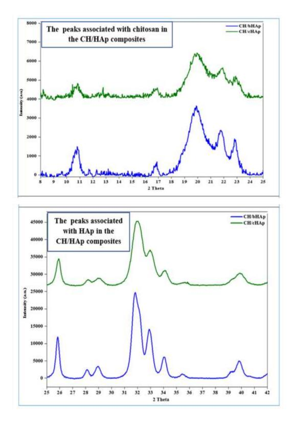
Figure 3-12: The characteristic diffraction peaks of chitosan and HAp recorded in the CH/HAp composites and presented as a detailed view
