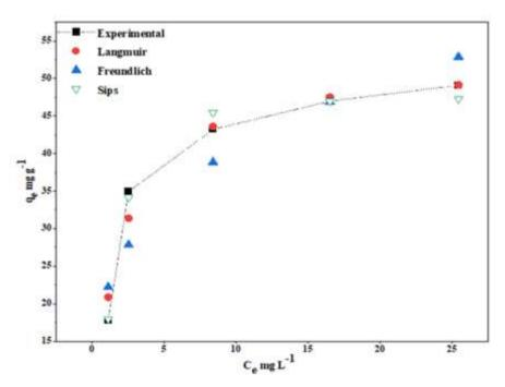
Figure 4-15: The fitting of various non-linear adsorption models to experimental data for  $Pb^{2+}$  adsorption on the CH/cHAp composites
