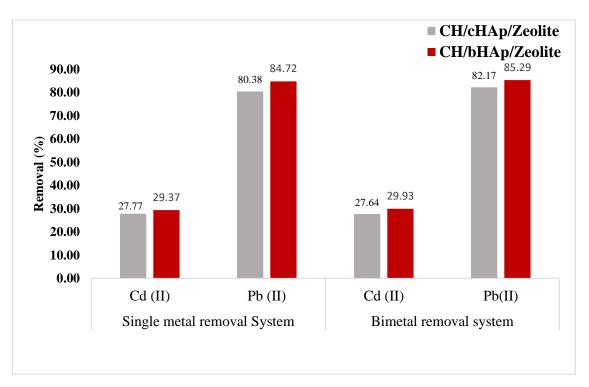
Figure 5-21: The comparison of the single and two-metal ion types removal systems for Cd<sup>2+</sup> and Pb<sup>2+</sup> ions adsorption on 0.01 g of adsorbent dose of CH/HAp/zeolite composites
