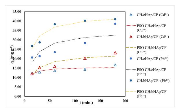
Figure 5-11: The fitting of the non-linear pseudo-second-order kinetic model to experimental (contact time) data relating to  $Cd^{2+}$  and  $Pb^{2+}$  competitive adsorption on the CH/HAp/CF composites for an adsorbent dose of 0.01 g
