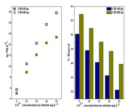
Figure 4-9: AAS data showing the effect of initial metal ion concentration on  $Cd^{2+}$  adsorption on the CH/HAp composites. Results are calculated as an average of 3 replicates.  $SE = \pm 0.1$ .
