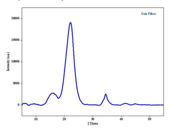
Figure 2-19: X-ray diffractogram of coir fibre
