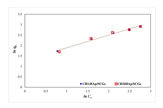
Figure 4-84: The fitting of the linearized Freundlich isotherm model to the experimental data for chromate ion adsorption on the CH/HAp/SCGs composites
