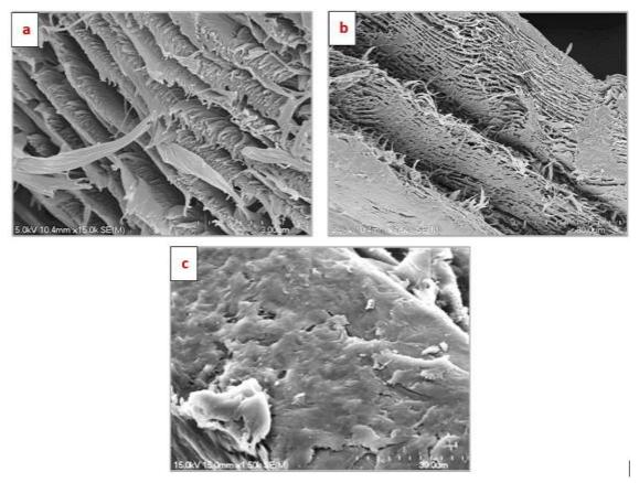
Figure 2-2: SEM micrographs of commercial chitosan 5.0 kV (a & b), 15 kV (c) used in the present study
