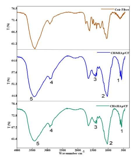
Figure 3-16: FTIR spectra of coir fibre (dust), CH/cHAp/CF and CH/bHAp/CF composites
