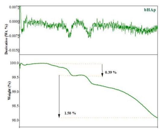
Figure 2-16: Thermograms of bHAp and corresponding DTG curves
