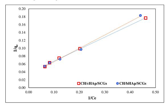
Figure 4-83: The fitting of the linearized Langmuir isotherm model to the experimental data for chromate ion adsorption on the CH/HAp/SCGs composites
