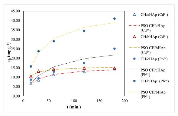
Figure 5-5: The fitting of the pseudo-second-order kinetic model to experimental (contact time) data relating to  $Cd^{2+}$  and  $Pb^{2+}$  competitive adsorption on the CH/HAp composites on an adsorbent dose of 0.01 g.
