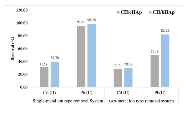
Figure 5-3: Comparison of removal data for Cd<sup>2+</sup> and Pb<sup>2+</sup> ions by a 0.01 g adsorbent dose of the CH/HAp composites from solutions containing either one or two metal ion types.
