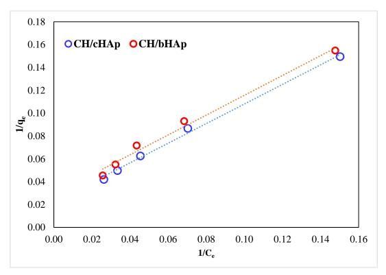
Figure 4-19: Fitting of the linearized Langmuir isotherm model to the experimental data for chromate ion adsorption on the CH/HAp composites
