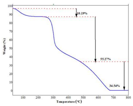
Figure 2-8: Thermogram of chitosan used in this study (Thermal degradation curve)
