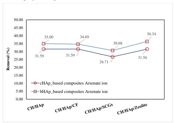
Figure 5-7: Comparison of the removal efficiencies of the synthesised composites for the removal of arsenate ions from the industrial input stream sample using 0.01 g of adsorbent dose
