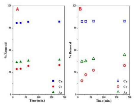
Figure 6-2: Simultaneous removal of  $Cu^{2+}$ , arsenate ion and chromate ion by the CH/HAp composites using 0.1 g adsorbent doses of (A) CH/cHAp composite and (B) CH/bHAp composites
