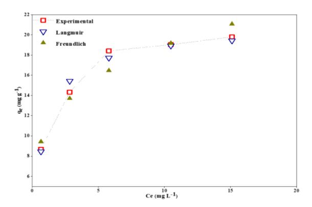
Figure 4-46: The fitting of non-linear Langmuir and Freundlich isotherm models to experimental data for Cd<sup>2+</sup> adsorption on the CH/bHAp/CF composite.
