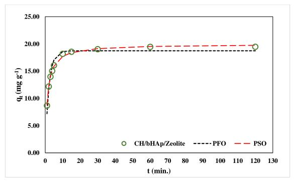
Figure 4-127: The fitting of the non-linear pseudo-first-order (PFO) and pseudo-second-order (PSO) kinetic models to the experimental data for  $Pb^{2+}$  adsorption on the CH/bHAp/zeolite composites
