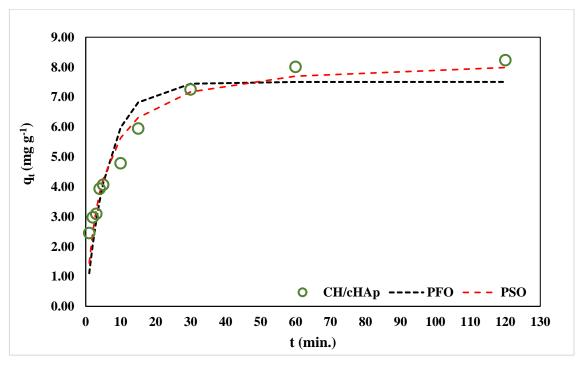
Figure 4-29: The fitting of the non-linear pseudo-first-order (PFO) and pseudo-second-order (PSO) kinetic models to the contact time experimental data for  $Cu^{2+}$  adsorption on the CH/cHAp composite
