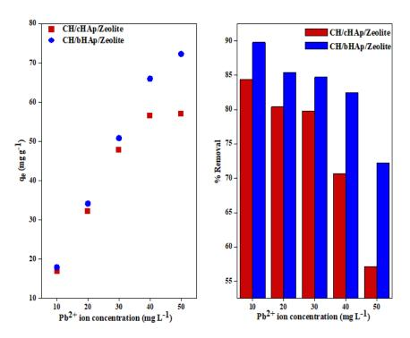
Figure 4-106: AAS data showing the effect of initial metal ions concentration on  $Pb^{2+}$  removal and adsorption on the CH/HAp/zeolite composites. The results are presented as the average of measurements of three replicates.  $SE = \pm 0.3$
