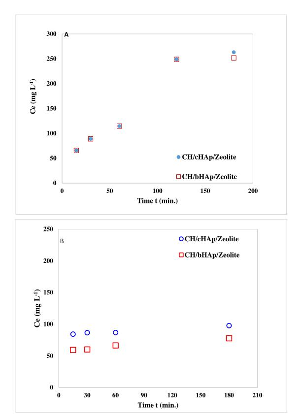
Figure 6-16: The concentration of phosphorus as analysed using ICP-MS in the industrial input stream solution exposed to the CH/HAp/zeolite composites at (A) 0.01 g, (B) 0.1 g of adsorbent doses.
