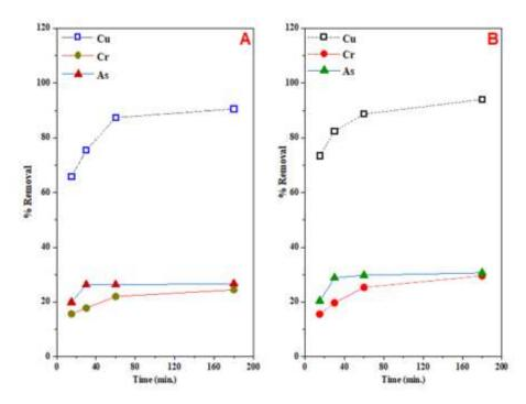
Figure 6-5: ICP-MS data for simultaneous removal of Cu<sup>2+</sup>, arsenate and chromate ions by the CH/HAp/SCGs composites using 0.01 g adsorbent doses of (A) CH/cHAp/SCGs composite and (B) CH/bHAp/SCGs composites.
