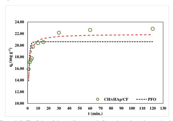
Figure 4-63: The fitting of the non-linear pseudo-first-order and pseudo-second-order kinetic models to the contact time data for chromate ion adsorption on the CH/cHAp/CF composites
