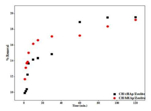
Figure 4-123: AAS data showing the effect of contact time on chromate ion removal by using the CH/HAp/zeolite composites. The results are presented as the average of measurements of three replicates.  $SE=\pm~0.02$
