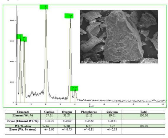
Figure 3-19: SEM micrograph and EDX analysis of the CH/cHAp/SCGs composite
