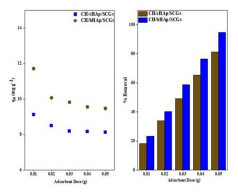
Figure 4-67: AAS data showing the effect of adsorbent dose on  $Cu^{2+}$  adsorption on the CH/HAp/SCGs composites. Results are presented as the average of 3 replicates. SE =  $\pm 0.4$
