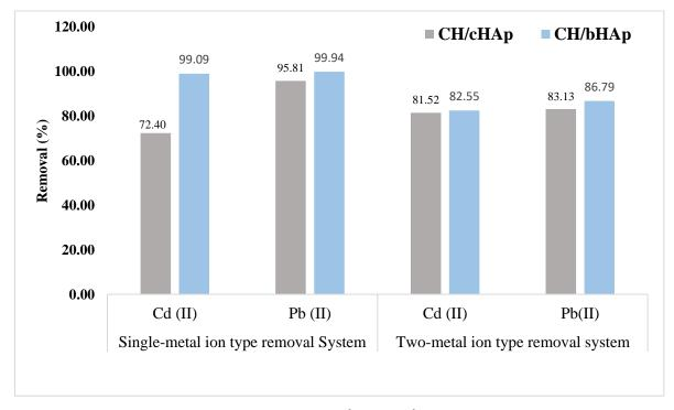
Figure 5-4: Comparison of removal data for Cd<sup>2+</sup> and Pb<sup>2+</sup> ions by a 0.05 g adsorbent dose of the CH/HAp composites from solutions containing either one or two metal ion types.
