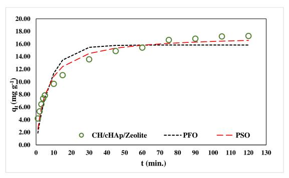
Figure 4-124: The fitting of the pseudo-first-order (PFO) and pseudo-second-order (PSO) kinetic models to the experimental data for  $Cd^{2+}$  adsorption on the CH/cHAp/zeolite composites
