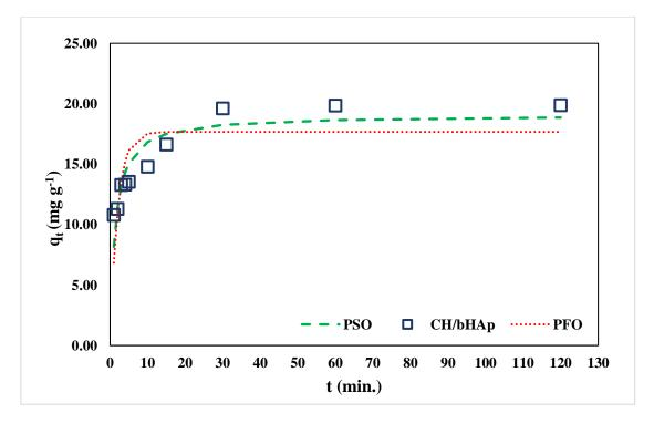
Figure 4-26: The fitting of the non-linear pseudo-first-order (PFO) and pseudo-second-order (PSO) kinetic models to the contact time experimental data for  $Cd^{2+}$  adsorption on the CH/bHAp composite
