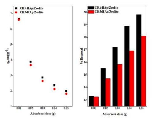
Figure 4-100: AAS data showing the effect of adsorbent dose on chromate ion removal and adsorption on the CH/HAp/zeolite composites. The results are presented as the average of measurements of three replicates.  $SE = \pm 0.1$
