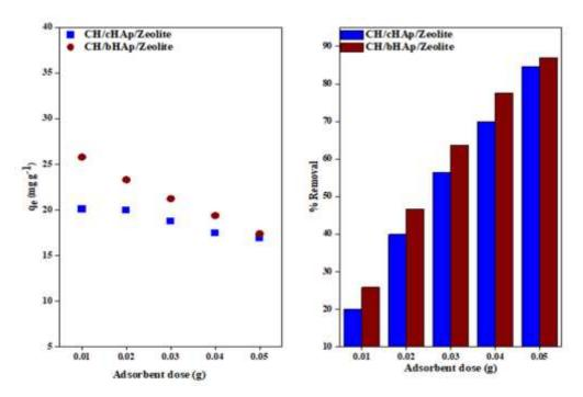
Figure 4-97: AAS data showing the effect of adsorbent dose on  $Cd^{2+}$  ion removal and adsorption of Cd2+ ion on the CH/HAp/zeolite composites: Results are presented as the average of measurements from 3 replicates.  $SE = \pm 0.7$
