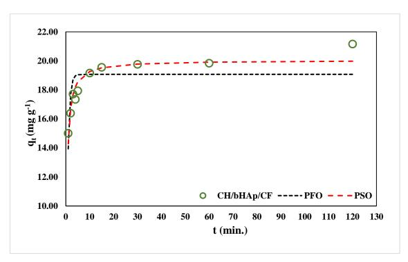
Figure 4-64: The fitting of the non-linear pseudo-first-order and pseudo-second-order kinetic models to the contact time data for chromate ion adsorption on the CH/bHAp/CF composites
