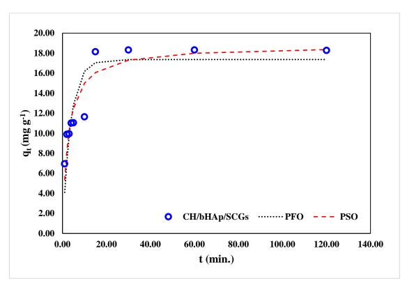
Figure 4-96: The fitting of the non-linear pseudo-first-order and pseudo-second-order kinetics model to the data for chromate ion adsorption on the CH/bHAp/SCGs composites
