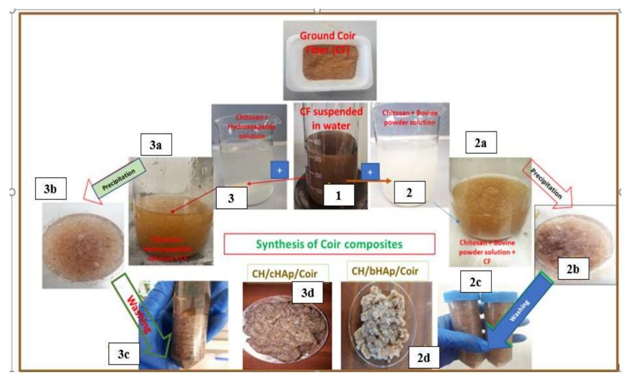
Figure 3-3: The synthesis of the CH/HAp/CF composites
