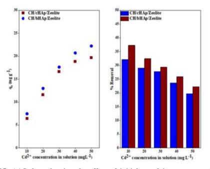
Figure 4-105: AAS data showing the effect of initial metal ion concentration on  $Cd^{2+}$  adsorption on CH/HAp/zeolite composites. Results are calculated as an average of 3 replicates. SE =  $\pm$  0.2.
