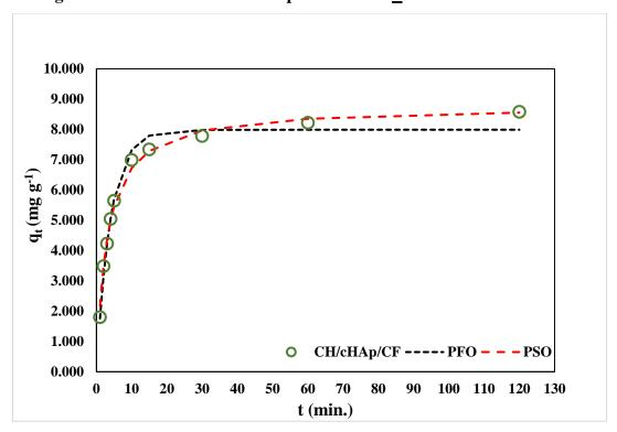
Figure 4-57: The fitting of the non-linear pseudo-first-order (PFO) and pseudo-second-order kinetic models to the contact time experimental data for  $Cd^{2+}$  adsorption on the CH/cHAp/CF composites
