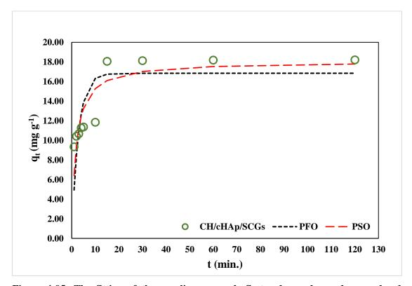
Figure 4-95: The fitting of the non-linear pseudo-first-order and pseudo-second-order kinetics model to the data for chromate ion adsorption on the CH/cHAp/SCGs composites
