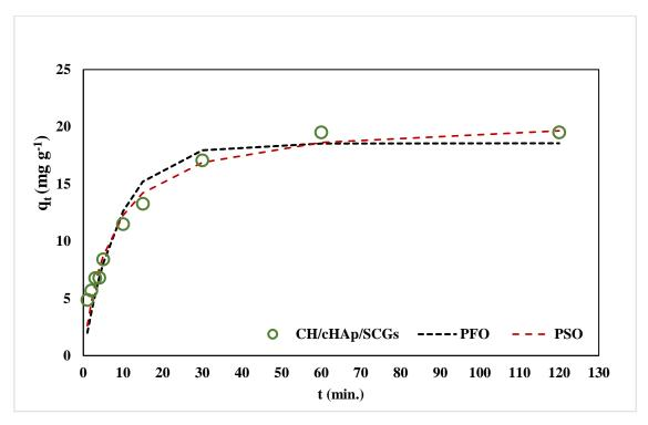
Figure 4-91: The fitting of the non-linear pseudo-first-order (PFO) and pseudo-second-order (PSO) kinetics models to the experimental data for  $Pb^{2+}$  adsorption on the CH/cHAp/SCGs composites
