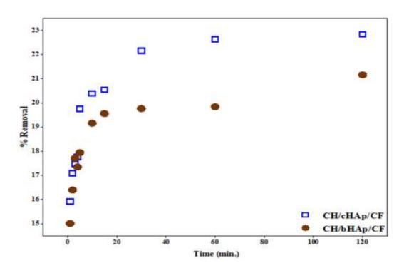
Figure 4-56: AAS data showing the effect of contact time on chromate ion removal and adsorption on the CH/HAp/CF composites. The results are presented as the average of measurements of three replicates.  $SE = \pm 0.1$
