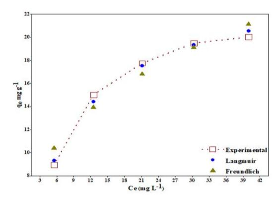
Figure 4-78: The fitting of the non-linear Langmuir and Freundlich adsorption isotherms to experimental data for Cd<sup>2+</sup> adsorption on the CH/bHAp/SCGs composites
