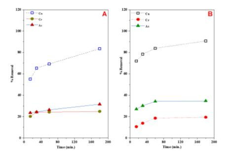
Figure 6-3: ICP-MS data showing the removal of Cu<sup>2+</sup>, chromate ion and arsenate ion from an industrial input stream sample by the CH/HAp/CF composites for a 0.01 g dose of (A) CH/cHAp/CF composites and (B) CH/bHAp/CF composites (Contact time data).
