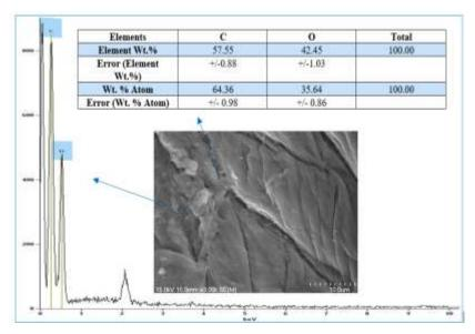
Figure 2-3: SEM micrograph and EDX analysis of the as-received TCI chitosan used in the present study
