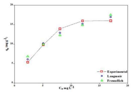
Figure 4-18: The fitting of the non-linear Langmuir and Freundlich isotherm models to the experimental data relating to  $Cu^{2+}$  adsorption on the CH/bHAp composites.
