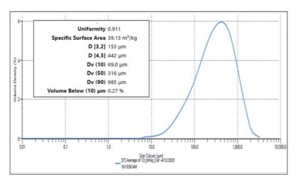
Figure 3 D: The average particle size of CH/bHAp/CF composites and estimated specific surface area (the results are presented as an average of three replicates)
