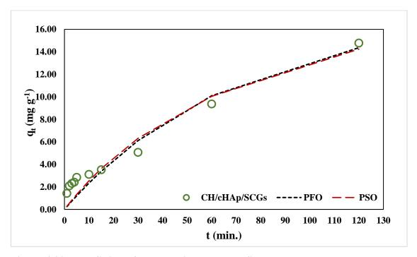
Figure 4-93: The fitting of the non-linear pseudo-first-order and pseudo-second-order kinetics models to experimental data for Cu<sup>2+</sup> adsorption on the CH/cHAp/SCGs composite
