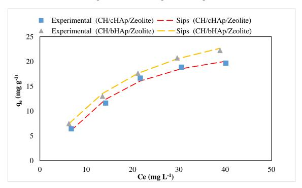
Figure 4-117: The fitting of the Sips isotherm model to the experimental data for  $Cd^{2+}$  ion adsorption on the CH/HAp/zeolite composites
