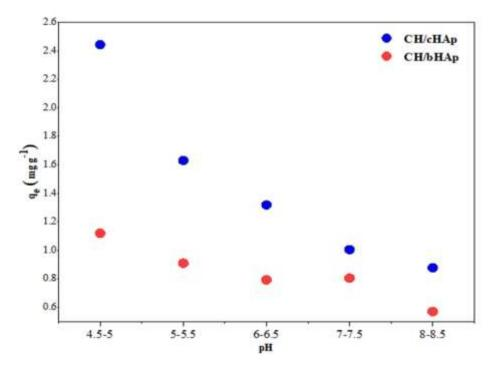
Figure 4-8: AAS data showing the effect of initial solution pH on chromate ion adsorption on the CH/HAp composites. Results are reported as the average of 3 replicates.  $SE=\pm0.01$
