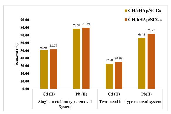
Figure 5-15: The comparison of single and two-metal ion type solution systems for  $Cd^{2+}$  and  $Pb^{2+}$  ions adsorption on 0.01 g of adsorbent dose of CH/HAp/SCGs composites
