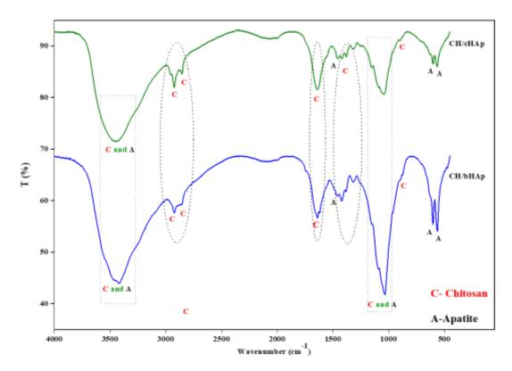
Figure 3-10: FTIR spectra of the CH/HAp composites
