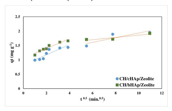
$Figure \ 5-26: The \ fitting \ of \ the \ intra-particle \ diffusion \ model \ (IPD) \ to \ the \ experimental \ data$  for chromate ion adsorption on the CH/HAp/zeolite composites
