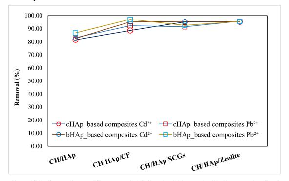
Figure 5-2: Comparison of the removal efficiencies of the synthesised composites for the removal of  $Pb^{2+}$  and  $Cd^{2+}$  in competitive adsorption system (in solutions containing two metal ion types) at 0.05 g of adsorbent dose
