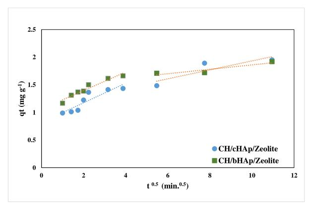
Figure 4-135: The fitting of intra-particle diffusion model (IPD) to the experimental data for chromate ion adsorption on the CH/HAp/zeolite composites
