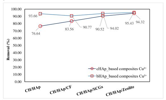
Figure 5-3: Comparison of the removal efficiencies of the synthesised composites for the removal of  $Cu^{2+}$  in industrial input stream sample when using 0.01 g of adsorbent dose
