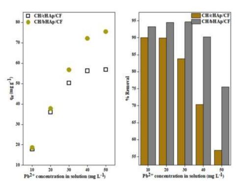
Figure 4-42: AAS data showing the effect of initial metal ion concentration on  $Pb^{2+}$  removal and adsorption on CH/HAp/CF composites. The results are presented as the average of measurements of three replicates.  $SE = \pm 0.1$
