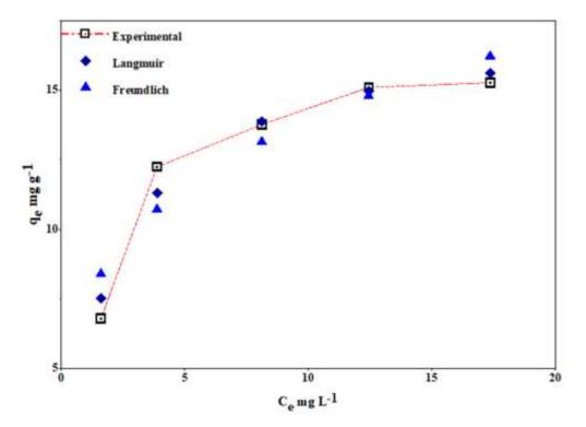
Figure 4-113: The fitting of the non-linear Langmuir and Freundlich isotherms to data for  $Cu^{2+}$  adsorption on the CH/cHAp/zeolite composite
