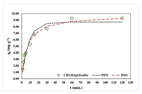
Figure 4-128: The fitting of the non-linear pseudo-first-order and pseudo-second-order kinetics models to experimental data for  $Cu^{2+}$  adsorption on the CH/cHAp/zeolite composite
