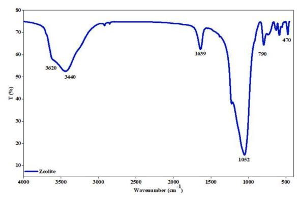
Figure 2-28: FTIR spectrum of zeolite (mordenite)
