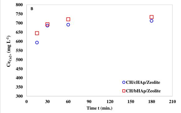
Figure 6-12: The concentration of  $Ca^{2+}$  ions analysed by ICP-MS in an industrial input stream during its exposure to (A) 0.01 g and (B) 0.1 g doses of the CH/HAp/zeolite composites
