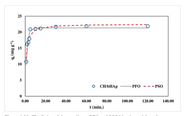
Figure 4-32: The fitting of the non-linear PFO and PSO kinetic models to the contact time experimental data for chromate ion adsorption on the CH/bHAp composites
