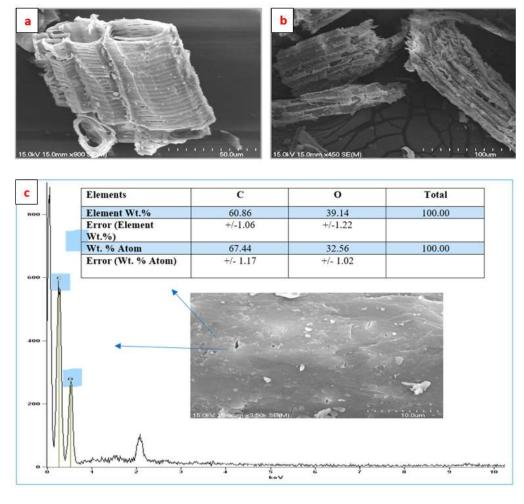
Figure 2-17: SEM micrograph of coir fibre with accompanying EDX analysis.
