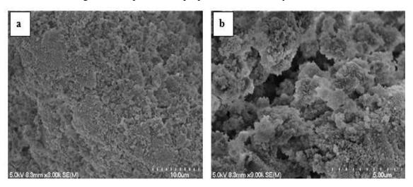
Figure 2-9: SEM micrographs of the commercial HAp (cHAp) used in this study
