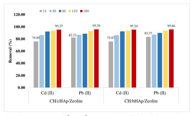
Figure 5-20: The competitive  $Cd^{2+}$  and  $Pb^{2+}$  removal (%) using 0.05 g of the CH/HAp/zeolite composites at contact times ranging from 15 minutes to 180 minutes.
