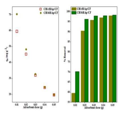
Figure 4-34: AAS data showing the effect of adsorbent dose on  $Pb^{2+}$  removal and adsorption on the CH/HAp/CF composites. The results are presented as the average of measurements of three replicates.  $SE = \pm 0.1$
