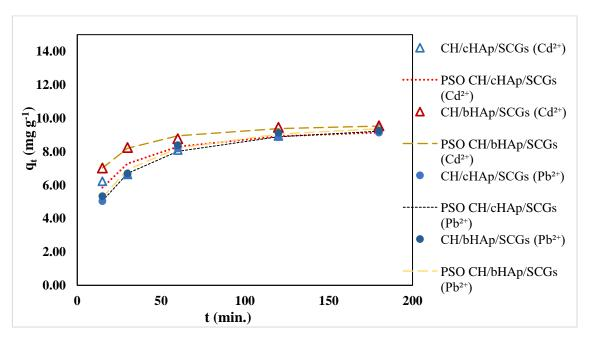
Figure 5-18: The fitting of the non-linear pseudo-second-order kinetic model to experimental (contact time) data relating to  $Cd^{2+}$  and  $Pb^{2+}$  competitive adsorption on the CH/HAp/SCGs composites on an adsorbent dose of 0.05 g
