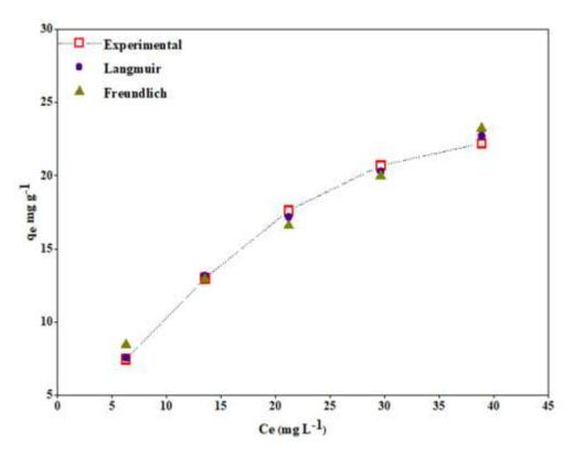
Figure 4-110: The fitting of the non-linear Langmuir and Freundlich adsorption isotherms to the experimental data for  $Cd^{2+}$  adsorption on the CH/bHAp/zeolite composite
