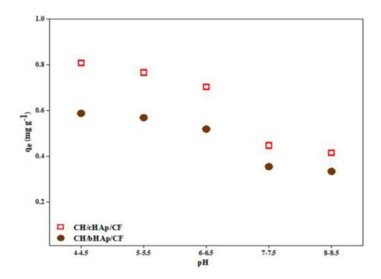
Figure 4-40: AAS data showing the effect of initial pH of the metal ion solution on chromate ion adsorption on the CH/HAp/CF composites. The results are presented as the average of measurements of three replicates.  $SE = \pm 0.1$
