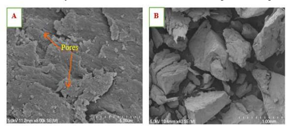
Figure 3-6: SEM micrographs of CH/cHAp composites at different magnifications
