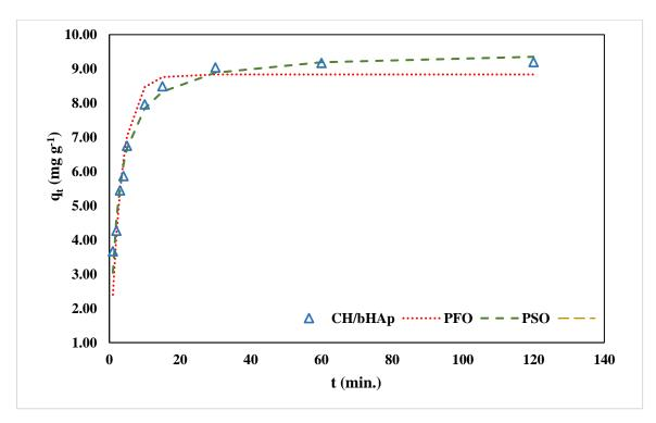
Figure 4-30: The fitting of the non-linear pseudo-first-order (PFO) and pseudo-second-order (PSO) kinetic models to the contact time experimental data for  $Cu^{2+}$  adsorption on the CH/bHAp composite
