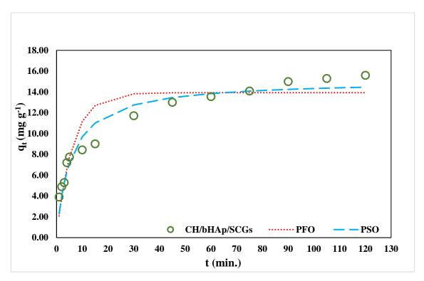
Figure 4-90: The fitting of the non-linear pseudo-first-order (PFO) and pseudo-second-order (PSO) kinetic models to the experimental data for  $Cd^{2+}$  adsorption on the CH/bHAp/SCGs composites
