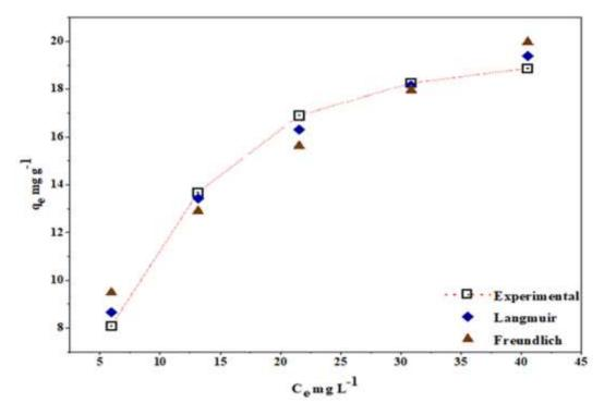
Figure 4-77: The fitting of the non-linear Langmuir and Freundlich adsorption isotherms to experimental data for Cd<sup>2+</sup> adsorption on the CH/cHAp/SCGs composite
