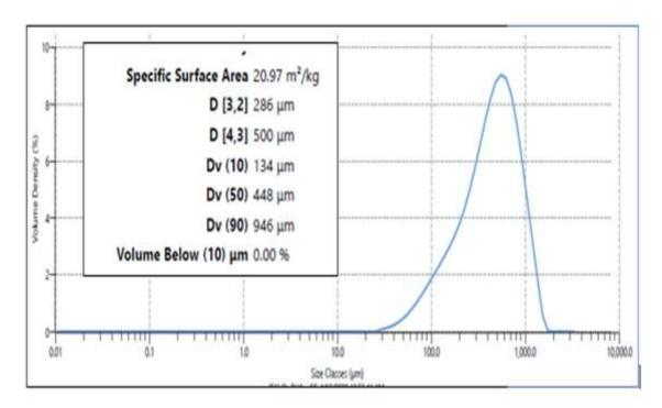
Figure 3 G: The average particle size of CH/cHAp/SCGs composites and estimated specific surface area (the results are presented as an average of three replicates)
