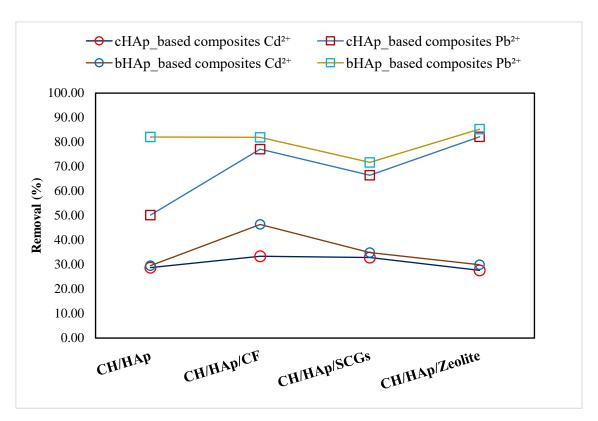
Figure 5-1: Comparison of the removal efficiencies of the synthesised composites for the competitive removal of  $Pb^{2+}$  and  $Cd^{2+}$  by adsorption (in solutions containing two metal ion types) when using 0.01 g of adsorbent
