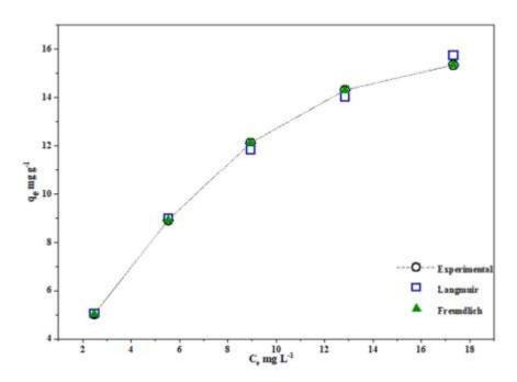
Figure 4-13: Graph showing the fitting of the non-linear Langmuir and Freundlich adsorption models to the experimental data for Cd<sup>2+</sup> adsorption on the CH/cHAp composite
