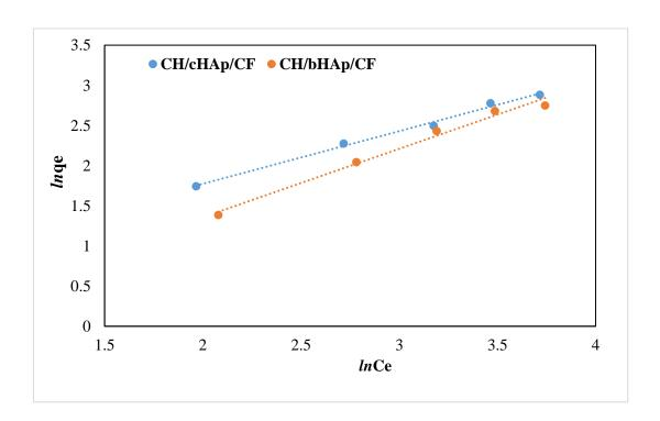
Figure 4-52: Fitting of the linearized Freundlich isotherm model to the experimental data for chromate ion adsorption on the CH/HAp/CF composites.
