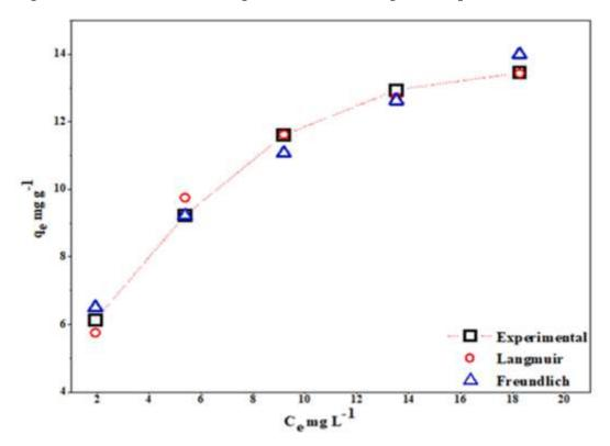
Figure 4-49: The fitting of the non-linear Langmuir and Freundlich isotherms to data for  $Cu^{2+}$  adsorption on the CH/cHAp/CF composite
