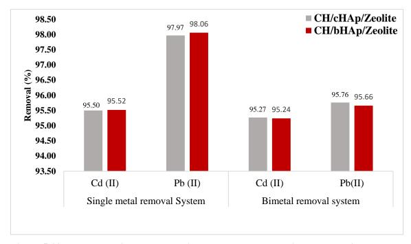
Figure 5-22: The comparison one-metal ion type and two-metal ion type solution systems for  $Cd^{2+}$  and  $Pb^{2+}$  adsorption on 0.05 g of adsorbent dose of CH/HAp/Zeolite composites
