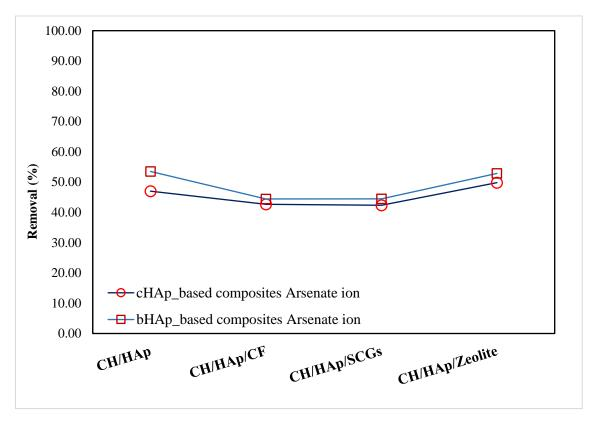
Figure 5-8: Comparison of the removal efficiencies of the synthesised composites for the removal of arsenate ions in industrial input stream sample using 0.1 g of adsorbent.
