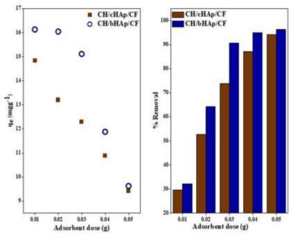
Figure 4-35: AAS data showing the effect of adsorbent dose on  $Cu^{2+}$  adsorption on the CH/HAp/CF composites. Results are presented as the average of 3 replicates. SE =  $\pm 0.1$
