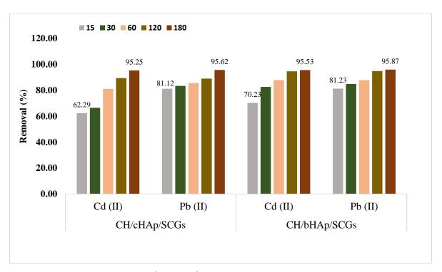
Figure 5-14: The competitive Cd<sup>2+</sup> and Pb<sup>2+</sup> removal (%) using 0.05 g of the CH/HAp/SCGs composites at contact times ranging from 15 minutes to 180 minutes.
