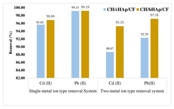
Figure 5-10: The comparison of single metal ion type and two-metal ion type systems for Cd<sup>2+</sup> and Pb<sup>2+</sup> adsorption on 0.05 g of adsorbent dose of CH/HAp/CF composites.
