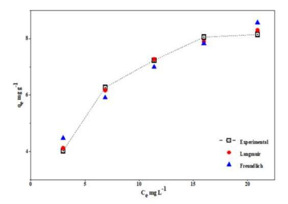
Figure 4-81: The fitting of the non-linear Langmuir and Freundlich isotherms to data for  $Cu^{2+}$  adsorption on the CH/cHAp/SCGs composite
