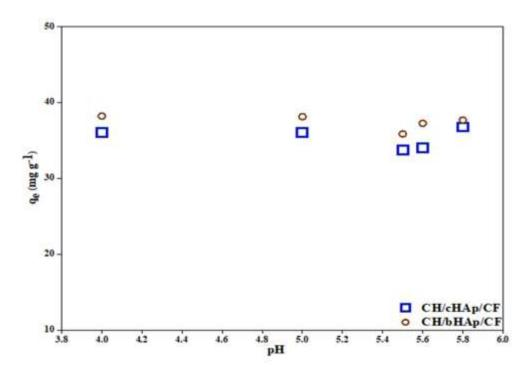
Figure4-38: AAS data showing the effect of solution pH on  $Pb^{2+}$  removal and adsorption on CH/HAp/Composites. The results are presented as the average of measurements of three replicates.  $SE=\pm0.1$
