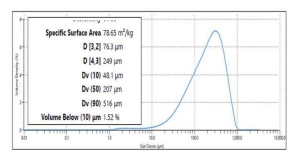
Figure 3 H: The average particle size of CH/bHAp/SCGs composites and estimated specific surface area (the results are presented as an average of three replicates
