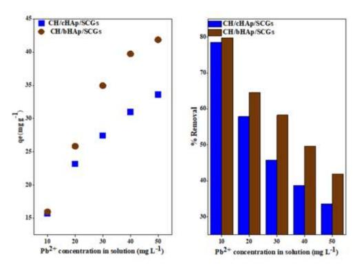
Figure 4-74: AAS data showing the effect of initial metal ion concentration on  $Pb^{2+}$  removal and adsorption on CH/HAp/SCGs composites. The results are presented as the average of measurements of three replicates.  $SE = \pm 0.3$
