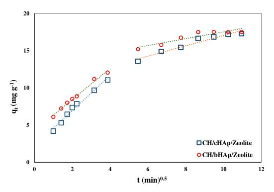
Figure 4-132: The fitting of the intra-particle diffusion model (IPD) to the experimental data for  $Cd^{2+}$  adsorption on the CH/HAp/zeolite composites
