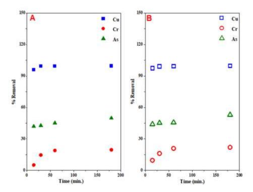
Figure 6-8: ICP-MS data showing simultaneous removal of Cu<sup>2+</sup>, arsenate ion and chromate ion by the CH/HAp/Zeolite composites using 0.1 g adsorbent doses of (A) CH/cHAp/zeolite composite and (B) CH/bHAp/zeolite composites
