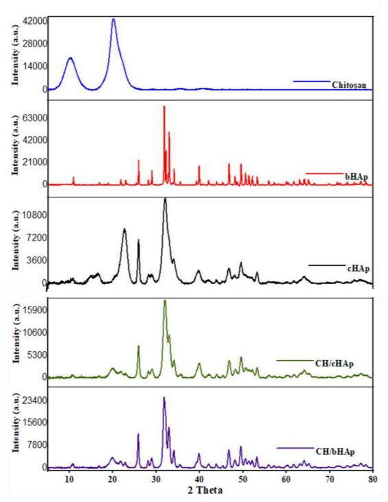
Figure 3-11: Diffractograms of CH/HAp composites and the candidate materials used to synthesise the composite
