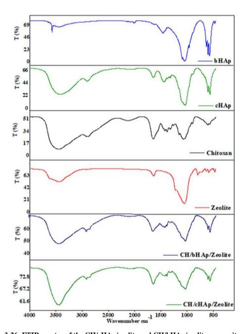
Figure 3-26: FTIR spectra of the CH/cHAp/zeolite and CH/bHAp/zeolite composites
