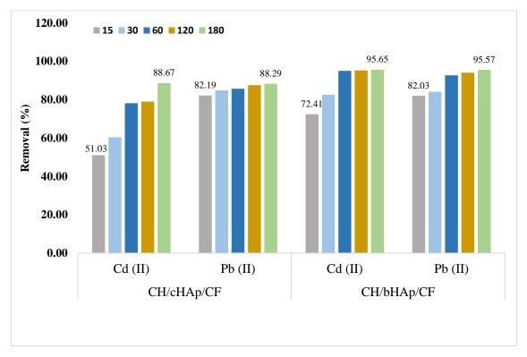
Figure 5-8: The competitive Cd<sup>2+</sup> and Pb<sup>2+</sup> removal (%) using 0.05 g of the CH/HAp/CF composites at contact times ranging from 15 minutes to 180 minutes.
