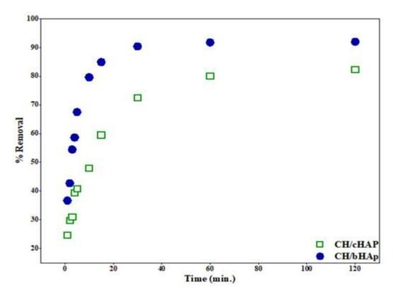
Figure 4-23: AAS data showing the effect of contact time on  $Cu^{2+}$  adsorption by the CH/HAp composites. Results are reported as the average of 3 replicates.  $SE = \pm 0.1$
