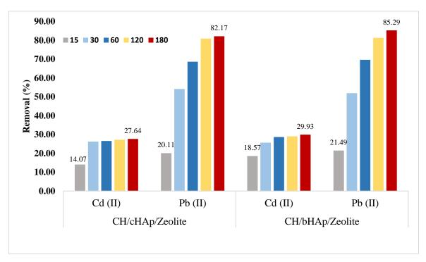
Figure 5-19: Graph showing the competitive removal (%) of Cd<sup>2+</sup> and Pb<sup>2+</sup> ions by 0.01 g doses of the CH/HAp/zeolite composites at contact times ranging from 15 minutes to 180 minutes.
