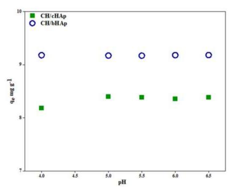
Figure 4-7: AAS data showing the effect of initial solution pH on  $Cu^{2+}$  adsorption on the CH/HAp composites. Results are reported as the average of 3 replicates. SE= $\pm 0.01$
