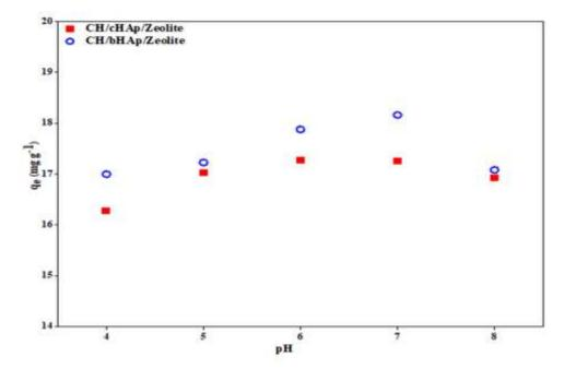
Figure 4-101: AAS data showing the effect of solution pH on  $Cd^{2+}$  adsorption on the CH/HAp/zeolite composites. The results are presented as the average of measurements of three replicates.  $SE = \pm 0.3$
