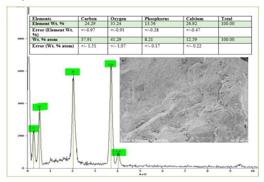
Figure 3-14: SEM micrograph and EDX analysis of CH/cHAp/CF composites
