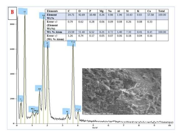
Figure 3-25: SEM micrograph and EDX analysis of the CH/bHAp/Zeolite composite
