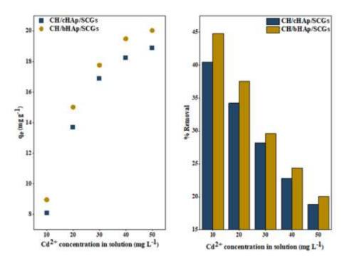
Figure 4-73: AAS data showing the effect of initial metal ion concentration on  $Cd^{2+}$  adsorption on the CH/HAp/SCGs composites. Results are calculated as an average of 3 replicates. SE =  $\pm$  0.1.
