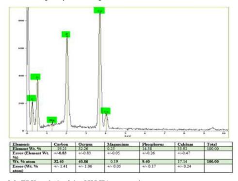
Figure 3-9: EDX analysis of the CH/bHAp composite
