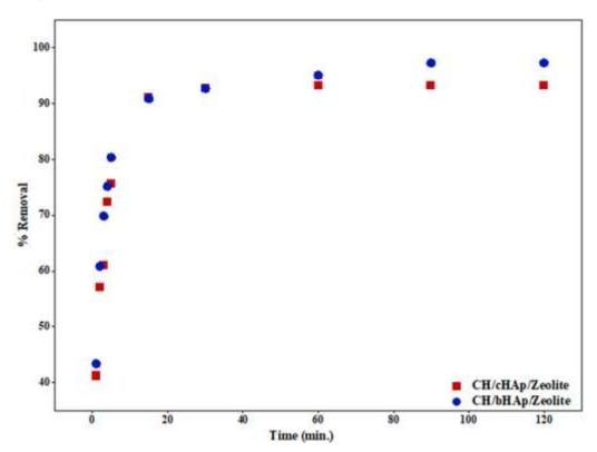
Figure 4-121: AAS data showing the effect of contact time on  $Pb^{2+}$  adsorption on the CH/HAp/zeolite composites. Results are reported as the average of 3 replicates.  $SE = \pm 0.1$ .
