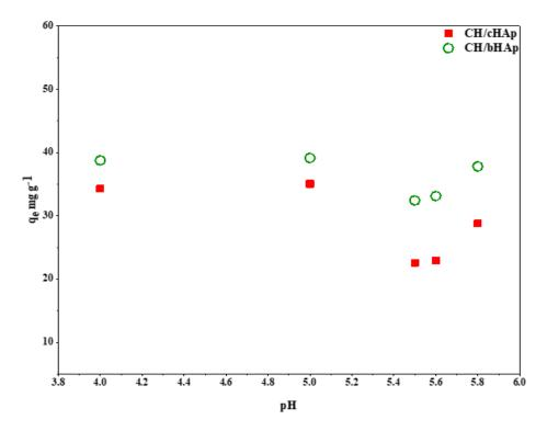
Figure 4-6: AAS data showing the effect of initial solution pH on  $Pb^{2+}$  adsorption on the CH/HAp composites. Results are reported as the average of 3 replicates.  $SE=\pm0.1$
