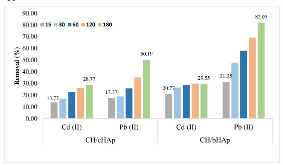
Figure 5-1: The competitive Cd<sup>2+</sup> and Pb<sup>2+</sup> ion removal (%) by 0.01 g doses of the CH/HAp composites at contact times ranging from 15 minutes to 180 minutes.
