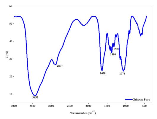
Figure 2-5: FTIR spectrum of TCI chitosan used in this study
