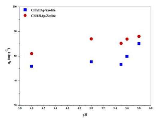
Figure 4-102: AAS data showing the effect of solution pH on  $Pb^{2+}$  adsorption on the CH/HAp/zeolite composites. The results are presented as the average of measurements of three replicates.  $SE = \pm 0.2$
