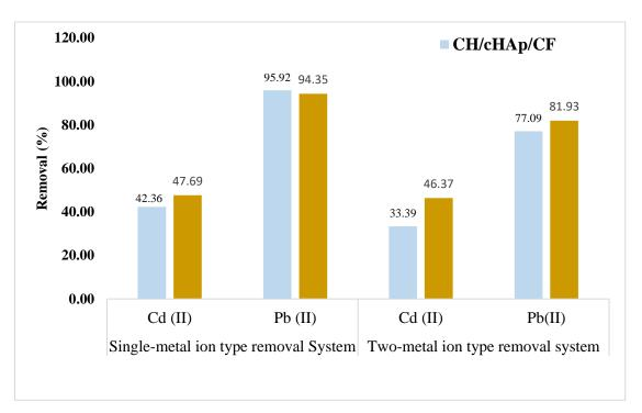
Figure 5-9: The comparison of single metal ion type and two-metal ion type systems for  $Cd^{2+}$  and  $Pb^{2+}$  adsorption on 0.01 g of adsorbent dose of CH/HAp/CF composites
