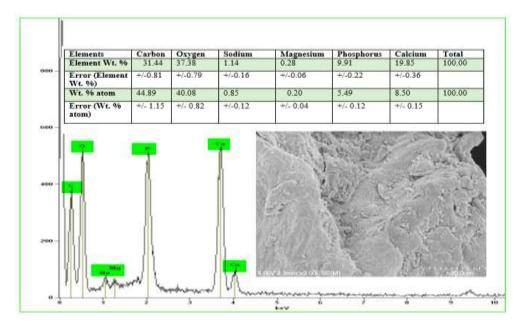
Figure 3-15: SEM micrograph and EDX analysis of the CH/bHAp/CF composite
