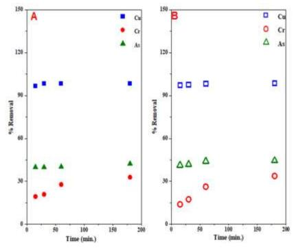
Figure 6-6: ICP-MS data showing simultaneous removal of Cu<sup>2+</sup>, arsenate ion and chromate ion by the CH/HAp/SCGs composites using 0.1 g adsorbent doses of (A) CH/cHAp/SCGs composite and (B) CH/bHAp/SCGs composites.
