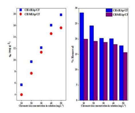
Figure 4-44: AAS data showing the effect of the initial metal ion concentration on chromate ion removal and adsorption on the CH/HAp/CF composites. The results are presented as the average of measurements of three replicates.  $SE = \pm 0.1$
