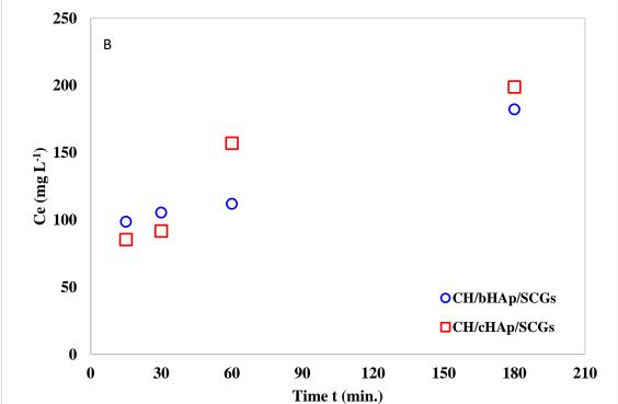
Figure 6-15: The concentration of phosphorus as analysed using ICP-MS in the industrial input stream solution exposed to the CH/HAp/SCGs composites at  $(A)\ 0.01\ g$ ,  $(B)\ 0.1\ g$  of adsorbent doses
