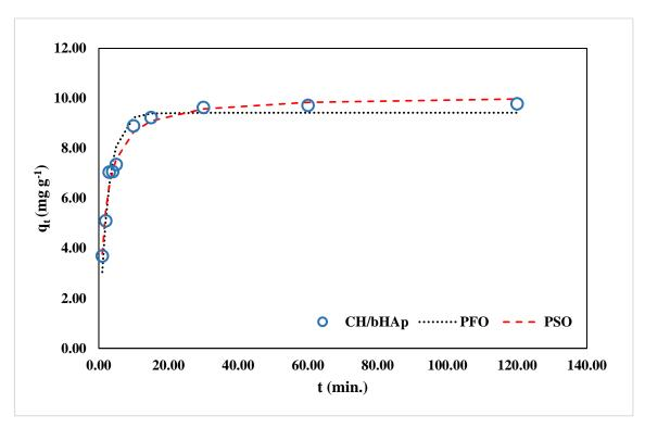
Figure 4-28: The fitting of the non-linear pseudo-first-order (PFO) and pseudo-second-order (PSO) kinetic models to the contact time experimental data for  $Pb^{2+}$  adsorption on the CH/bHAp composite
