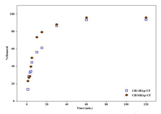
Figure 4-55: AAS data showing the effect of contact time on  $Cu^{2+}$  removal by the CH/HAp/CF composites. The results are presented as the average of measurements of three replicates.  $SE=\pm0.1$
