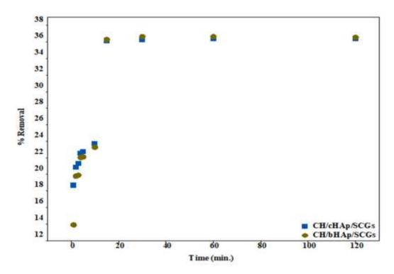
Figure 4-88: AAS data showing the effect of contact time on chromate ion removal and adsorption on the CH/HAp/SCGs composites. The results are presented as the average of measurements of three replicates.  $SE = \pm 0.2$
