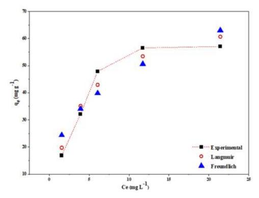
Figure 4-111: The fitting of the non-linear Langmuir and Freundlich adsorption isotherms to experimental data for Pb<sup>2+</sup> adsorption on the CH/cHAp/zeolite composite
