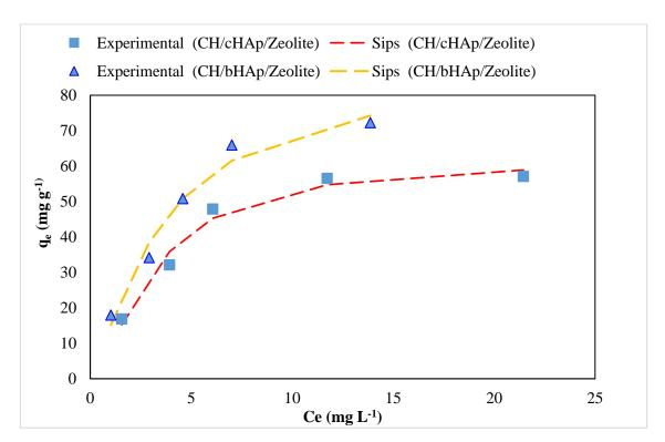
Figure 4-118: The fitting of the Sips isotherm model to the experimental data for  $Pb^{2+}$  ion adsorption on the CH/HAp/zeolite composites
