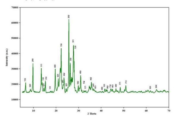
Figure 2-29: X-ray Diffractogram of zeolite (mordenite) used in this study
