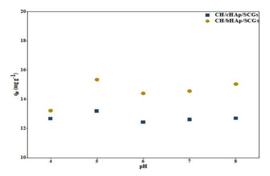
Figure 4-69: AAS data showing the effect of the solution pH on  $Cd^{2+}$  removal and adsorption on the CH/HAp/SCGs composites. The results are presented as the average of measurements of three replicates.  $SE = \pm 0.1$
