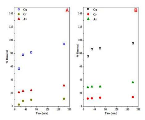
Figure 6-7: ICP-MS data for simultaneous removal of Cu<sup>2+</sup>, arsenate and chromate ions by the CH/HAp/Zeolite composites using 0.01 g adsorbent doses of (A) CH/cHAp/Zeolite composite and (B) CH/bHAp/Zeolite composites.
