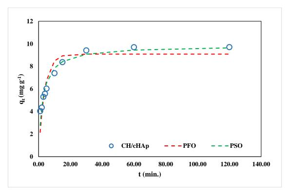
Figure 4-27: The fitting of the non-linear pseudo-first-order (PFO) and pseudo-second-order (PSO) kinetic models of the contact time experimental data for  $Pb^{2+}$  adsorption on the CH/cHAp composite
