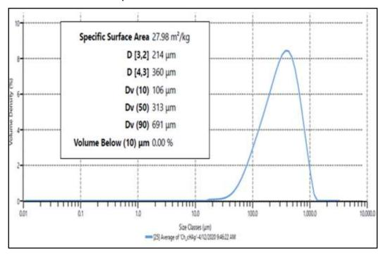
Figure 3A: The average particle size of the CH/cHAp composites and estimated specific surface area (the results are presented as an average of three replicates)
