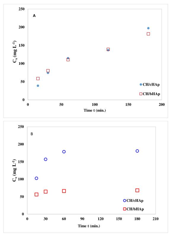
Figure 6-13: The concentration of phosphorus as analysed using ICP-MS in the industrial input stream solution exposed to the CH/HAp composites at doses of (A) 0.01 g (B) 0.1 g
