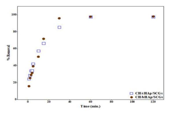
Figure 4-86: AAS data showing the effect of contact time on  $Pb^{2+}$  adsorption on the CH/HAp/SCGs composites. Results are reported as the average of 3 replicates.  $SE = \pm 0.1$ .
