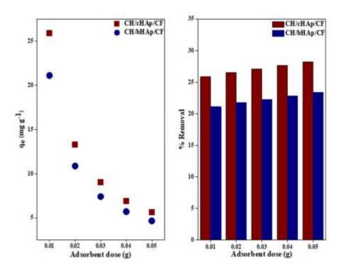
Figure 4-36: AAS data showing the effect of adsorbent dose on chromate ion removal and adsorption on the CH/HAp/CF composites. The results are presented as the average of measurements of three replicates.  $SE = \pm 0.1$
