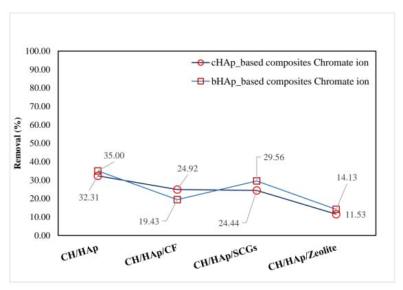
Figure 5-5: Comparison of the removal efficiencies of the synthesised composites for the removal of chromate ions from an industrial input stream sample using 0.01 g of adsorbent
