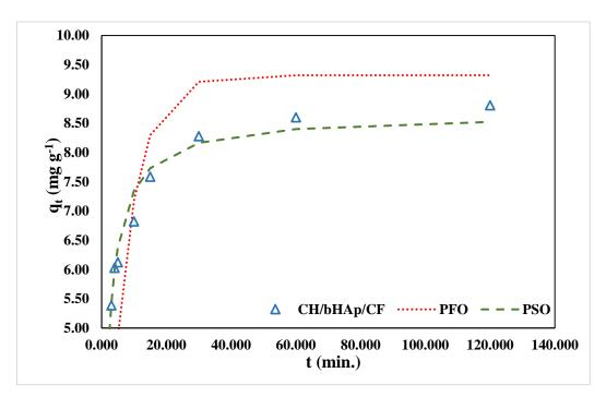
Figure 4-62: The fitting of the non-linear pseudo-first-order and pseudo-second-order kinetics models to contact time experimental data for Cu<sup>2+</sup> adsorption on the CH/bHAp/CF composite
