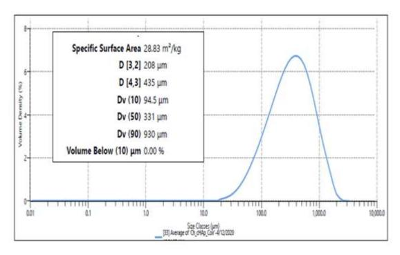
Figure 3 C: The average particle size of CH/cHAp/CF composites and estimated specific surface area (the results are presented as an average of three replicates)
