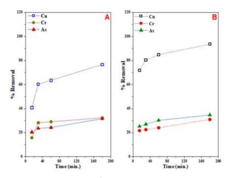
Figure 6-1: Simultaneous removal of  $Cu^{2+}$ , arsenate ion and chromate ion by the CH/HAp composites using 0.01 g adsorbent doses of (A) CH/cHAp composite and (B) CH/bHAp composites
