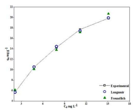
Figure 4-14: Graph showing the fitting of the non-linear Langmuir and Freundlich adsorption models to the experimental data for  $Cd^{2+}$  adsorption on the CH/bHAp composite
