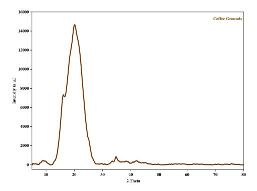
Figure 2-24: Powder X-ray diffractogram of spent coffee grounds used in the current study
