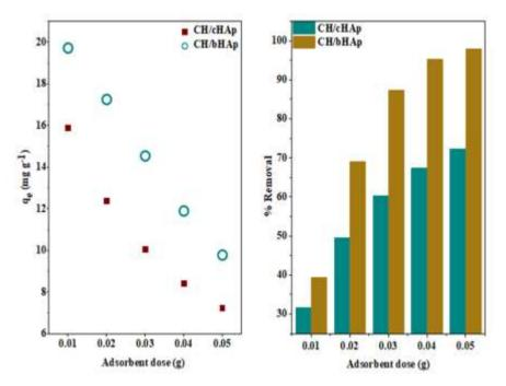
Figure 4-1: AAS results showing the effect of adsorbent dose on  $Cd^{2+}$  ion removal and adsorption of  $Cd^{2+}$  ion on the CH/HAp composites: Results are presented as the average of measurements from 3 replicates.  $SE = \pm 0.1$
