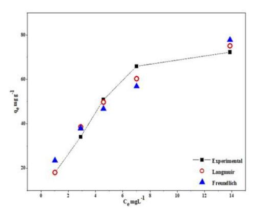
Figure 4-112: The fitting of the non-linear Langmuir and Freundlich adsorption isotherms to experimental data for  $Pb^{2+}$  adsorption on the CH/bHAp/zeolite composite
