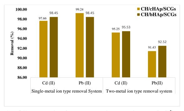
Figure 5-16: The comparison of one and two-metal ion type solution systems for  $Cd^{2+}$  and  $Pb^{2+}$  adsorption on 0.05 g of adsorbent dose of CH/HAp/SCGs composites
