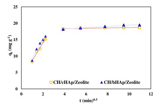
Figure 4-133: The fitting of the intra-particle diffusion model (IPD) to the experimental data for  $Pb^{2+}$  adsorption kinetics data on the CH/HAp/zeolite composites
