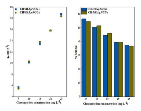
Figure 4-76: AAS data showing the effect of initial metal ion concentration on chromate ion removal and adsorption on the CH/HAp/SCGs composites. The results are presented as the average of measurements of three replicates.  $SE = \pm 0.3$
