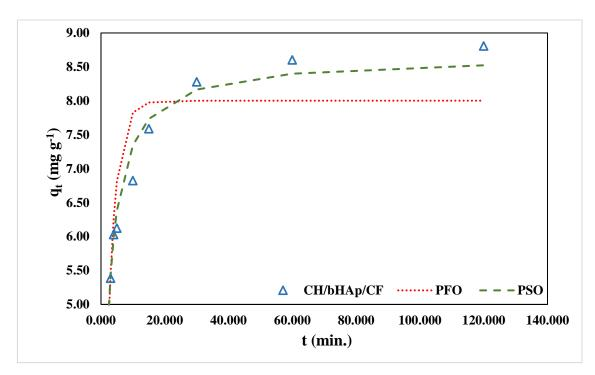
Figure 4-58: The fitting of the non-linear pseudo-first-order (PFO) and pseudo-second-order kinetic models to the contact time experimental data for Cd<sup>2+</sup> adsorption on the CH/bHAp/CF composites
