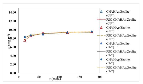
Figure 5-24: relating to  $Cd^{2+}$  and  $Pb^{2+}$  competitive adsorption on the CH/HAp/zeolite composites for an adsorbent dose of 0.05 g
