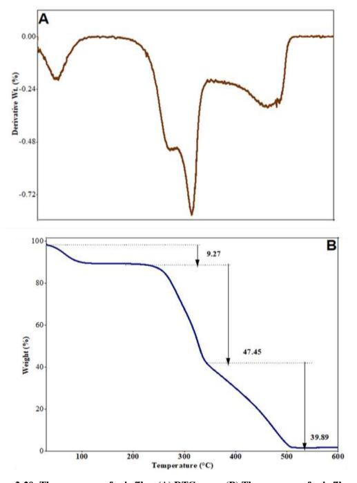
Figure 2-20: Thermograms of coir fibre (A) DTG curve (B) Thermogram of coir fibre
