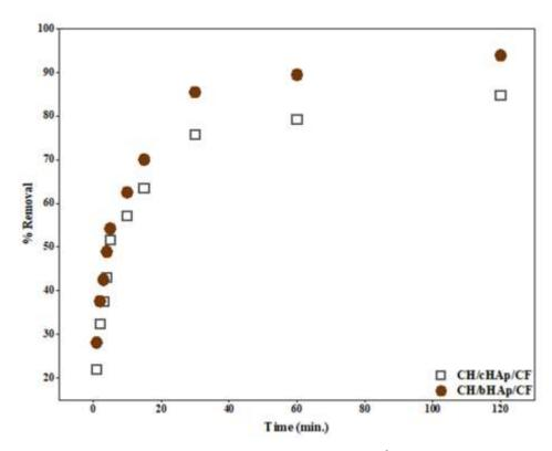
Figure 4-54: AAS data showing the effect of contact time on  $Pb^{2+}$  adsorption on CH/HAp/CF composites. Results are reported as the average of 3 replicates.  $SE = \pm 0.1$ .
