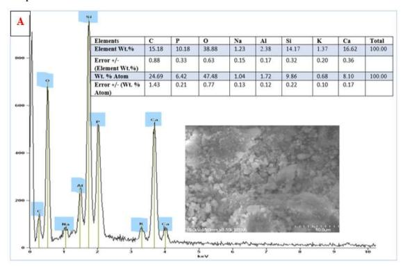
Figure 3-24: SEM micrograph and EDX analysis of the CH/cHAp/Zeolite composite
