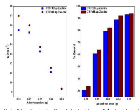
Figure 4-99: AAS data showing the effect of adsorbent dose on  $Cu^{2+}$  adsorption and removal of  $Cu^{2+}$  by the CH/HAp/zeolite composites. Results are presented as the average of 3 replicates.  $SE = \pm 0.2$
