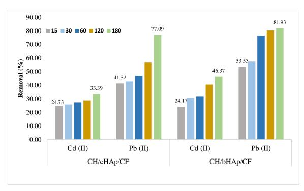
Figure 5-7: Graph showing the competitive removal (%) of Cd<sup>2+</sup> and Pb<sup>2+</sup> ions by 0.01 g doses of the CH/HAp/CF composites at contact times ranging from 15 minutes to 180 minutes.
