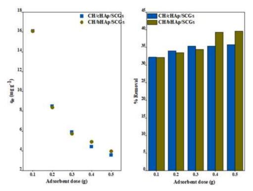
Figure 4-68: AAS data showing the effect of adsorbent dose on chromate ion removal and adsorption on the CH/HAp/SCGs composites. The results are presented as the average of measurements of three replicates.  $SE = \pm 0.7$
