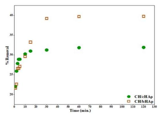
Figure 4-21: The effect of contact time on  $Cd^{2+}$  removal by the CH/HAp composites (from AAS data). Results are reported as the average of 3 replicates.  $SE=\pm0.1$
