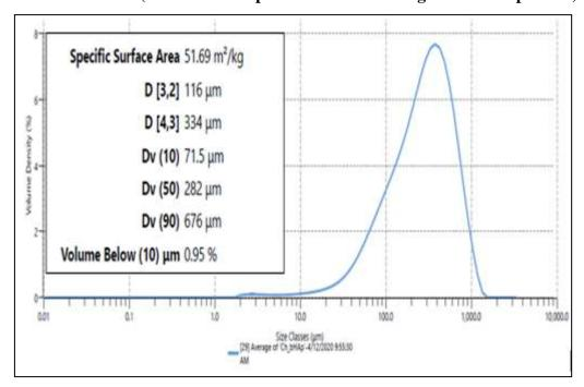
Figure 3B: The average particle size of CH/bHAp composites and estimated specific surface area (the results are presented as an average of three replicates)
