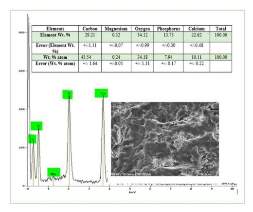
Figure 3-20: SEM micrograph and EDX analysis of the CH/bHAp/SCGs composite
