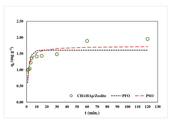
Figure 4-130: The fitting of the non-linear pseudo-first-order and pseudo-second-order kinetics model to the data for chromate ion adsorption on the CH/cHAp/zeolite composites
