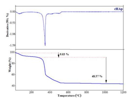
Figure 2-15: Thermogram of cHAp and corresponding DTG curve
