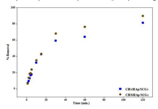
Figure 4-87: AAS data showing the effect of contact time on  $Cu^{2+}$  removal by the CH/HAp/SCGs composites. The results are presented as the average of measurements of three replicates.  $SE=\pm0.02$
