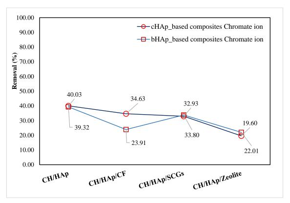
Figure 5-6: Comparison of the removal efficiencies of the synthesised composites for the removal of chromate ions in industrial input stream sample using 0.1 g of adsorbent dose
