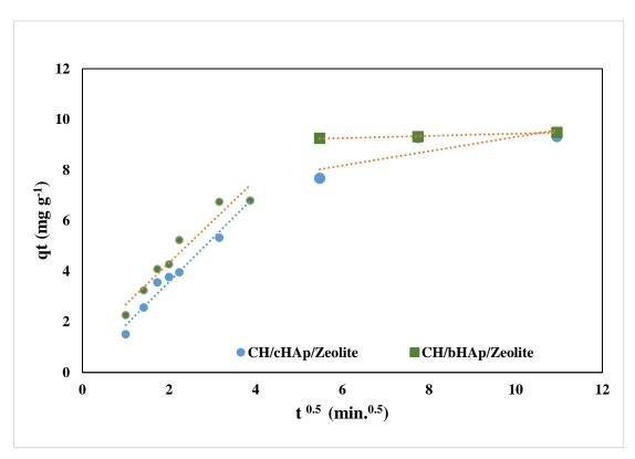
Figure 5-25 : The fitting of the intra-particle diffusion model (IPD) to the experimental data for  $Cu^{2+}$  adsorption on the CH/HAp/zeolite composites
