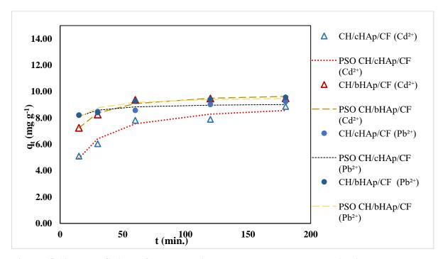
Figure 5-12: The fitting of the non-linear pseudo-second-order kinetic model to experimental (contact time) data relating to  $Cd^{2+}$  and  $Pb^{2+}$  competitive adsorption on the CH/HAp/CF composites on an adsorbent dose of 0.05 g
