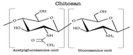
Figure 2-4: The basic structural unit of chitosan biopolymer <sup>399</sup>
