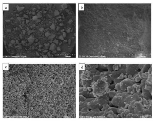
Figure 2-11: SEM micrographs of bHAp (a) x30 (b) x500 (c) x5.00k (d) x15.0k
