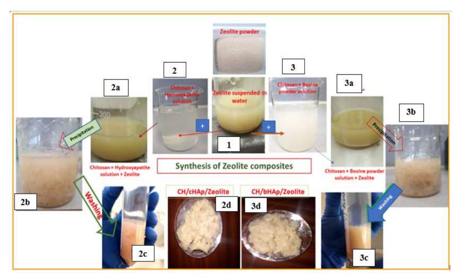
Figure 3-5: The synthesis of the CH/HAp//Zeolite composites
