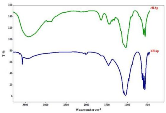
Figure 2-13: FTIR spectra of cHAp and bHAp
