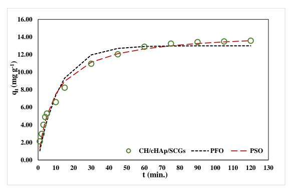
Figure 4-89: The fitting of the non-linear pseudo-first-order (PFO) and pseudo-second-order (PSO) kinetic models to the experimental data for  $Cd^{2+}$  adsorption on the CH/cHAp/SCGs composites
