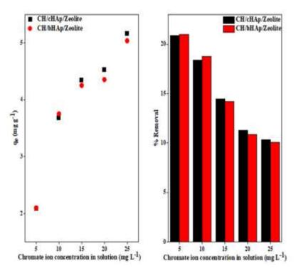
Figure 4-108: AAS data showing the effect of initial metal ion concentration on chromate ion removal and adsorption on the CH/HAp/zeolite composites. The results are presented as the average of measurements of three replicates. SE =  $\pm$  0.
